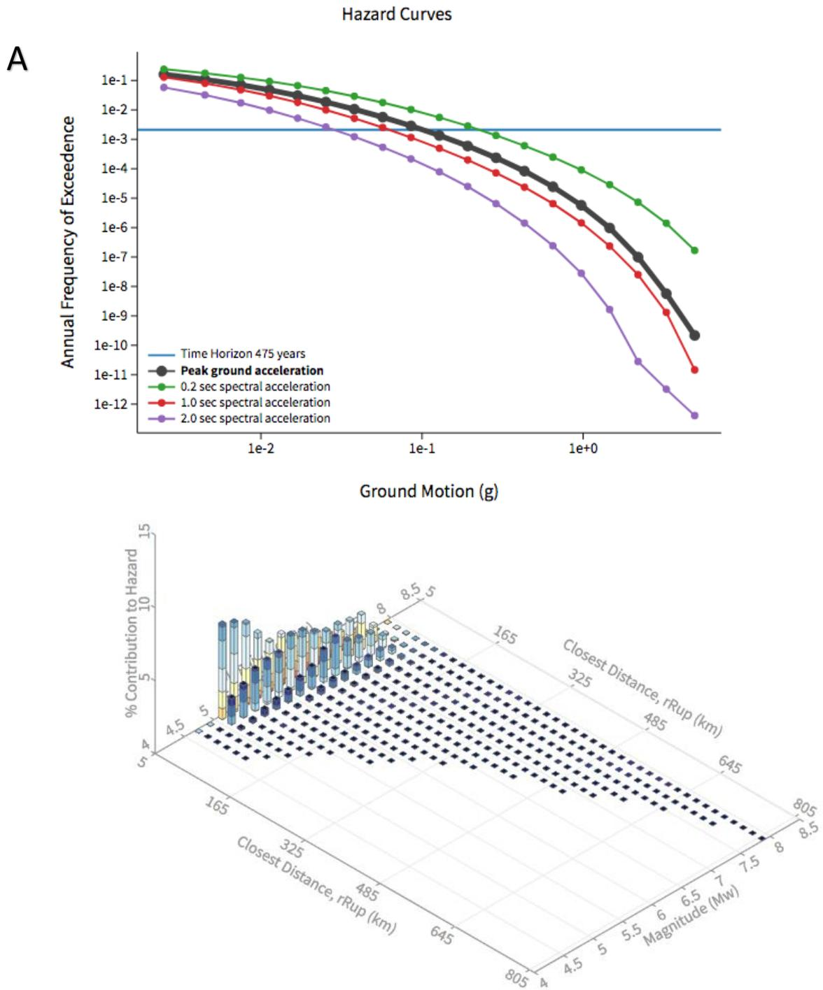
**Figure II.1.23.** Probabilistic seismic hazard at the FORGE site from the 2014 National Seismic Hazard map and tools found at (<https://earthquake.usgs.gov/hazards/interactive/>; last accessed 1/29/2017). (a) Hazard curves for the FORGE site. (b) Deaggregation for the 10% in 50 yrs PGA hazard (475 yr return period). Results show that the largest contribution to this hazard is from M 5.2 earthquakes at <20 km distance.
