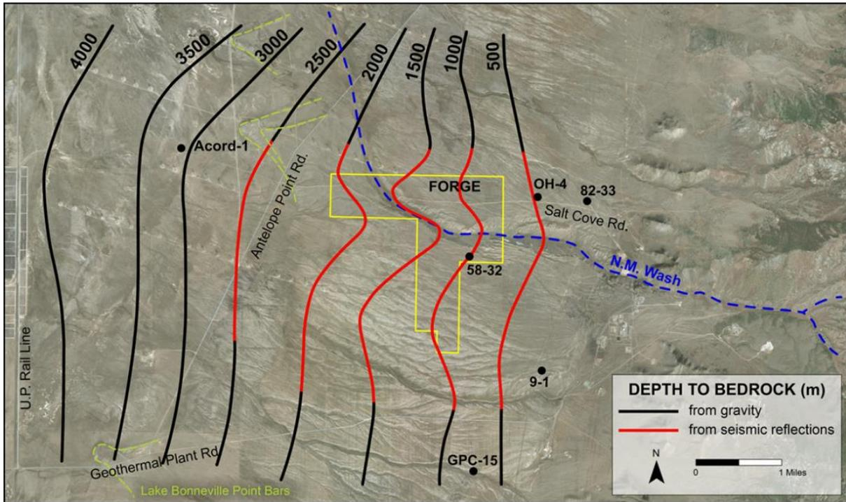
**Figure II.1.7.** Structure contour map of the basement contact beneath the FORGE site from seismic reflection surveys and gravity modeling. Contours represent depth below a horizontal datum of 1800 m asl. N.M. wash=Negro Mag wash.
