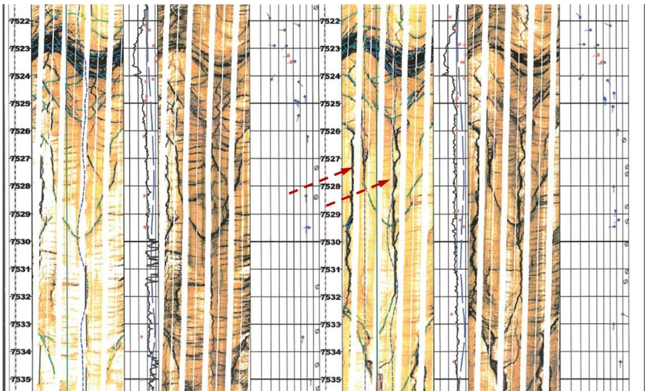
**Figure II.1.11.** 58-32 injection testing results. A) Time series of surface pressure measured at the wellhead; B) Comparison of FMI logs before (left two FMI images) and after (right two FMI images) injection, showing enhancement and growth of vertical fractures and the maximum horizontal stress in the north northeast direction. Symbols: tadpole=natural fracture showing orientation (dip azimuth and dip angle); circle with diagonal line=induced fracture and the angle represents strike azimuth.
