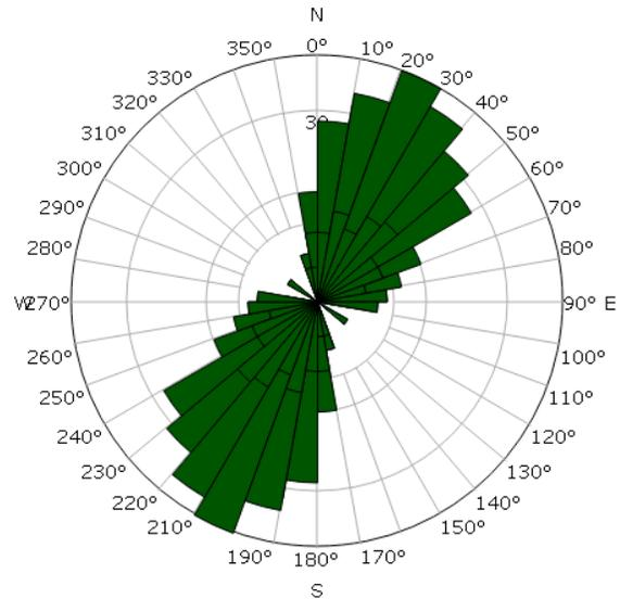
**Figure II.1.10.** Well 58-32 fracture data: A) Rose diagram of fracture azimuths and stereo net of poles to ~2000 natural fractures (upper hemisphere projection); B) Rose plot of azimuths of 356 drilling induced subvertical tensile fractures.
