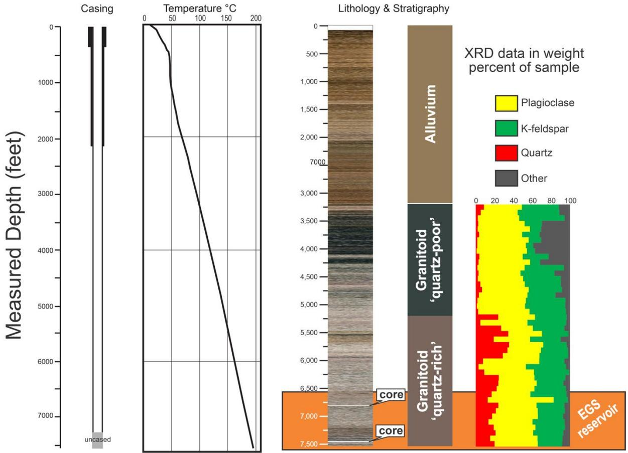
**Figure II.1.8.** Well 58-32 casing profile, temperature gradient, stratigraphic and lithologic columns, and quantitative mineralogy, based on X-ray diffraction and thin section analyses.
