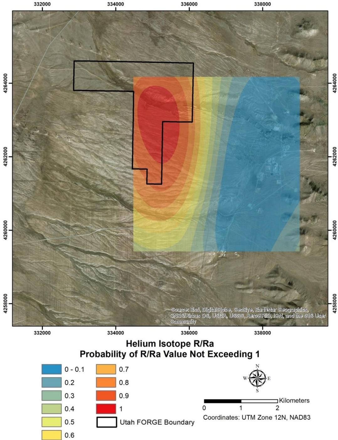
**Figure II.1.19.** The probability of helium R/Ra resembling background values. The FORGE site, where data was available, generally has probability in the range of 0.08-1.0 indicating a high certainty of no hydrothermal activity, while the area near Roosevelt Hot Springs, to the east, shows low probability indicating an active system.
