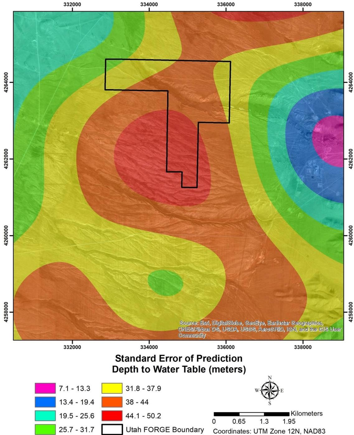
**Figure II.1.22.** This map shows potential spatial error for the top of the water table in depth m. This was created using simple kriging standard error of prediction. The error in the FORGE area is relatively high, however, the range of depth to ground water is relatively shallow in nearby wells, ranging from 15 m to 166 m.
