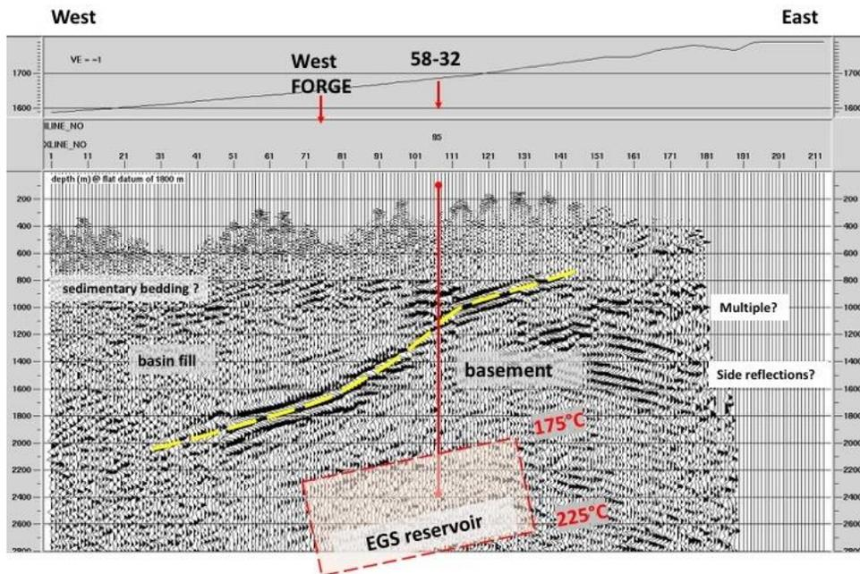
**Figure II.1.6.** 2D and 3D seismic reflection surveys and profile over the FORGE site; A) Seismic survey locations acquired November, 2017; B) East-west profile on Inline 95, which runs through well 58-32. Basement contact is highlighted with dashed yellow line.
