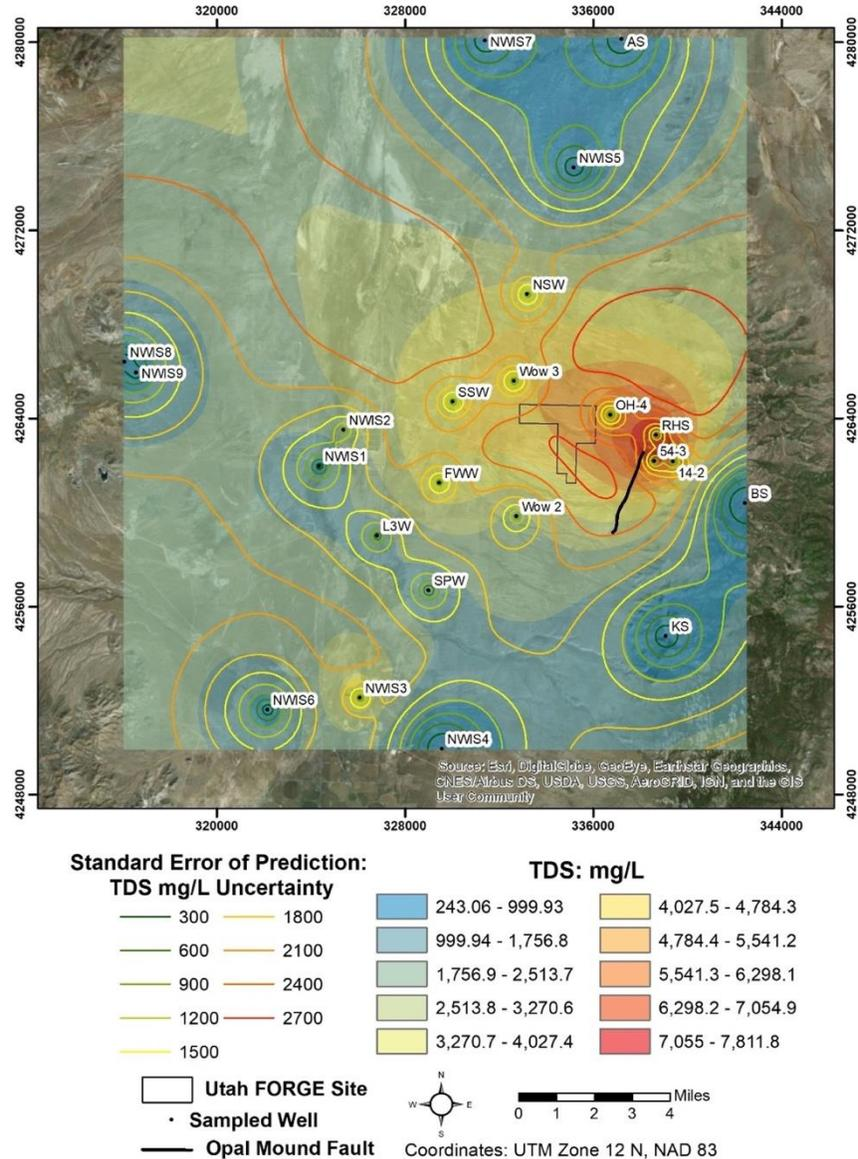
**Figure II.1.21.** This map shows simple kriging standard error of prediction contours superimposed on a TDS statistical surface. The error is relatively high in at the FORGE site.
