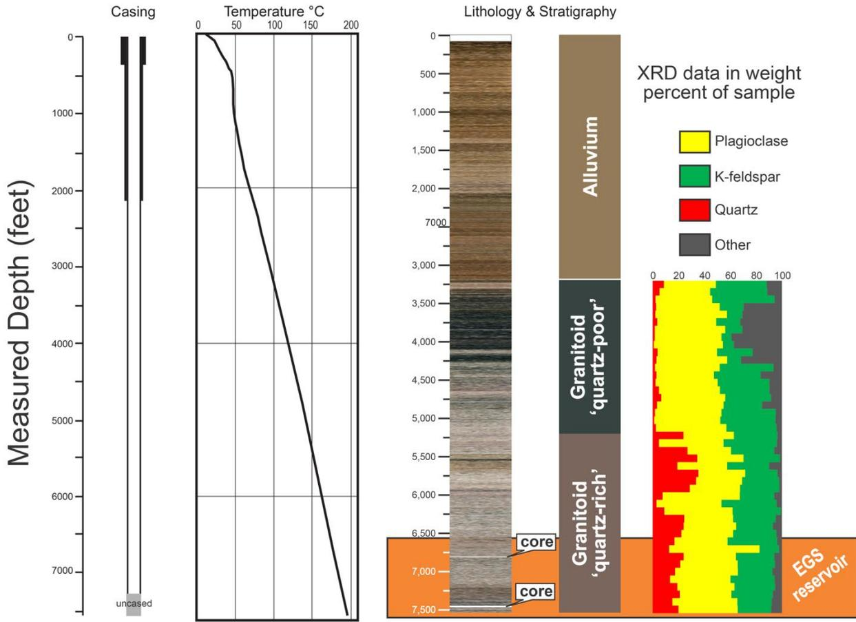
**Figure II.1.8.** Well 58-32 casing profile, temperature gradient, stratigraphic and lithologic columns, and quantitative mineralogy, based on X-ray diffraction and thin section analyses.
