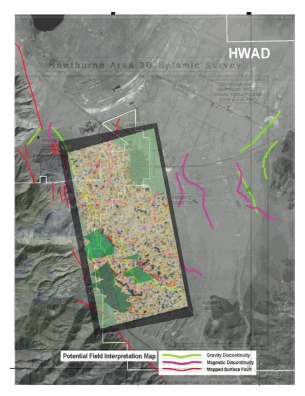
This image is an overlay of the survey area with previously mapped discontinuities. The spatial fit is not exact but it is apparent that there are matches between the multiple study types. The three faults we interpreted also appear as gradients in the geophysical potential-field maps.
