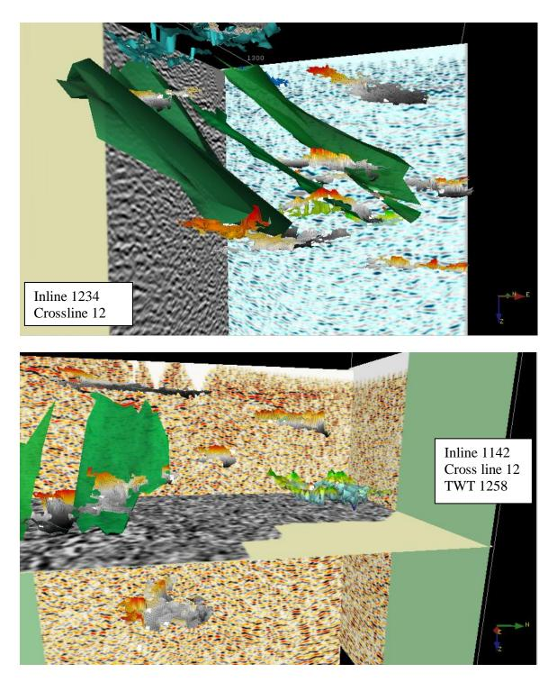
There is coherency in tracked strata in the range of 400-500 ms, which would correspond with the volcanic sediments in the upper basin, and in the range of 1100-1200 ms. With a migration velocity of 8000 ft/s, 1100 ms corresponds to a depth of 4400 ft.
