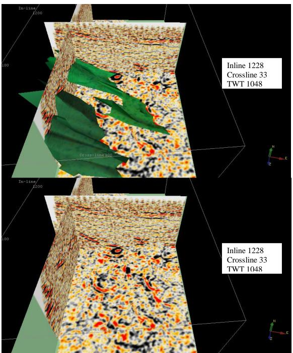
There are three faults in green that are the most readily picked through vertical sections. These begin at an inline of 1011 and can be followed well through inline 1248. They have eastward dip, and the reflections enter the volume at a minimum TWT of approximately 400 ms. As seen in the image, they follow the fault strike displayed in the time section.
