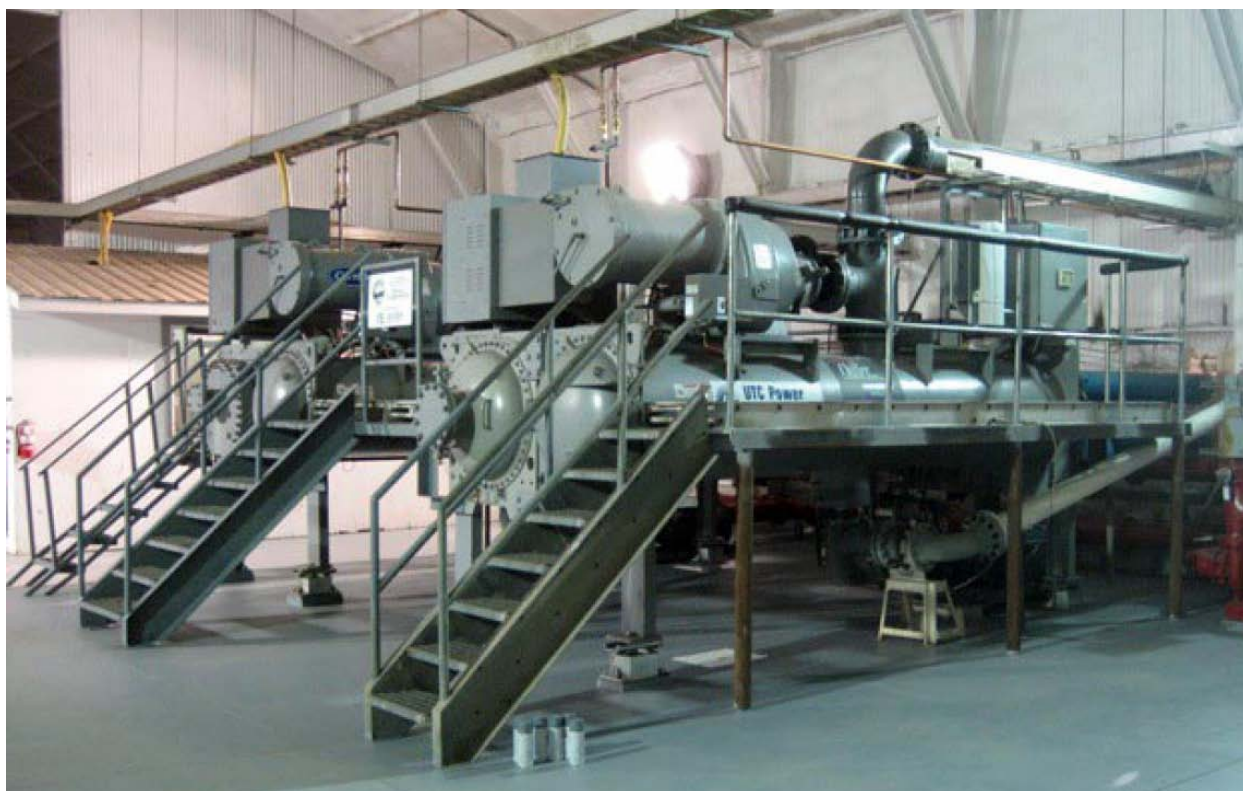
Figure 20: PureCycle binary units at Chena, Alaska (Holdmann, 2007)
