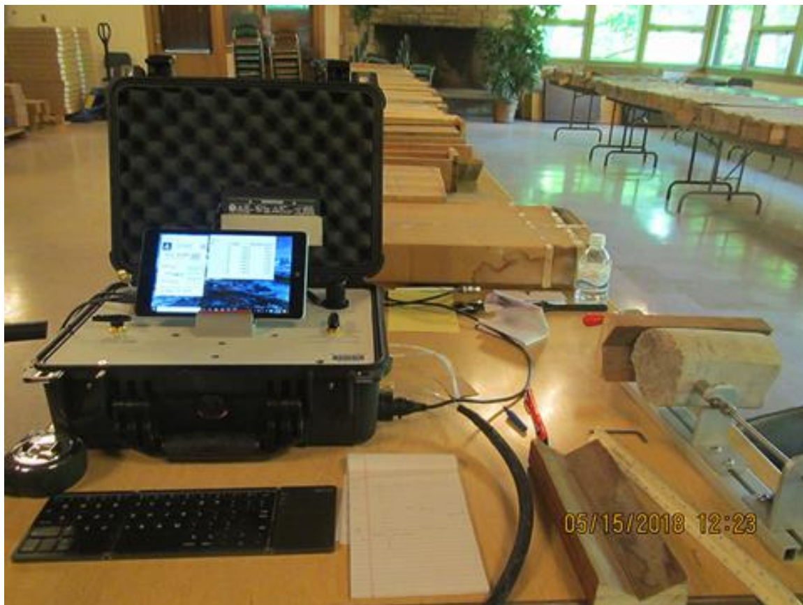
Figure 6: Core Labs PPP-250 Minipermeameter in operation. The instrument's probe is held tightly against the face of a core sample (on the right) while air is injected into the rock at approximately 26 psig. The instrument itself (on the right) measures the rate of gas uptake by the sample and computes the sample's permeability which is stored digitally on a small tablet computer (also on the right). The quantity being measured is k_{hAir} (horizontal permeability to air) in millidarcies (mD).
