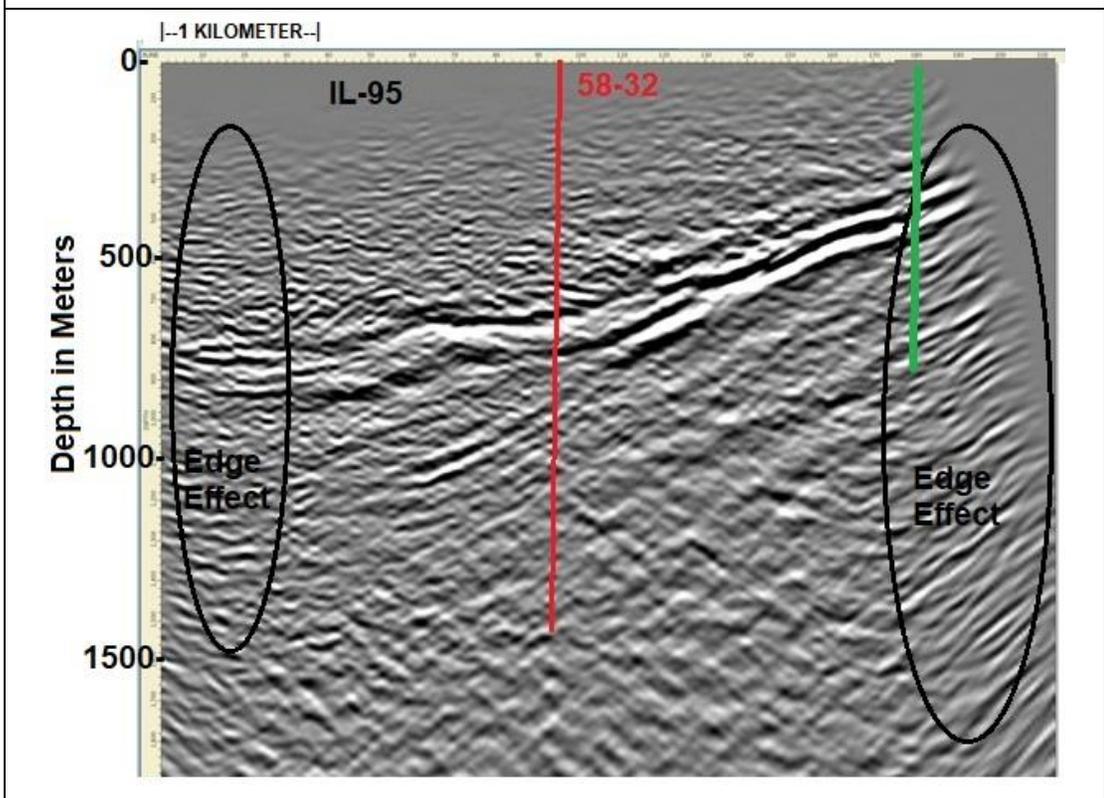
**Figure 5.** Top: Unmigrated time shows lack of reflections on the west, possibly because of low fold; also indicated is low fold on the east end. Vertical green line indicates eastern extent of shallow surface coverage. Bottom: Migrated depth of A. Migration edge effects can be seen on the west end. The granite reflection has migrated east of the green line which is valid. Migration artifacts are deeper.
