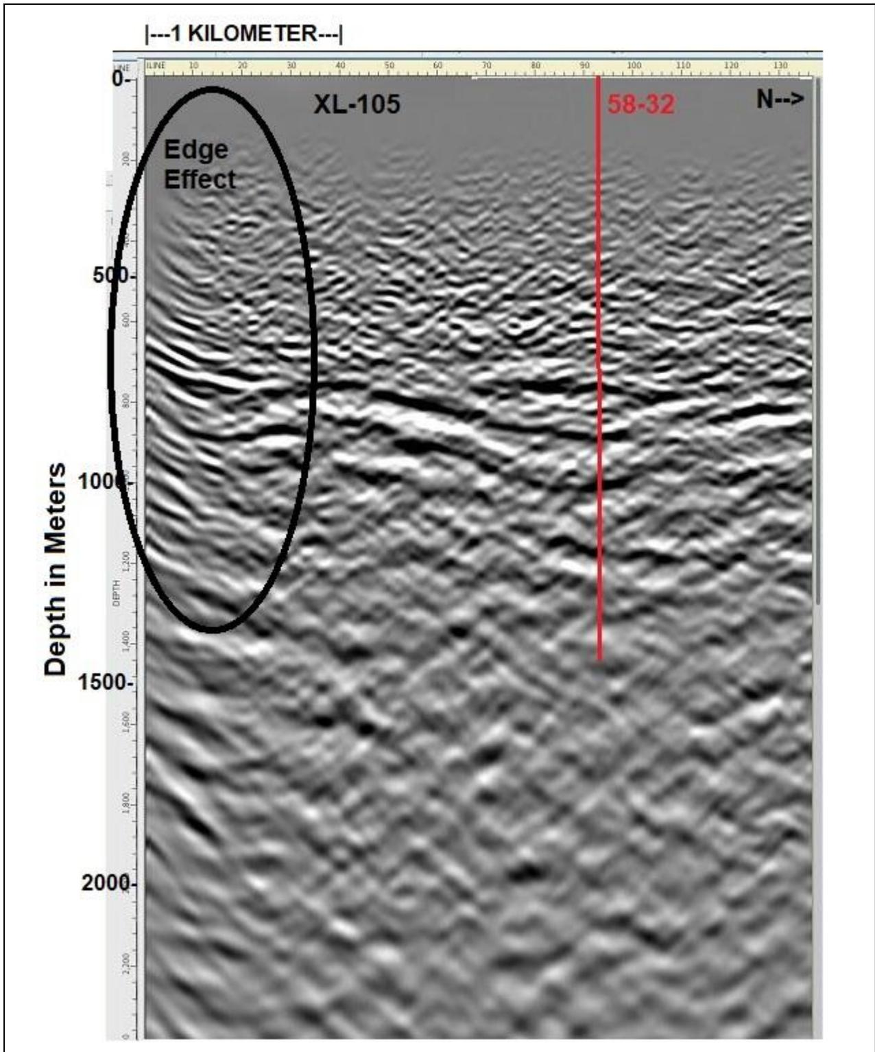
**Figure 4.** North-south crossline 105 (XL-105) intersecting test well 58-32 indicating the 3D “edge effect” at the southern end of the line. This effect arises from the low fold and the migration process (migration artifact) and should not be considered valid information.
