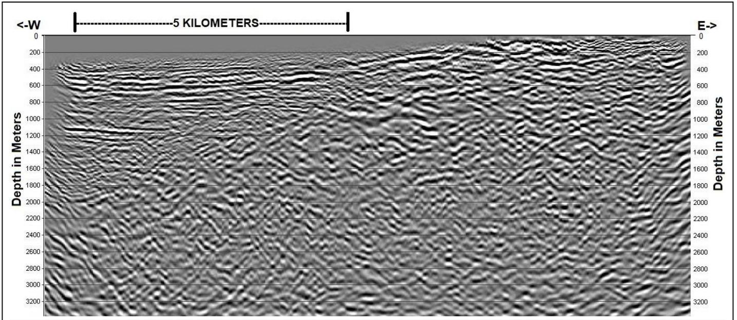
Figure 12: Legacy Line 5. Prestack depth migration by LSNS. Subhorizontal reflections are better resolved than in the 2016 reprocessing shown in Figure 11, bottom.
