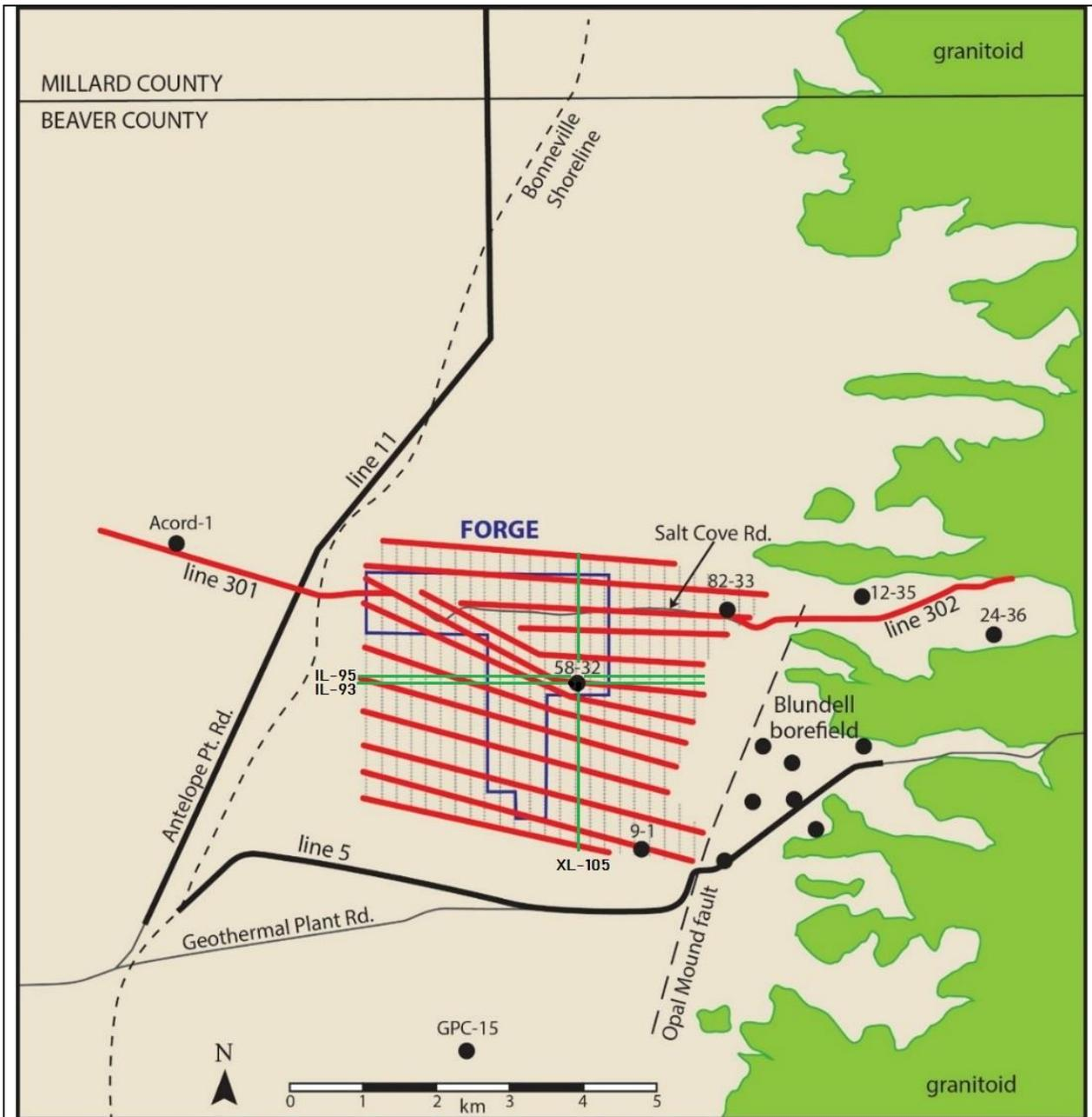
**Figure 1:** Seismic survey profile locations. The 3D survey area comprises 13 red source lines (vibrator point locations 50 m apart), and 27 gray geophone lines geophone locations (oriented N-S, geophone interval 50 m). Red lines 301 and 302 are new 2D seismic lines; heavy black lines labeled 5 and 11 are legacy 2D lines licensed from Seismic Exchange, Inc. After Miller et al. (2019). Green lines are 3D inlines (IL) and crosslines (XL) discussed in this report.
