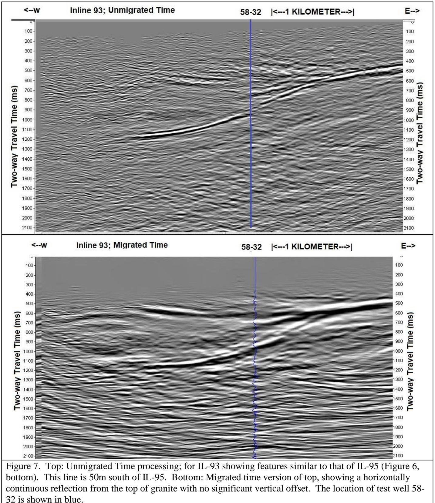
Figure 7. Top: Unmigrated Time processing; for IL-93 showing features similar to that of IL-95 (Figure 6, bottom). This line is 50m south of IL-95. Bottom: Migrated time version of top, showing a horizontally continuous reflection from the top of granite with no significant vertical offset. The location of test well 58-32 is shown in blue.
