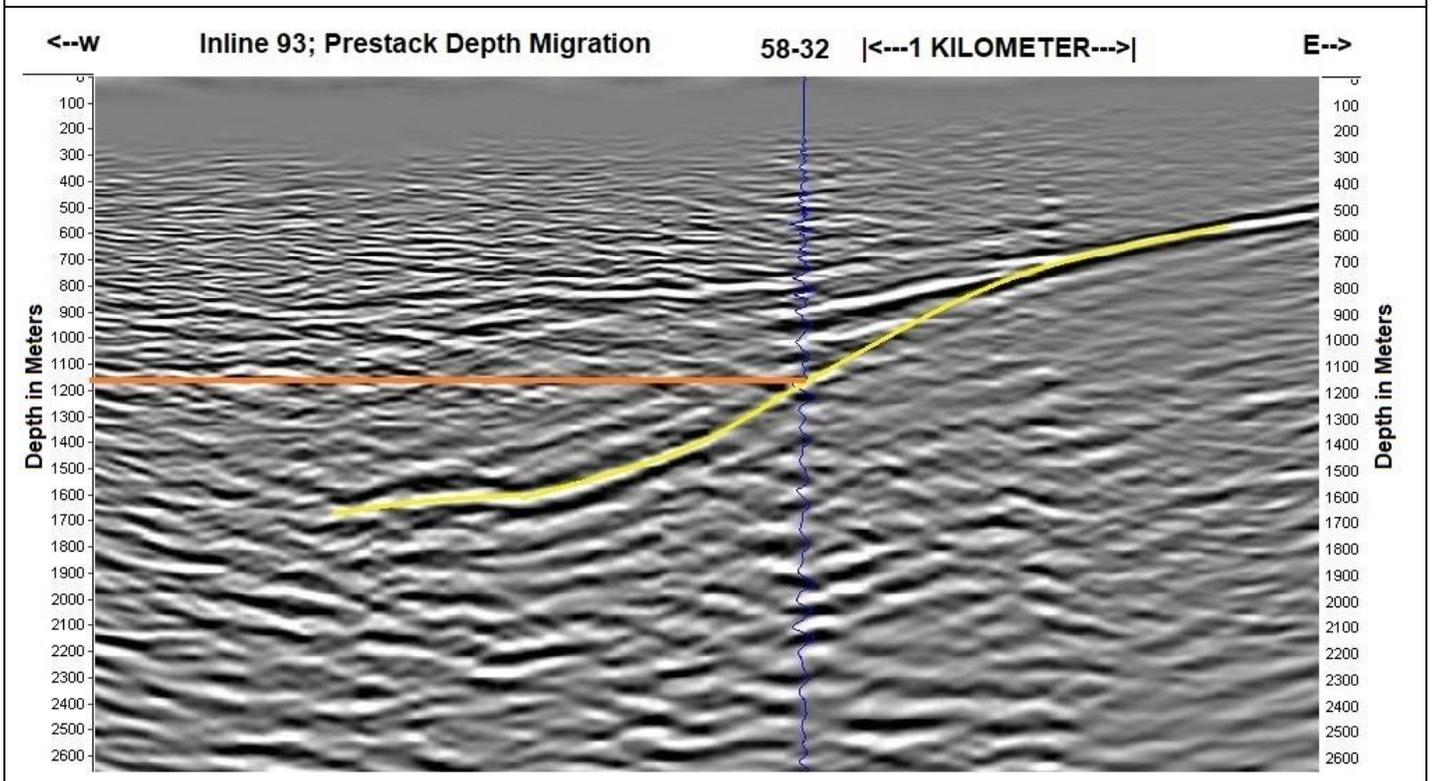
Figure 8. Top: Uninterpreted estimated anisotropic prestack depth migration. Bottom: Interpreted version of the top. Yellow line indicates the author's interpretation of the top of granite reflector. The horizontal amber line indicates the depth to top-of-granite at test well 58-32. This depth corresponds well with the depth of granite from logs and cuttings in well 58-32. The location of test well 58-32 is shown in blue.
