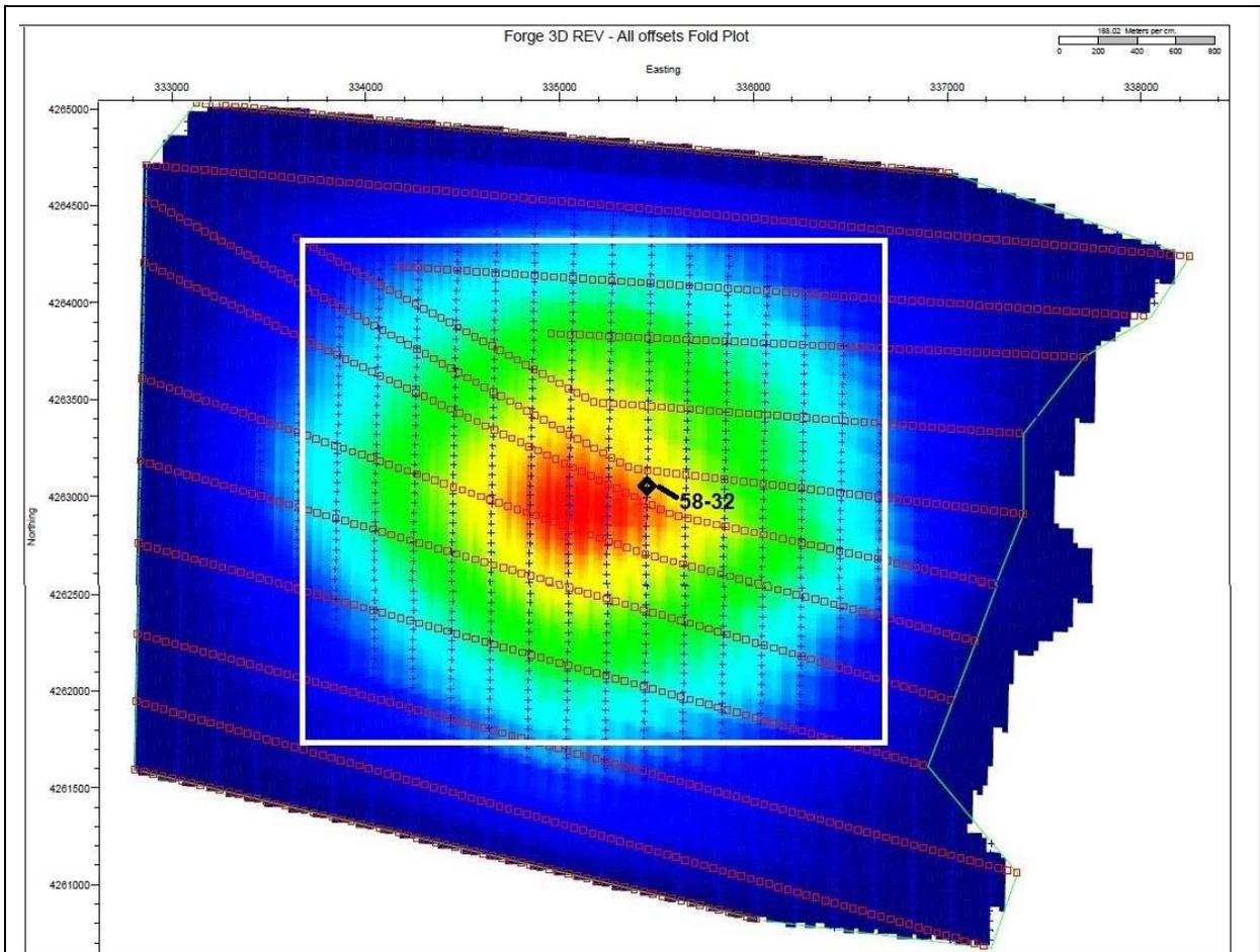
**Figure 3.** Diagram indicating relative minimum and maximum seismic fold (number of traces contributing to a CDP bin) based on the 3D recording configuration. Blue = Minimum fold; Red = maximum fold. White box indicates the general area where the 3D data should not be affected by edge effects of low fold and migration artifacts. Care should be taken when interpreting data outside of this box.
