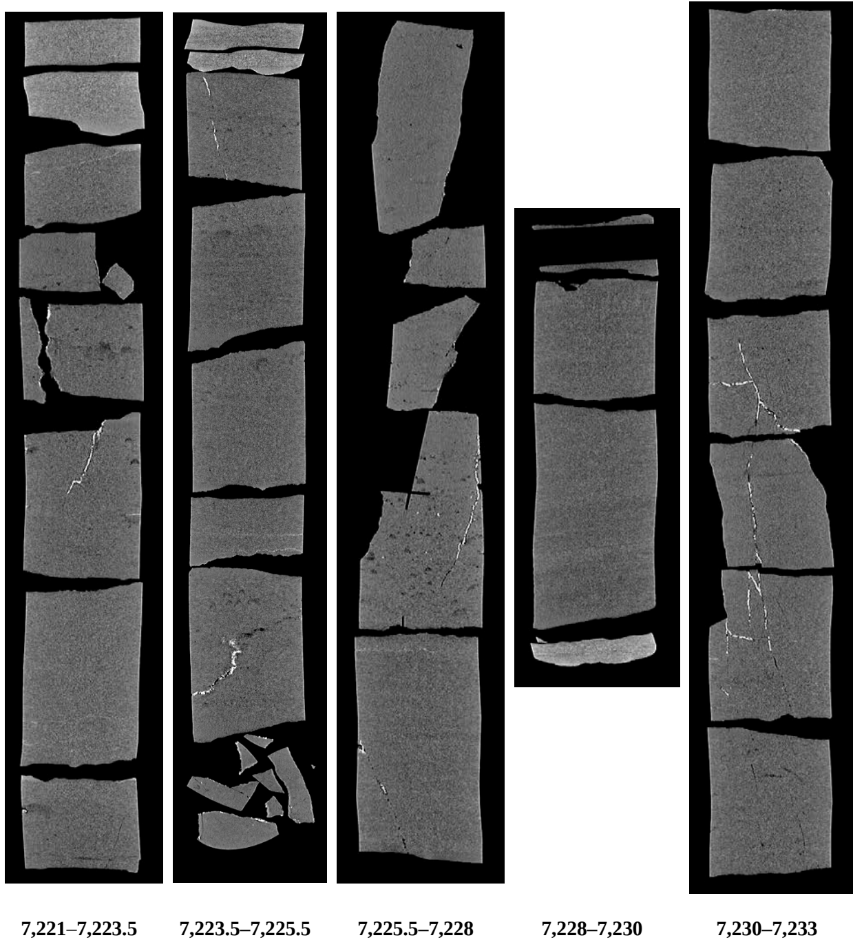
Figure 55: 2D isolated planes through the vertical center of the medical CT scans of the Pres-119 core from 7,221 to 7,233 ft.
