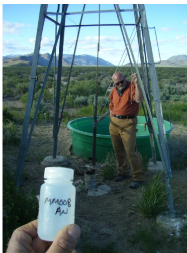
Figure 18: Water sample MM008 was taken from a non-functioning windmill. Mike Schramm is holding a makeshift block and tackle (minus the block) that we used to hold the top of the well in a position to get a bailer down the well. The windmill's pump rod is broken just above the top of the picture, just under the vanes. A large raven's nest with fledglings attest that it's been broken for a number of years.
