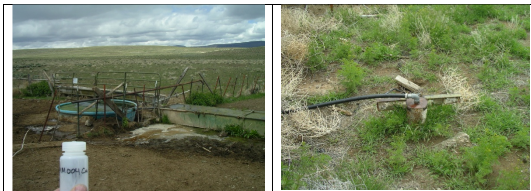
Figure 13: Water sample MM002 was collected from a developed spring. The water sample was taken from the spring box collection culvert using a rope to lower the sample pitcher some 10ft below the surface.
