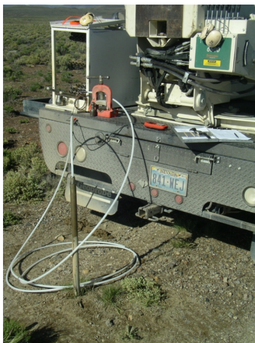
Figure 11: The equilibration test at site MMTG#1: The probe rods were at depth, the RTD Installed and temperature recorded over time.
