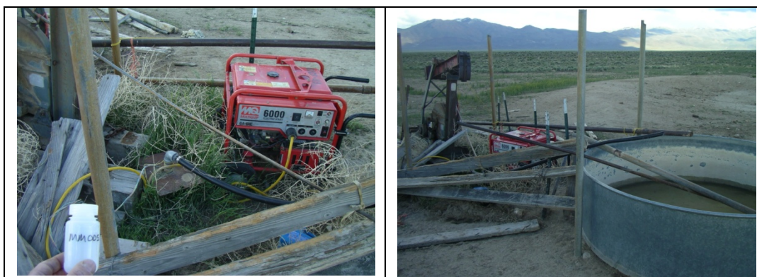
Figure 15: Water sample MM005 is a stock well that was not running on arrival. The generator was turned on, after adding gasoline, to run the well prior to sampling. The photo to the left is the wellhead and the photo on the right is the stock tank. Note the white ( \text{CaCO}_3 ) precipitate on the tank.
