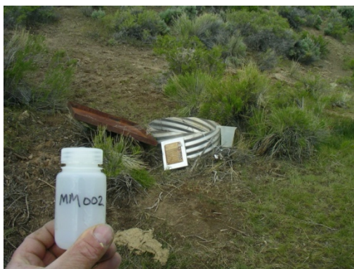
Figure 13: Water sample MM002 was collected from a developed spring. The water sample was taken from the spring box collection culvert using a rope to lower the sample pitcher some 10ft below the surface.
