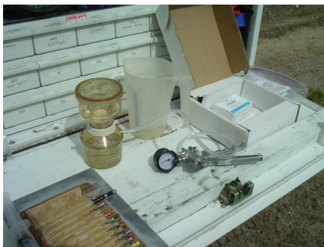
Figure 19: All water samples were filtered using the NALGENE Filter Holder with Receiver (Cat. No. 300-4050) and a Mighty Vac vacuum pump.
