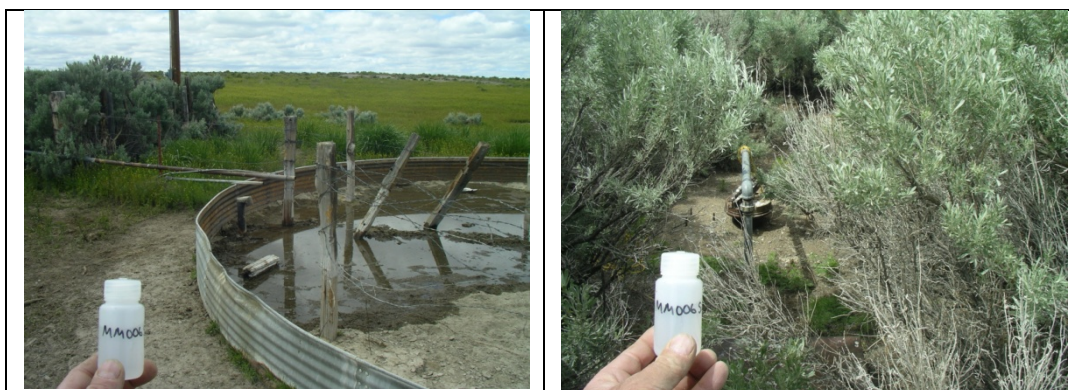
Figure 15: Water sample MM005 is a stock well that was not running on arrival. The generator was turned on, after adding gasoline, to run the well prior to sampling. The photo to the left is the wellhead and the photo on the right is the stock tank. Note the white ( \text{CaCO}_3 ) precipitate on the tank.
