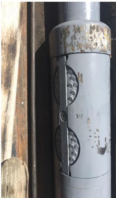
Figure 3. For the packer shown in Figure 2, not only the rubbers were damaged, but the slips had failed. The photograph at left shows new slips. The photograph at right shows the upper slips on the packer recovered from Zone 3 on May 3, 2019. The arrows highlight the damage.
