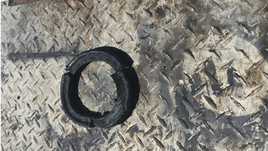
Figure 2. This photograph was taken on May 3, 2019 after recovery of the packer from above Zone 3. It shows a failed sealing element. An observer reported: "When packer pulled above the slips the broken ring fell into our hands." There was a significant amount of drag while recovering this tool (refer to Figure 4).
