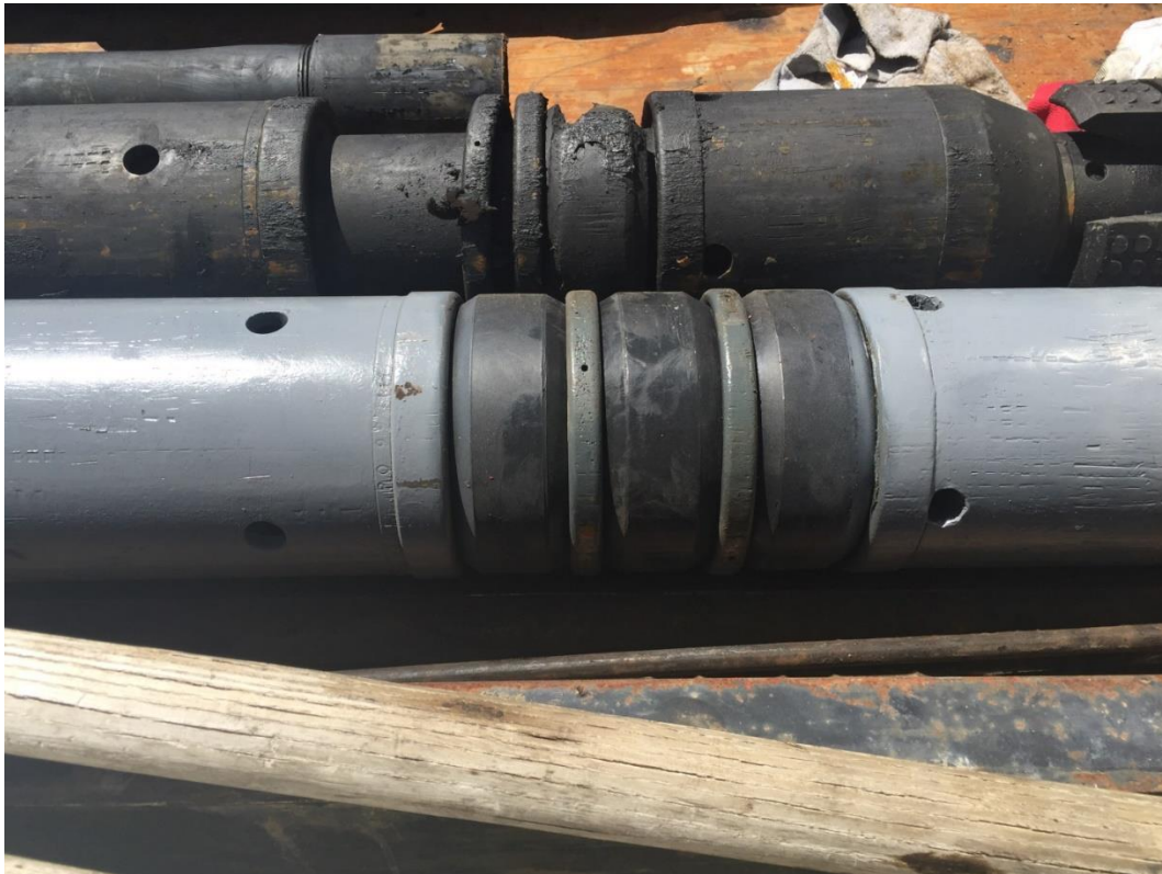
Figure 1. This image shows a new packer element (bottom) and the retrieved packer element from Zone 1 (run above the perforations at 6964 to 6974 ft measured depth).
