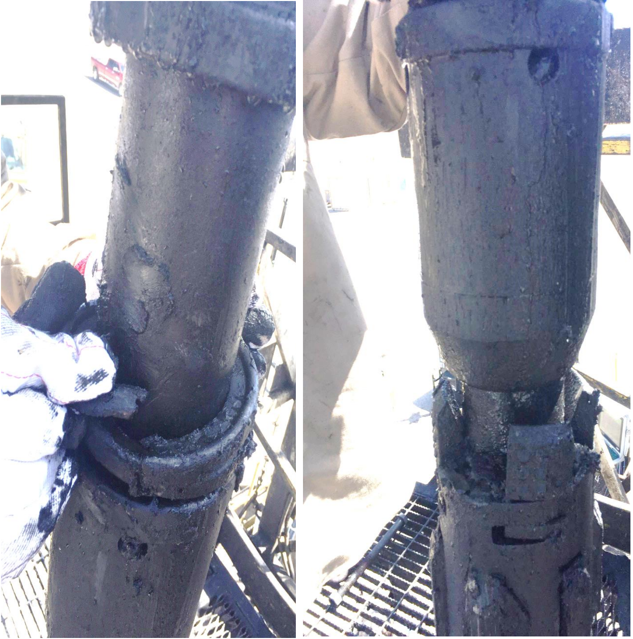
Figure 4: Two views of the Zone 3 packer after recovery. The broken rings caused significant drag.
