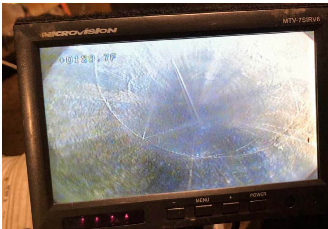
Figure 3: Water leaking (jetting) into E1-P on May 25 th (note depth registration in this image is approximate, +/- 1 foot).
