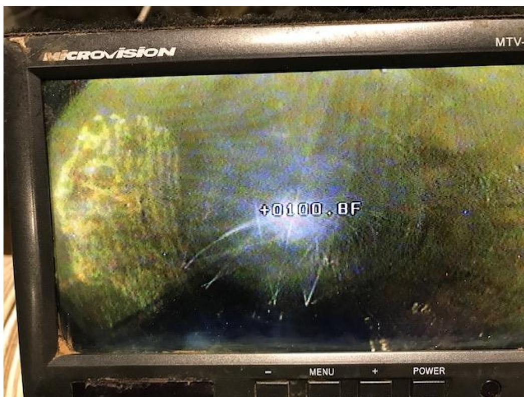
Figure 4: Water leaking (jetting) into E1-P on December 21 st (note depth registration in this image is approximate, +/- 1 foot).
