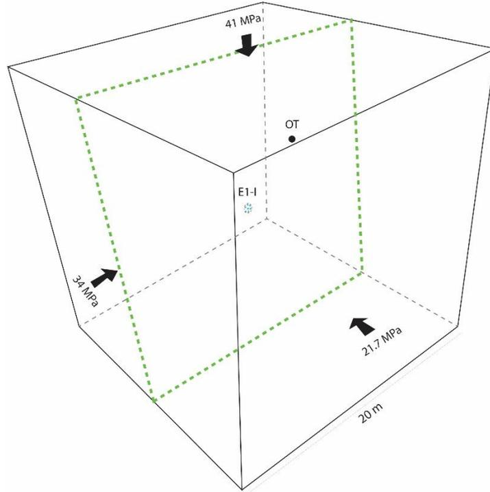
**Figure S2.** (a) Numerical Model setting. The green dashed line pre-figures the direction of propagation of the hydraulic fracture as it was deduced from the orientation of the field borehole displacements and induced seismicity. Injection is initiated at E1-I in a zone of this fictive plane that has been previously broken to figure the initial fracturing during stimulation step 1. That zone is about 1 meter diameter (green circles patch at E1-I).
