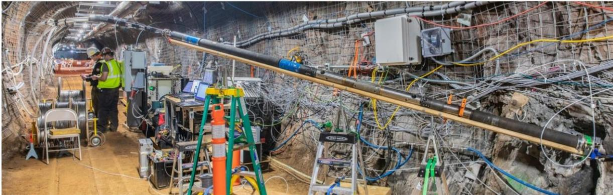
**Figure S1.** SIMFIP probe before deployment in borehole E1-I from the Sanford Underground Facility gallery 1478m depth.
