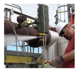
Figure 7. Fluid sampling sites, Roosevelt Hot Springs: A) mini-separator on a two-phase line, upstream of the separator, with steam jetting from the gas port; B) pipeline downstream of a separator with a drip tank containing cooled thermal water.
