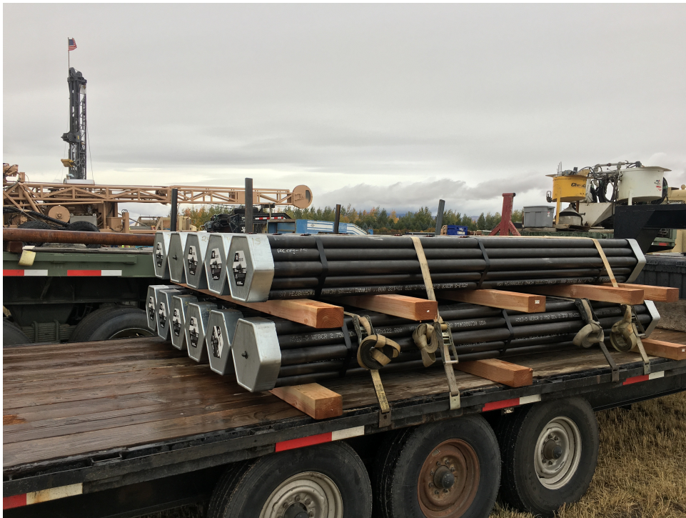
Arrival of new NQ coring drill rod.
