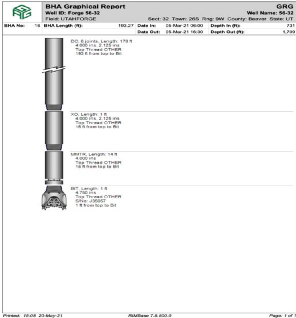
Figure 35: 4-3/4 in. BHA #16 to clean-out cement inside 5-1/2 in. casing
