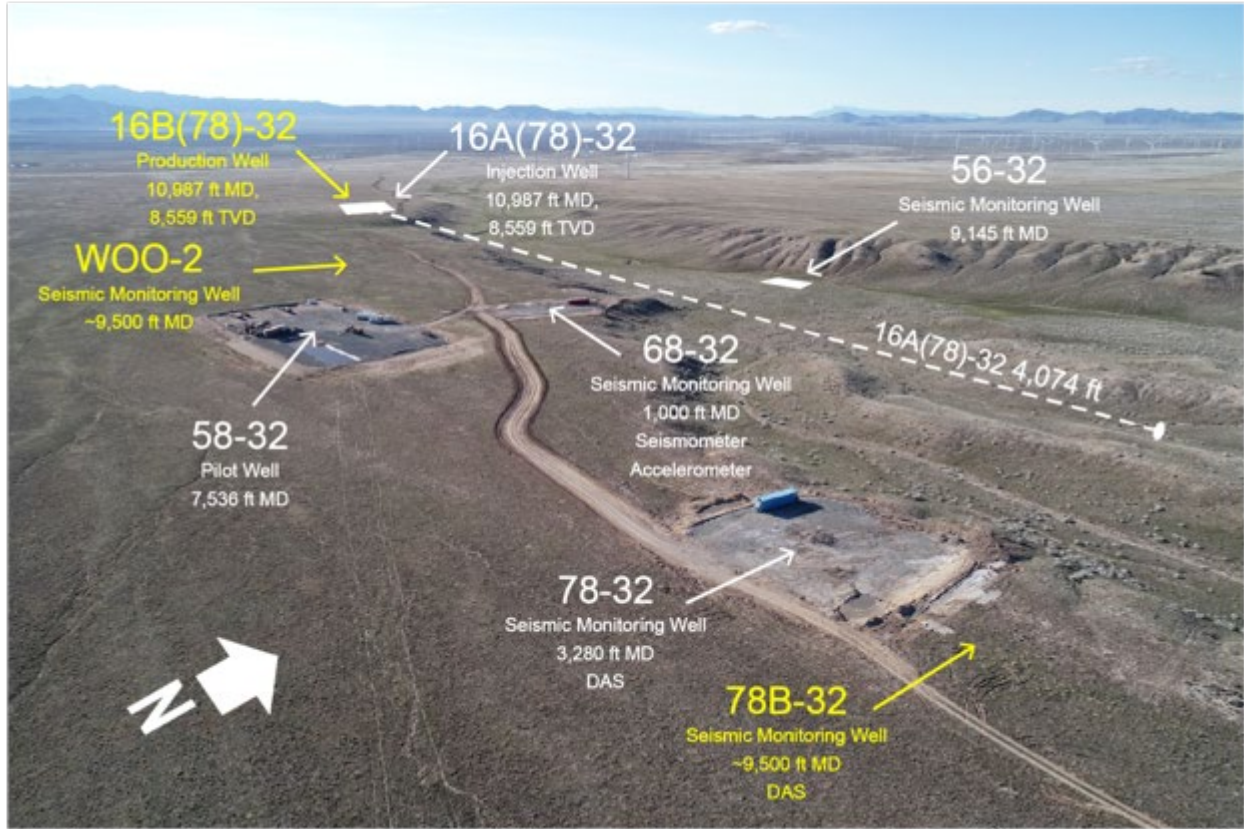
Figure 2: Aerial view of surface locations of Utah FORGE Wells. Drilled wells are shown in white, planned in yellow.
