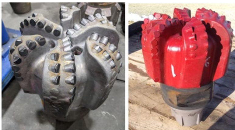
Figure 60. This bit, TKC63, drilled 742 ft with an average ROP of 47 fph. Bit grading was 1-3-CT-S-X-I-WT-PR.
