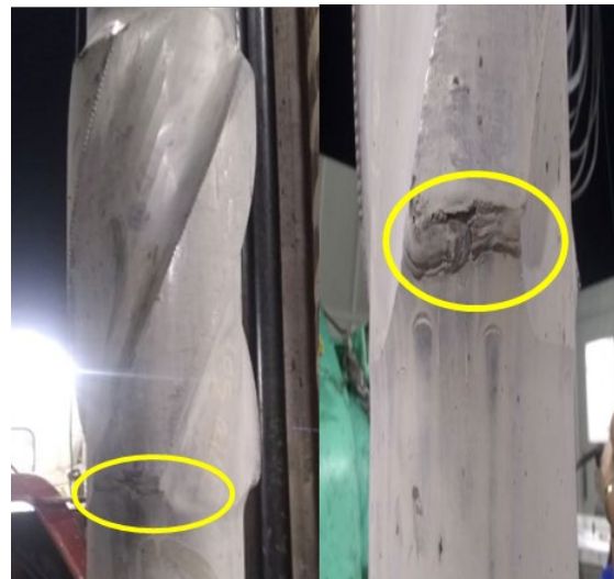
Figure 39. Bit SKC613M-01C and stabilizer damage. Bit grading: 1-1-WT-A-X-I-NO-BHA
