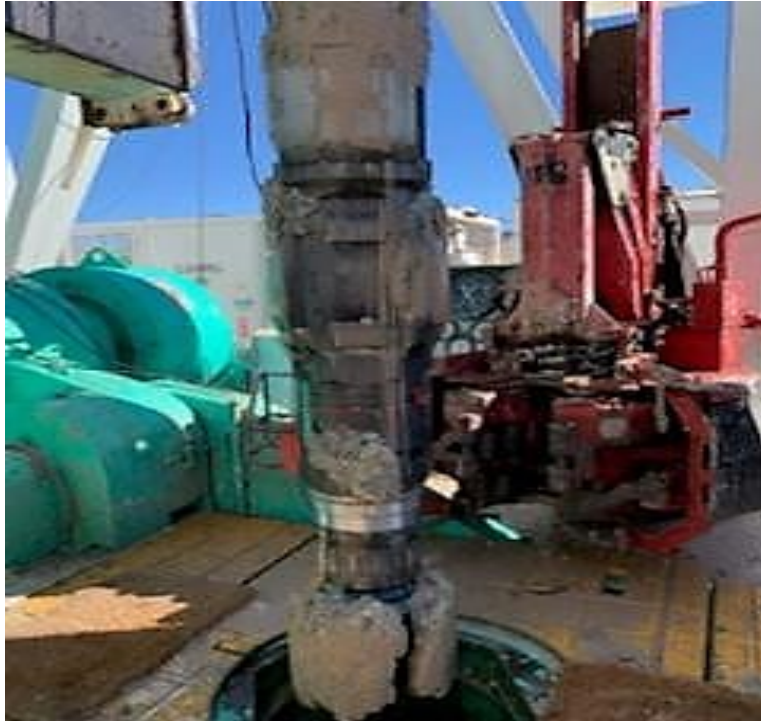
Figure 1. Evidence of bit balling
