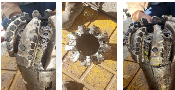
Figure 32. Canamera bit CCI 913, after core run 3.
