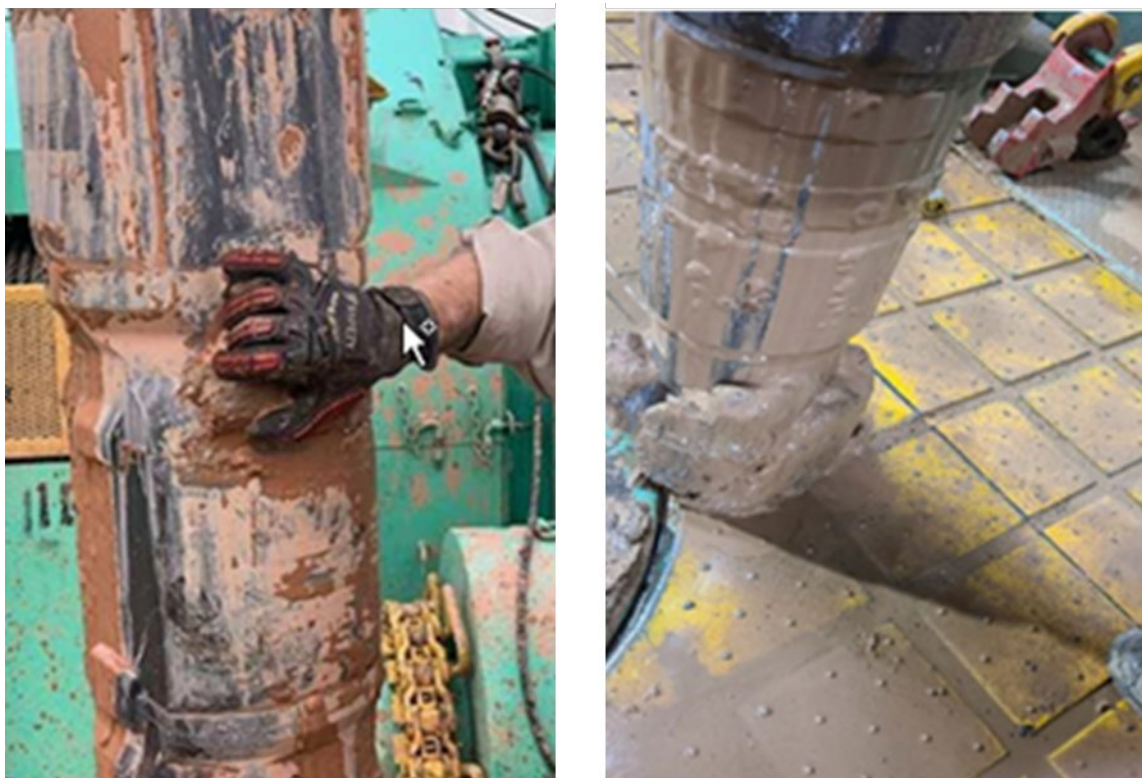
Figure 16. Two examples of clay-like material attached to the BHA and impeding ROP.
