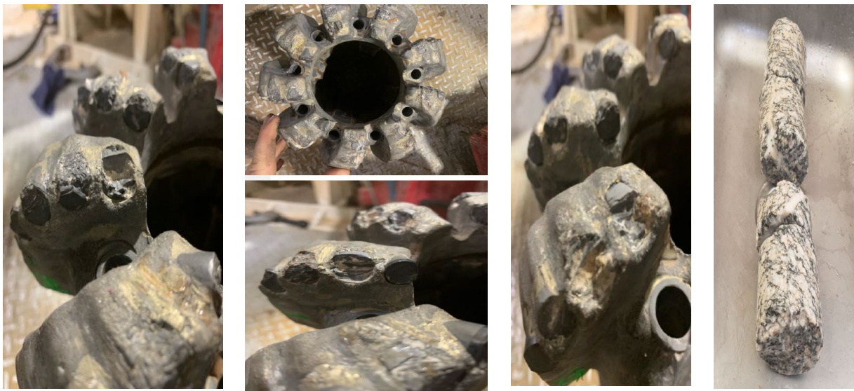
Figure 28. Core Run 2, bit DBR. Core recovered is shown at right.
