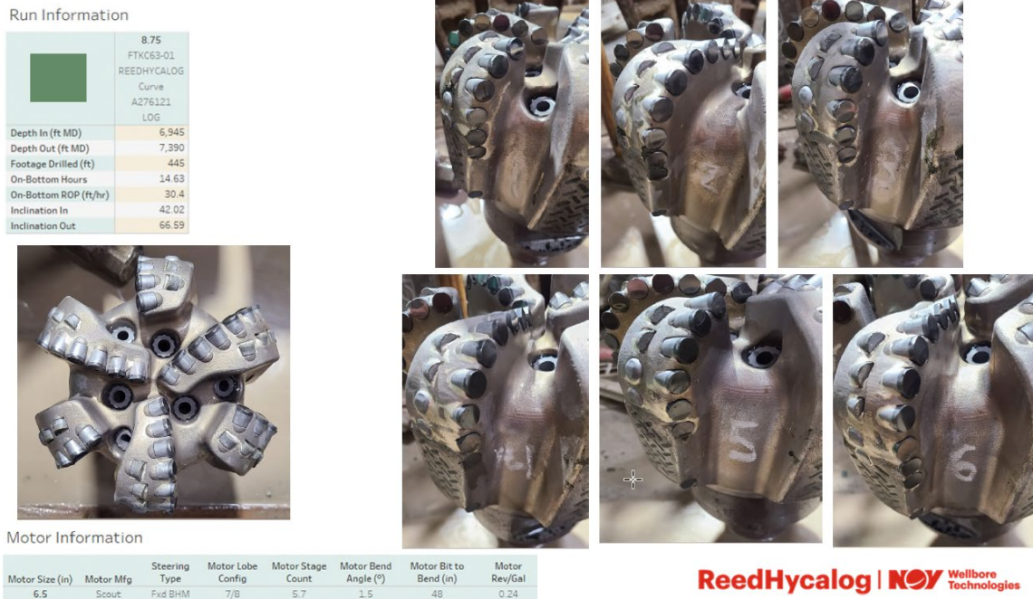
Figure 45. FTKC63-01. Bit grading was 1-1-WT-A-X-I-NO-BHA
