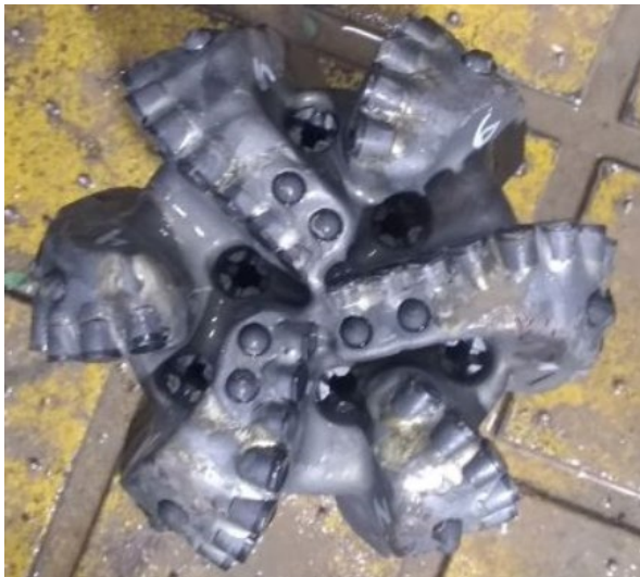
Figure 39. Bit SKC613M-01C and stabilizer damage. Bit grading: 1-1-WT-A-X-I-NO-BHA
