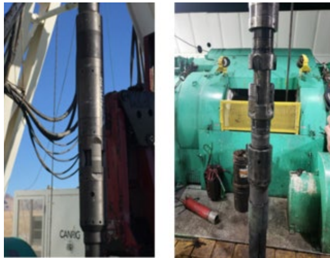
Figure 67. Photograph of the packer (before and after running).
