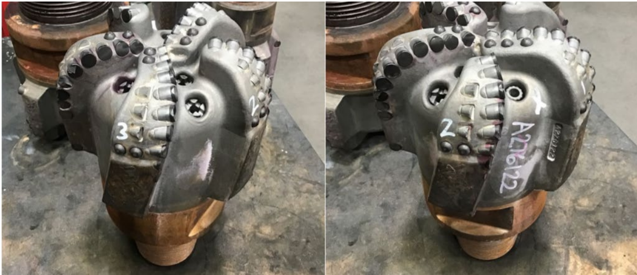
Figure 42. SKC513M-L1A. BHA pulled for non-bit-related reasons. Bit grading: 2-2-CT-S-X-I-WT-BHA. TCCs may have limited DOC/ROP (60K was applied). The subsequent bit had no TCCs and outperformed this bit.
