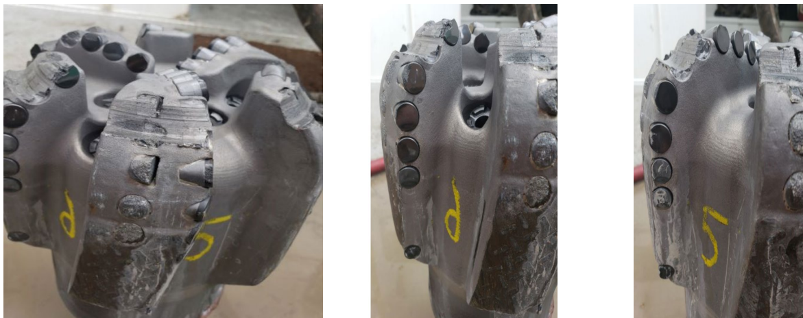
Figure 58. This bit is an FTKC63-01. Bit grading: 2-7-RO-S-X-I-CT-PR - ring out. The bit drilled 684 ft with an average ROP of 41 fph.
