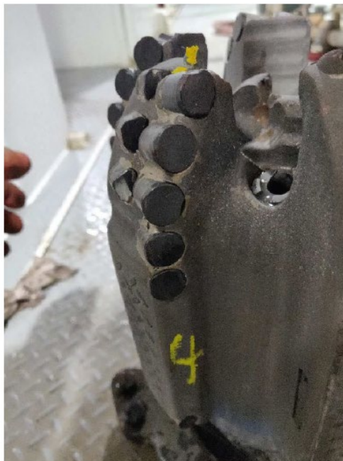
Figure 30. ReedHycalog TKC66-P3 bit. Bit grading: 8-3-CR-C-X-I-CT-CP.
