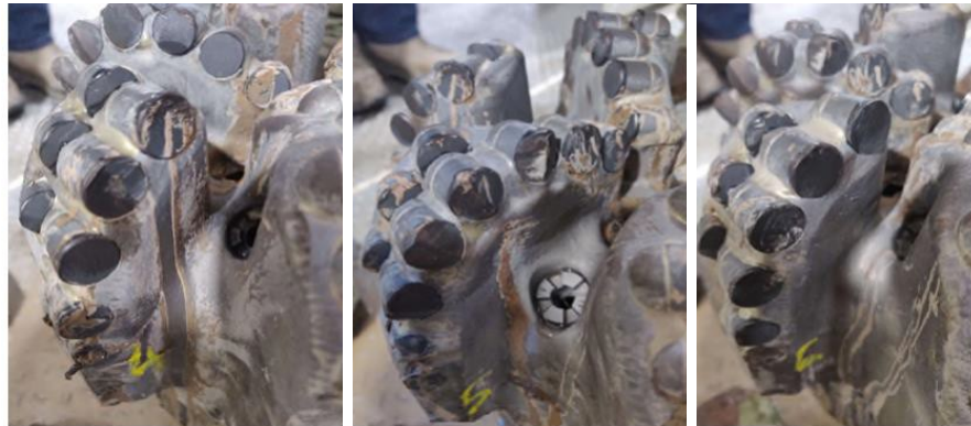
Figure 20. Smith XS 616. This bit, as with all others showed a characteristic rapid ROP-drop in the first 100 feet or so that was drilled. The run showed the inefficiency of 16 mm cutters. Schlumberger Smith's maximum allowable weight on bit was 45,000 lb f and, at the time, it is felt that one needs at least 50,000 lb f to engage all the cutters and prevent bit whirl. The VRSS was having difficulties holding angle and therefore a lower weight on bit was mandated.
