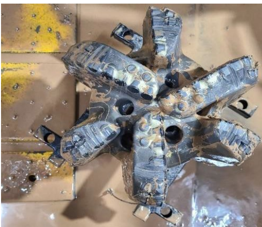
Figure 13. Smith MDSi616. This bit drilled from 4,552 to 4964 ft MD. The apparent initial failure mode sequence could have been micro-chipping and spalling. The failure may have been compounded by potential axial vibration. This bit run, like most others in the granite, (refer to Figure 14), showed high initial ROP and a relatively rapid drop thereafter. Rhyolitic layer in Well 58-32 suggests higher compressive strength near the top of the granite. Two rhyolites were encountered in well 16A(78)-32.
