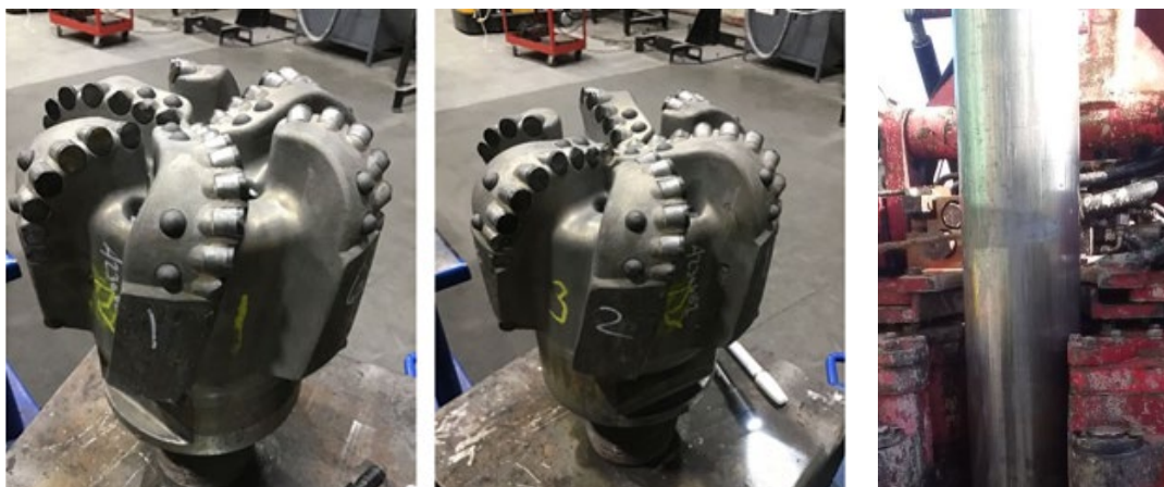
Figure 52. ReedHycalog SKC613M-O1C. The bit grading was 2-1-CT-C-X-I-CT-LOG. The bit was pulled to log the hole. The TCCs are 2mm off tip. The ROP was the highest to this point. There were weight transfer issues after drilling 114 ft. At right is a drill collar in the hydraulic tongs.
