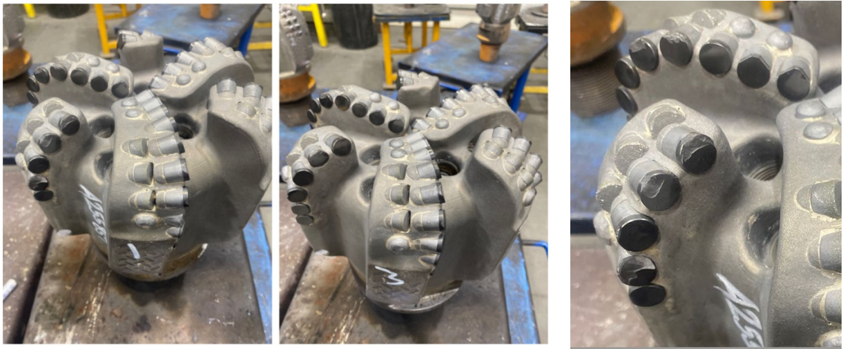
Figure 36. NOV Reed Hycalog TKC63 PDC. This bit exceeded performance expectations. These were the first 13 mm cutters used in the granite and the 13 mm efficiency was demonstrated. The initial ROP drop-off was reduced and overall, the sustained ROP was higher (see Figure 30). Also, tool face control was important - shaped 3D Cutters in the cone and Torque-Control Components (TCC) in the cone (1.5mm off-tip). Bit grading: 1-2-WT-A-X-I-CT-PR.
