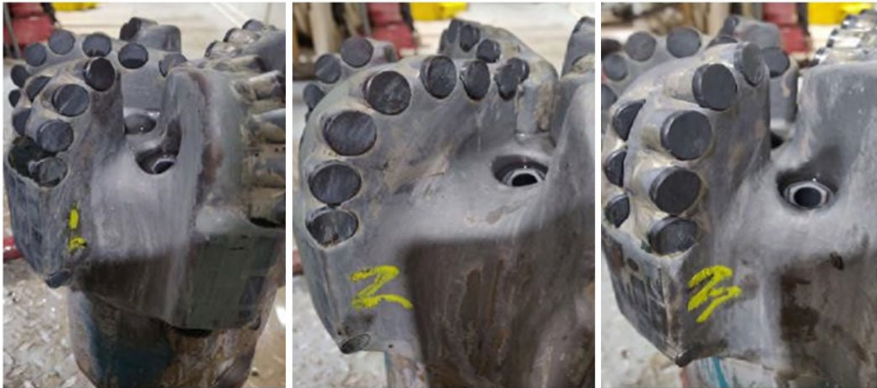
Figure 23. Photographs of the Ultra U616M after being tripped out. As with all other bits there was a characteristic rapid ROP-drop in the first 100 feet or so. 16mm cutter inefficiency was demonstrated. Ultra allowed all the weight on bit that was needed. The WOB ranged from 35K to 55K lb. The VRSS had difficulties holding angle and had to use lower weights - this was a major cause of low ROP.
