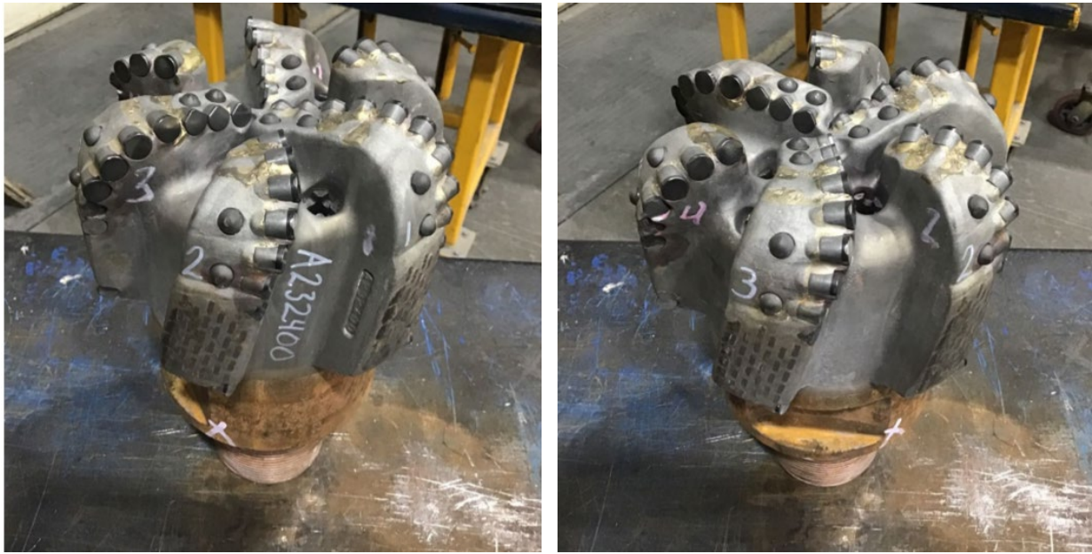
Figure 40 Bit SKC613M-01C. Bit grading: 1-1-WT-A-X-I-NO-BHA. This BHA was pulled because it became geometrically stuck (string stabilizer).
