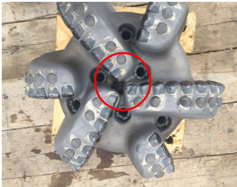
Figure 9. NOV TKC 66. Notice the highlighted damage inside the red circle.
