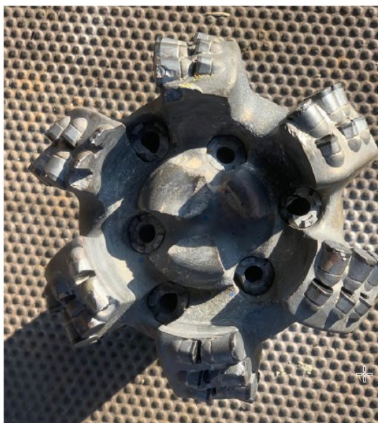
Figure 30. ReedHycalog TKC66-P3 bit. Bit grading: 8-3-CR-C-X-I-CT-CP.
