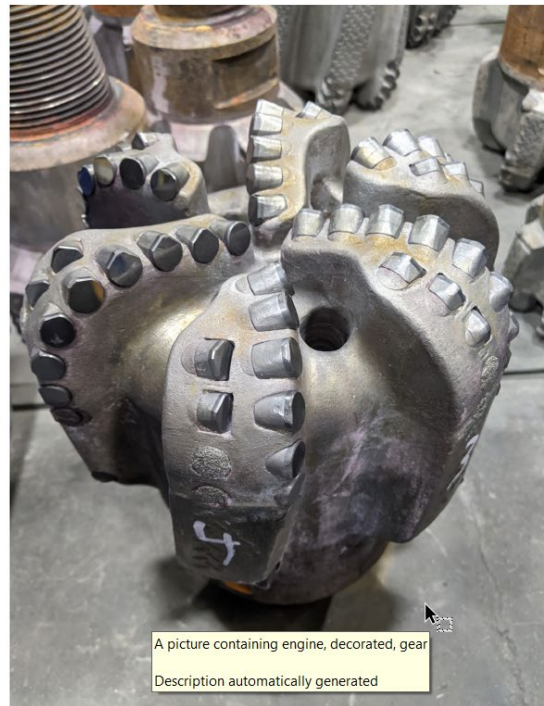
Figure 62. The bit was a TKC63-P1. This bit drilled 465 ft with an average ROP of 53 fph. Bit grading was 1-1-WT-A-X-I-NO-TD.
