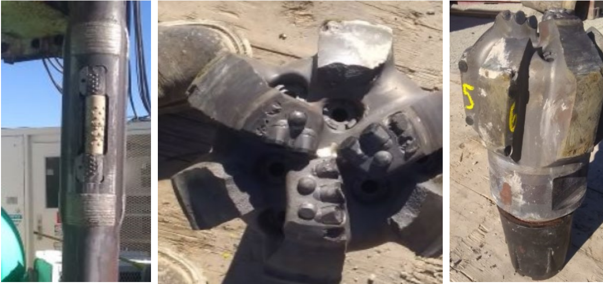
Figure 49. At left, a roller reamer was run above the motor. At right and in the middle panel is the bit, after recovery. TKC 63-C7 drilled 634 ft. It had a very aggressive tendency to build/drop/walk. Weight transfer issues were encountered after drilling 180 ft. ROP dropped and sliding became more difficult. Bit grading was 4-8-RO-S-X-I-BT-PR.
