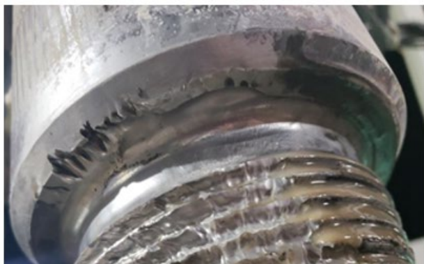
Figure 54. This BHA was pulled because of evidence of washout, which was diagnosed and the HWDP was replaced.
