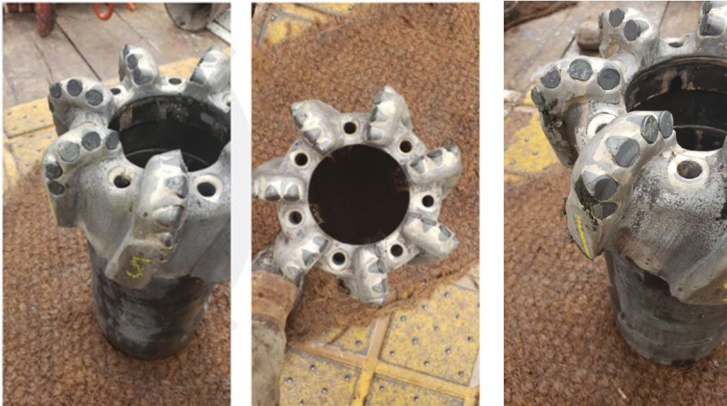
Figure 34. This is the bit for core run 4. The seven blades seemed to perform well.
