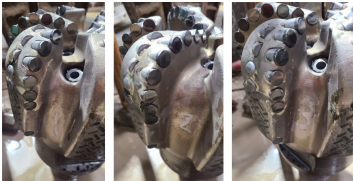
Figure 44. FTKC63-01. TCC has been removed and performance improved. Durability was sufficient. There was excellent dull condition and excellent build-rates. Landed the curve with this bit. Bit grading was 1-1-WT-A-X-I-NO-BHA.
