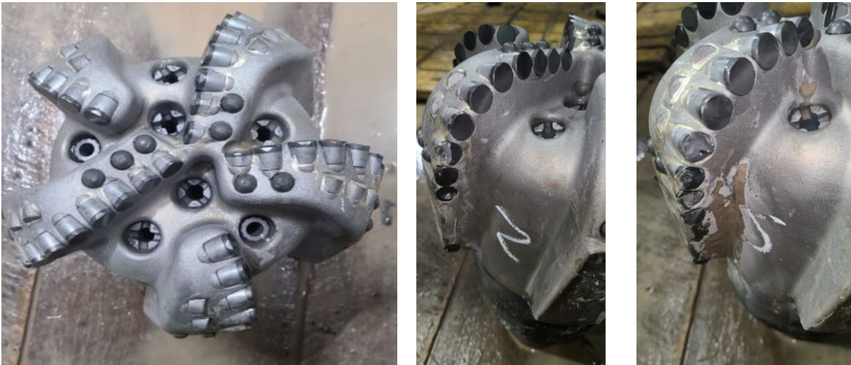
Figure 43. BHA pulled for non-bit-related reasons. Bit grading 2-2-CT-S-X-I-WT-BHA.
