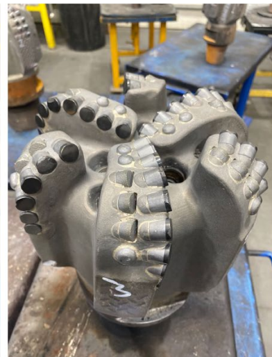
Figure 36. NOV Reed Hycalog TKC63 PDC. This bit exceeded performance expectations. These were the first 13 mm cutters used in the granite and the 13 mm efficiency was demonstrated. The initial ROP drop-off was reduced and overall, the sustained ROP was higher (see Figure 30). Also, tool face control was important - shaped 3D Cutters in the cone and Torque-Control Components (TCC) in the cone (1.5mm off-tip). Bit grading: 1-2-WT-A-X-I-CT-PR.
