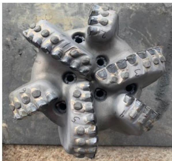
Figure 10. Rerun from BHA 02. Views of each blade are shown in Figure 11. This is a ReedHycalog TKC 66R1. It drilled 2908 feet in 59.58 hours at 48.8 ft/hr.
