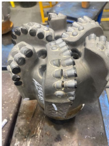
Figure 36. NOV Reed Hycalog TKC63 PDC. This bit exceeded performance expectations. These were the first 13 mm cutters used in the granite and the 13 mm efficiency was demonstrated. The initial ROP drop-off was reduced and overall, the sustained ROP was higher (see Figure 30). Also, tool face control was important - shaped 3D Cutters in the cone and Torque-Control Components (TCC) in the cone (1.5mm off-tip). Bit grading: 1-2-WT-A-X-I-CT-PR.
