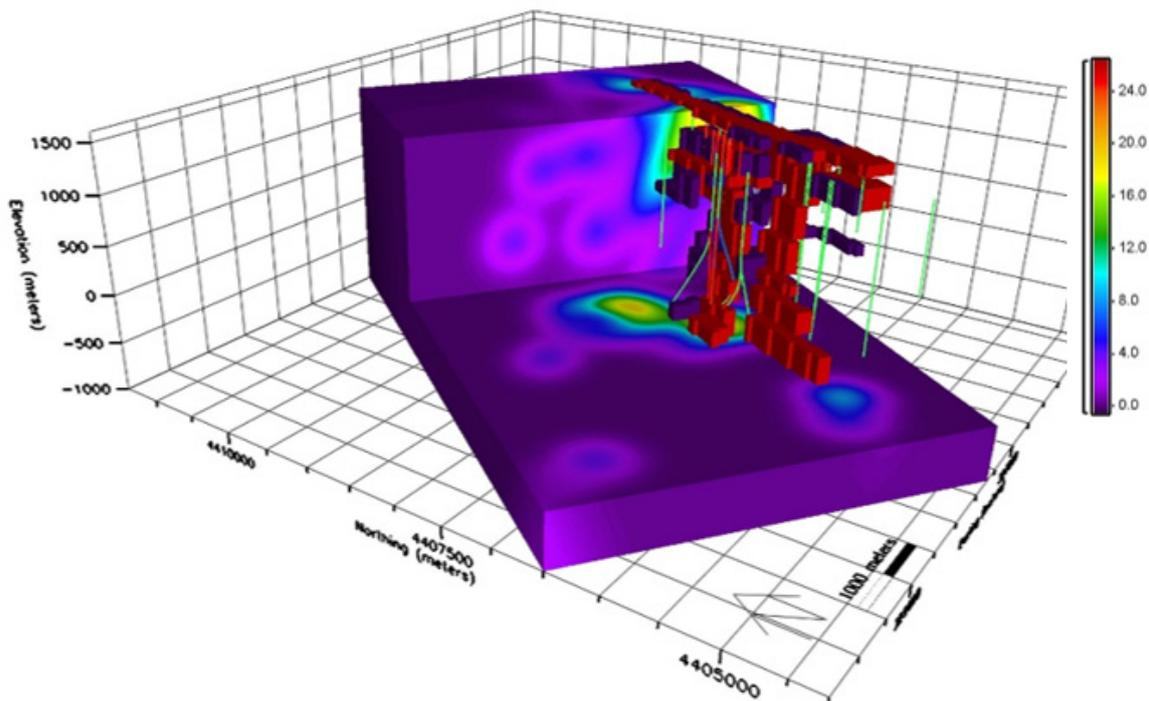
**Figure 8: Vertical fracture permeability from Ormat reservoir model (red cuboids indicate high permeability; purple cuboids indicate moderate permeability) overlain on fault intersection density (warm colors indicate high fault density) indicate strong correlation between these variables. Green lines represent wells. Analysis suggests promising zones in reservoir are currently under-developed.**
