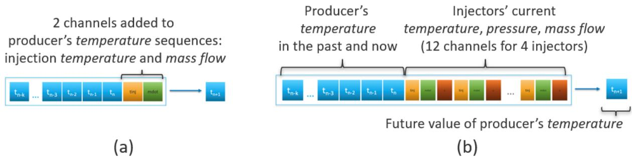
**Figure 2: Machine learning algorithms for time series prediction were developed for a simple single-fracture doublet system (a), and for BHS model with four active injector wells and six active production wells (b).**
