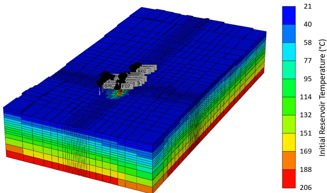
**Figure 1: CMG numerical reservoir model of Brady Hot Springs with initial temperature distribution. The model dimensions are approximately 18 km × 10 km × 3.5 km. Wells are concentrated near zone with elevated shallow temperature.**
