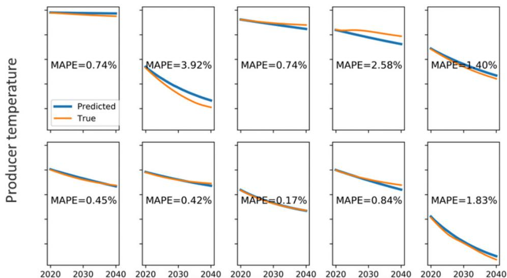
**Figure 5: Examples of temperature trajectories predicted from 2020–2040, for a BHS producer well. X-axis: time. Y-axis: selected producer well’s temperature (numbers are removed per industry partner requirements).**
