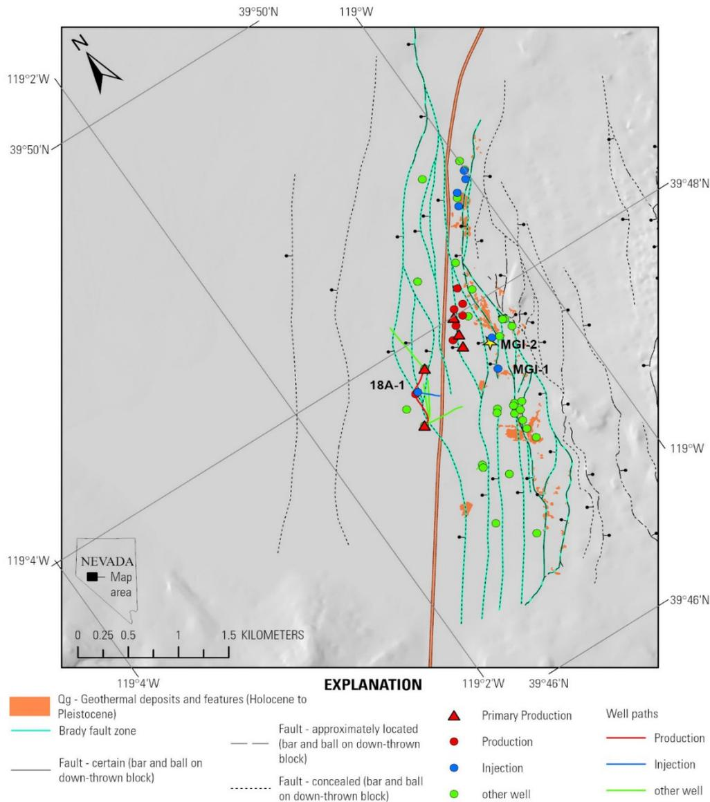
**Figure 9: Data gathering plan developed for Fiscal Year 21 includes temperature surveying of three idle wells (18A-1, MGI-1, and MGI-2), which look promising for future production.**
