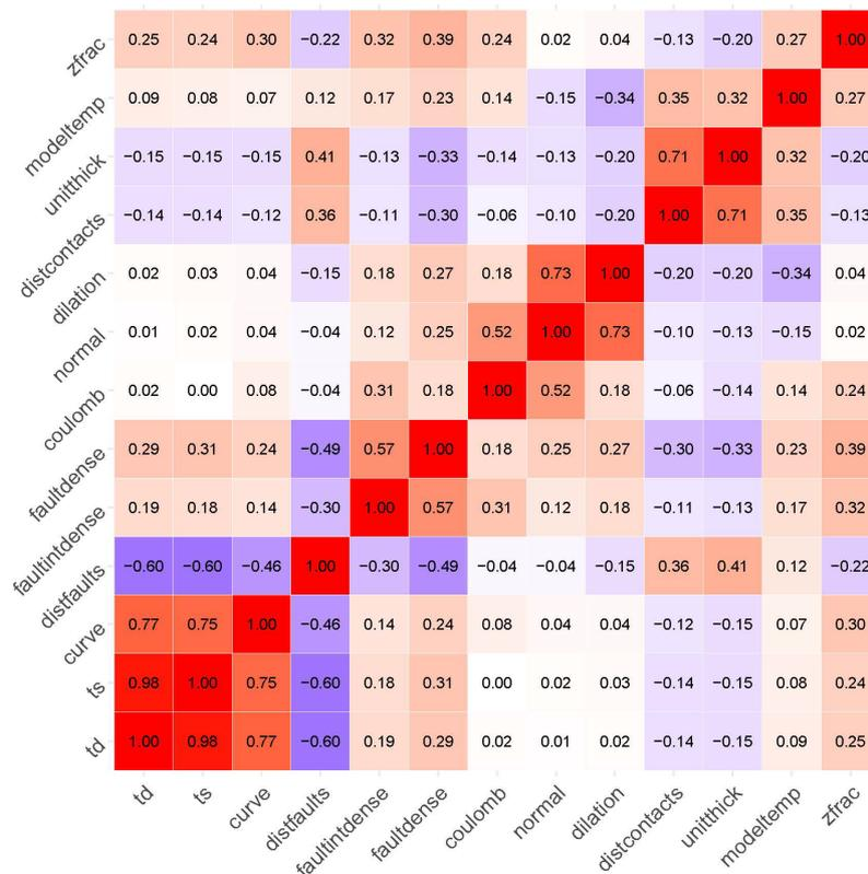
**Figure 7: Correlation heatmap between 13 geologic variables. Warm colors indicate high correlation between variables. Fracture permeability has highest correlation with fault density and fault intersection density.**
