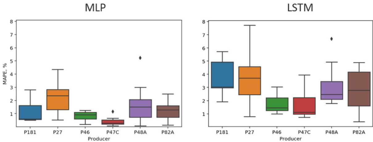
**Figure 6: MAPE values for prediction of temperatures of six production wells at BHS. Results are shown for the ten best-performing MLP and LSTM networks. The average MAPE for the MLP networks is on the order of 1%, while for the LSTM networks, it is around 2.5%.**
