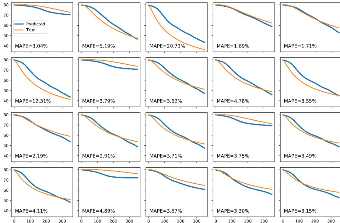
**Figure 3: Examples of the temperature trajectories predicted using LSTM networks for the single-fracture doublet system and MAPE values characterizing the accuracy of these predictions. X-axis: number of days since the beginning of learning and prediction. Y-axis: production well temperatures (in °C).**
