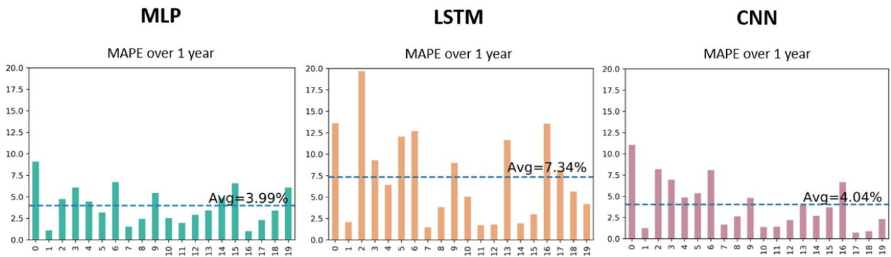
**Figure 4: MAPE values for temperature predictions in the single-fracture doublet system; evaluation results are shown for 3 network architectures being studied (MLP, LSTM, CNN). All these architectures produced accurate predictions, with 3.99%–7.34% relative errors (judged by the averaged MAPE values) between the predicted and true result in twenty scenarios. X-axis: test scenario’s number. Y-axis: MAPE (in %).**
