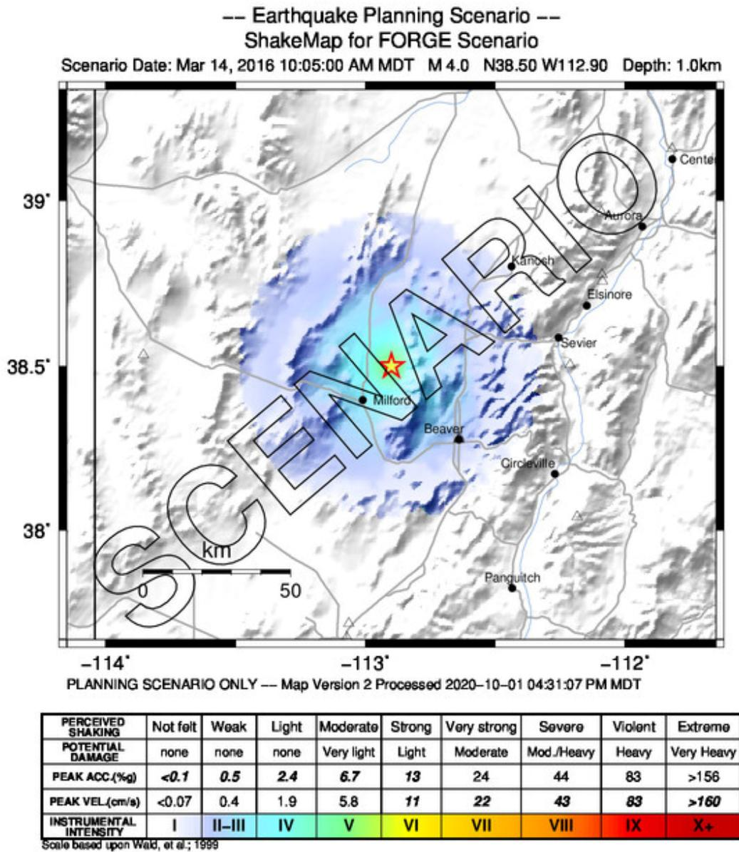
**Figure 23.** Deterministic intensity map for an induced scenario earthquake located near the Utah FORGE site (depth 1 km). Map was generated using ShakeMap (Wald et al., 1999; Worden and Wald, 2016). A point source is assumed because of the small magnitude.
