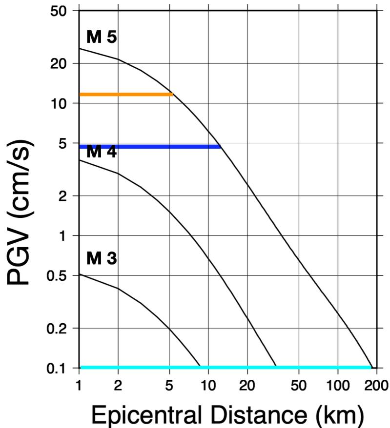
**Figure 12.** PGV curves (Chiou et al., 2010) for M 3, 4, and 5 earthquakes (depth 1km). Colored lines indicate threshold levels for felt (cyan), very light potential damage (blue), and moderate damage (orange) following Figure 10 (Worden et al., 2012).
