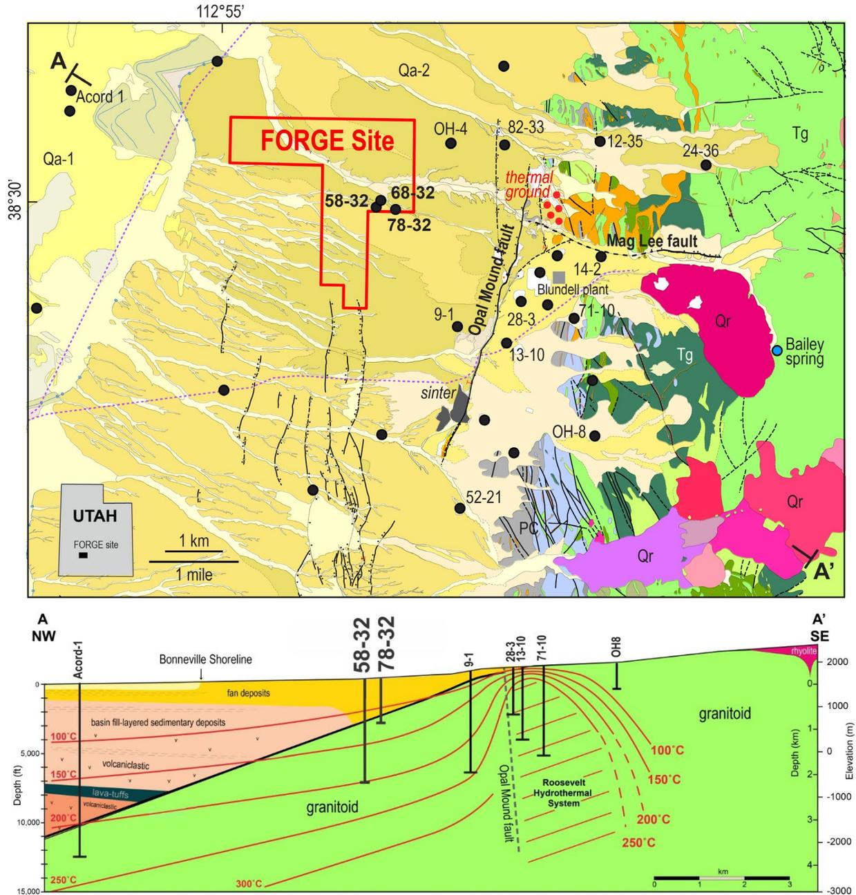
**Figure 20.** Geological map and cross-section for the Utah FORGE site. Shown are locations of mapped faults relative to the FORGE footprint and locations of earthquakes located with seismometers installed for the FORGE project (December 2016 through January 2018). Also shown on the cross-section are geotherms and location of nearby wells.
