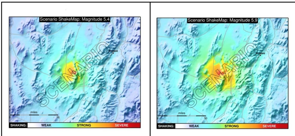
**Figure 22.** Deterministic intensity maps for two potential scenario earthquakes near the Utah FORGE site: Left, Opal Mound M 5.4 and right, Mag Lee M 5.9. Maps were generated using ShakeMap (Wald et al., 2005; Worden and Wald, 2016). Maximum magnitude (ground motions) based on fault dimension for the Opal Mound and Mag Lee scenarios (gray box surface projection of fault trace).
