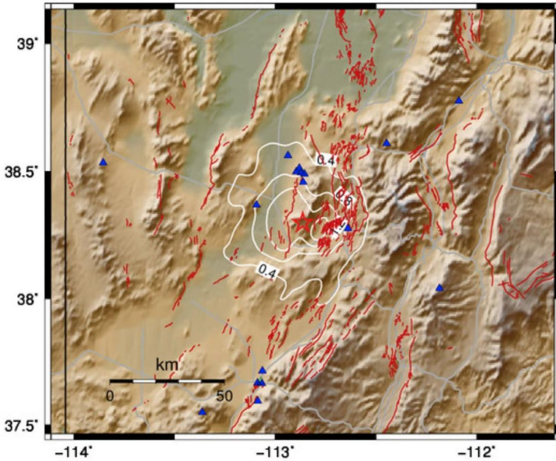
**Figure 15.** PGA contours (% g) generated by ShakeMap for the January 2020 M 3.9 earthquake located in the Mineral Mountains south of Milford (red star). Ground motion values are constrained by recordings at the nearby seismic stations. Red lines show the Quaternary faults. Blue triangles are seismic stations.
