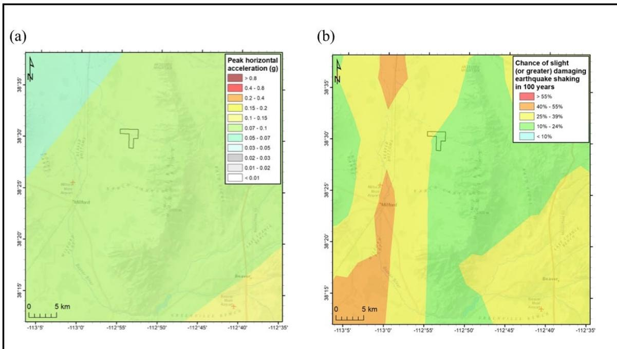
**Figure 2.** Probabilistic seismic hazard at the FORGE site from the 2018 National Seismic Hazard map (data from Rukstalis and Petersen, 2019). (a) 10% g in 50 yrs PGA hazard (475 yr return period). (b) Chance of slight to damaging ground motions in the next 100 years.
