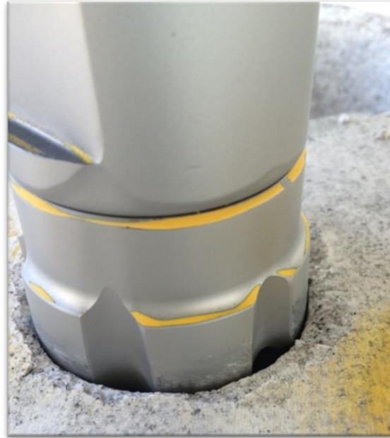
Figure 10: Percussive hammer bit engaged with rock.
