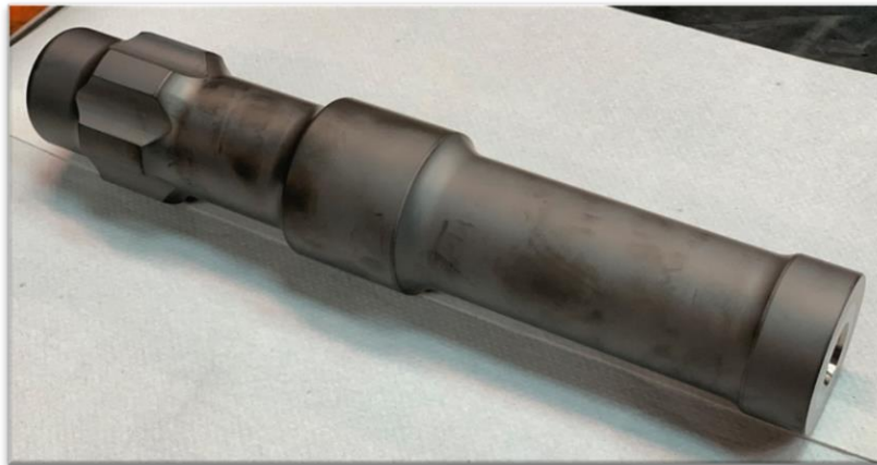
Figure 13: QLX 35 piston coated with DLC for solid lubrication.
