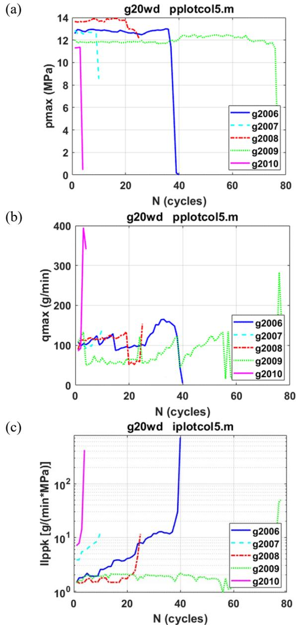
Figure 35 Fatigue responses as a function of number of cycles for G2 series: (a) maximum pressure, (b) maximum mass rate, and (c) pressure peak-based injectivity index
