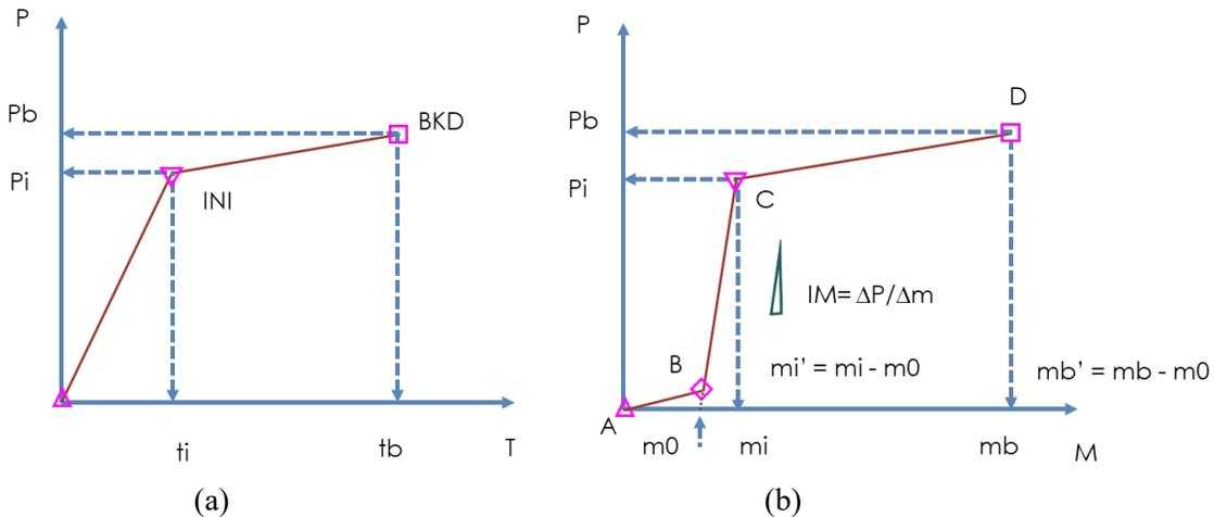
Figure 6 Diagrams showing pressure as a function of (a) time and (b) mass. Definitions of injection modulus, injection modulus ( $IM$ ) and filling amount identified,  $m_0$ ;  $P_i, m_i$  – pressure and injection mass at fracture initiation;  $P_b, m_b$  – pressure and injection
