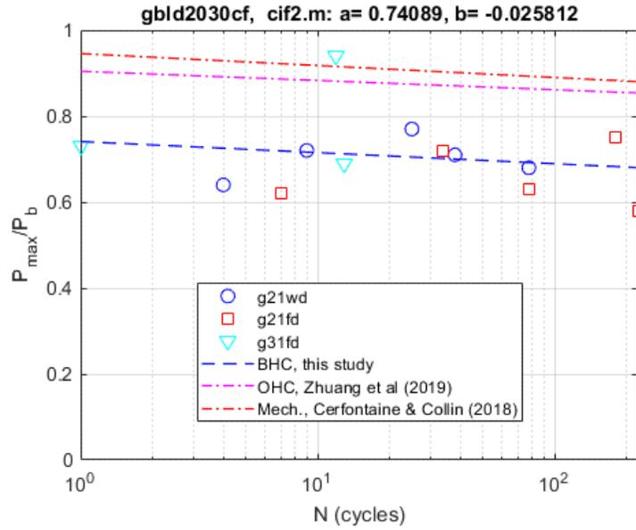
Figure 48 Ratios of maximum pressure in cycling to breakdown pressure in monotonic injection as a function of number of cycles to failure: (a)  $P_{max}/P_b$  and (b) fitting for pooled data using  $y = a + b \cdot \log_{10}(x)$ . g21wd – G2 series with water; g21fd – G2 series with foam; g31fd – G3 series with foam; BHC – blind hole cylinder; OHC – open hole cylinder, Mech. – mechanical fatigue.
