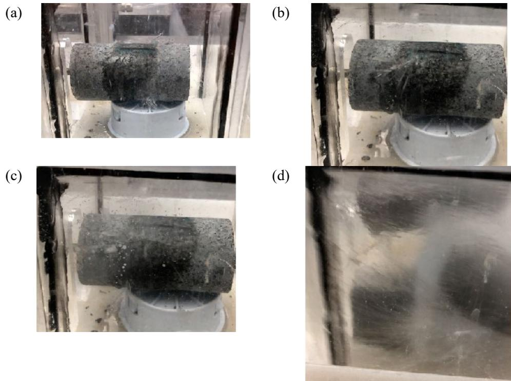
*Figure 38 Video-based cyclic injection responses of g2015 with foam as fracturing fluid for events (a) #1: 28.90 s fracture initiated with foam leaking, (b) #4: 132.31 s mixture injection, (c) #5: 132.35 s increased ejection, (d) #6: 132.40 s breakup.*
