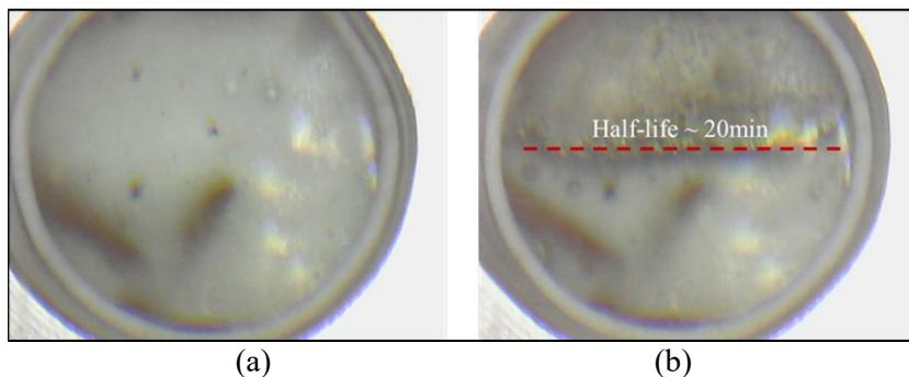
Figure 58 AOS + Crosslinker foams at 200°C and 1000 psi condition. The two images represent foam (a) after injection, (b) at 50% height.
