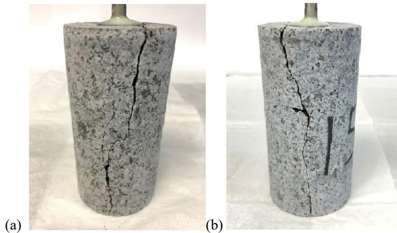
Figure 39 (a) and (b) Post-test images of g2015 induced by cyclic injection in two orientations showing axial fractures with secondary transverse fracture.
