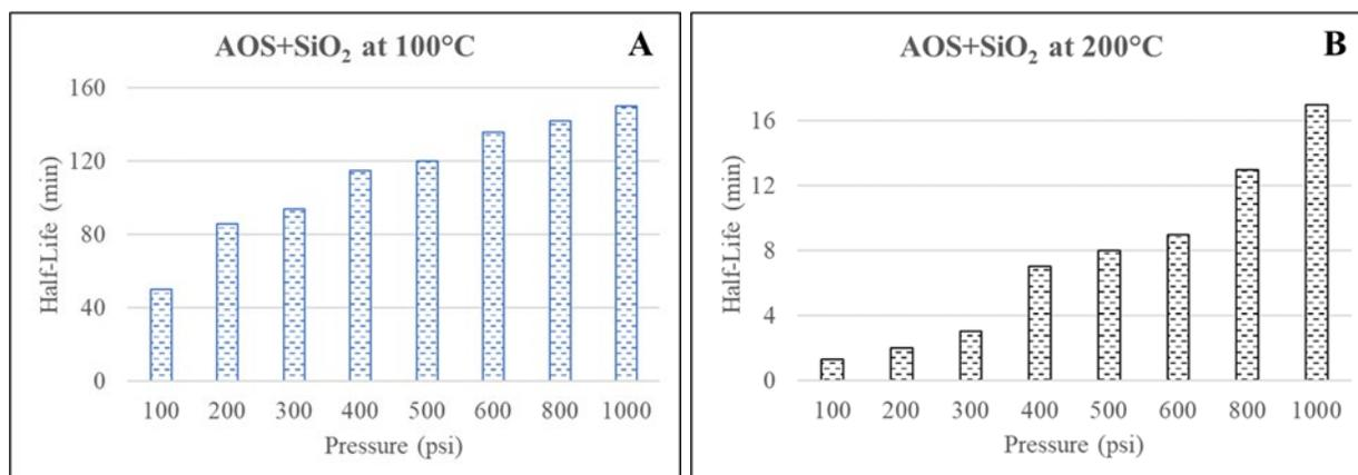
Figure 64 Thermal stability of AOS + SiO<sub>2</sub> foams at (A)100°C and (B) 200°C.
