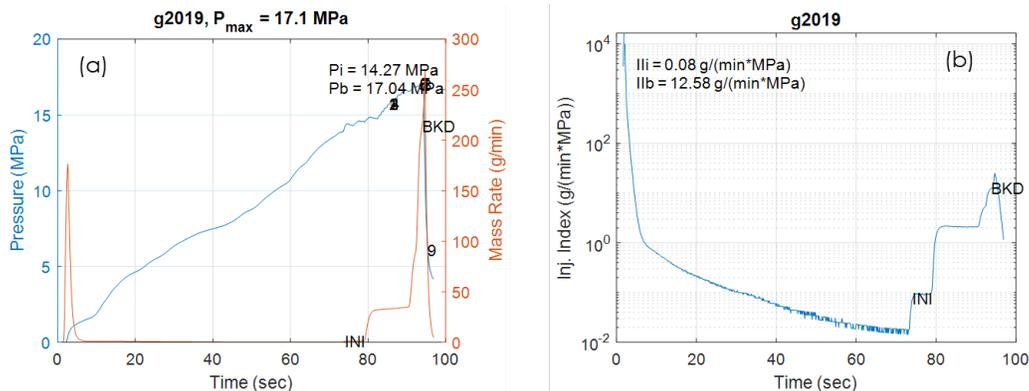
Figure 7 Responses as a function of time for g2019: (a) pressure & mass rate, (b) injectivity index. INI – fracture initiation, BKD – breakdown; same comments apply in the following.
