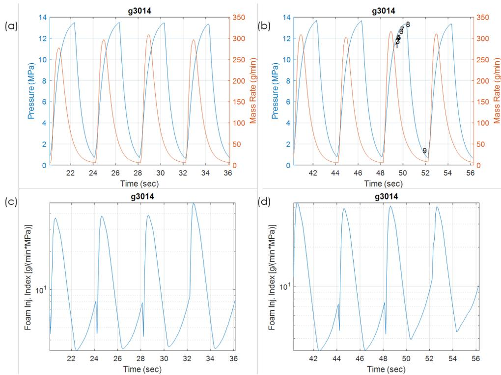
Figure 41 Responses as a function of time for g3014: pressure and mass rate in (a) middle life and (b) final cycles, and instantaneous injectivity index in (c) middle life and (d) final cycles.
