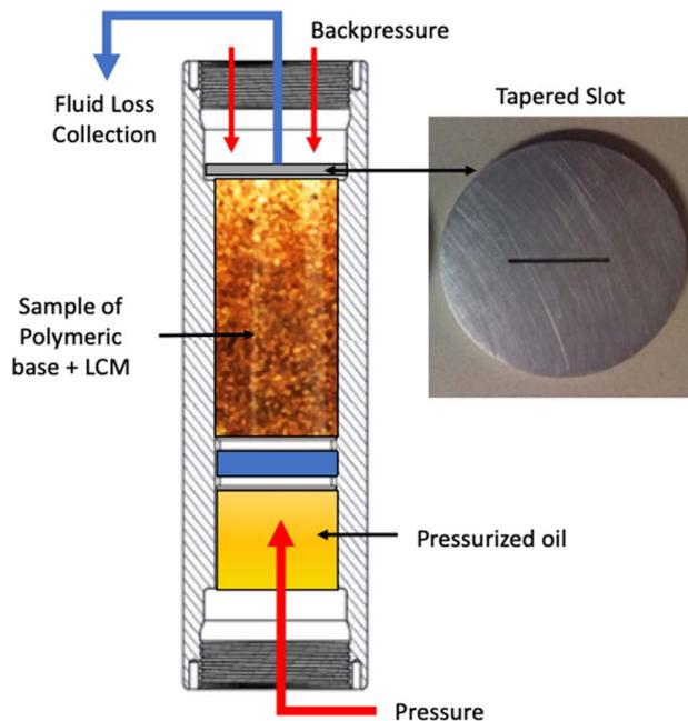
**Fig. 5 Diagram of the pressure cell of the PPT apparatus for LCM filtration screening**
