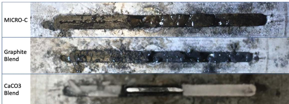
Fig. 9 Close-up view of 1000  $\mu\text{m}$  fracture once the disk was removed from the pressure cell
