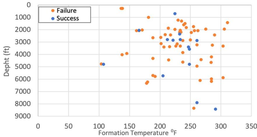
**Fig. 1 LCM treatments effectiveness from temperature versus depth perspective (plot generated with information adapted from Cole et al. [8])**
