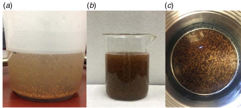
**Fig. 6 Walnut fine mixed with free of solids mud: (a) walnut settling in mud non-thermally activated, (b) walnut evenly distributed in thermally activated mud, and (c) top of the PPT pressure cell filled with mud + LCM**
