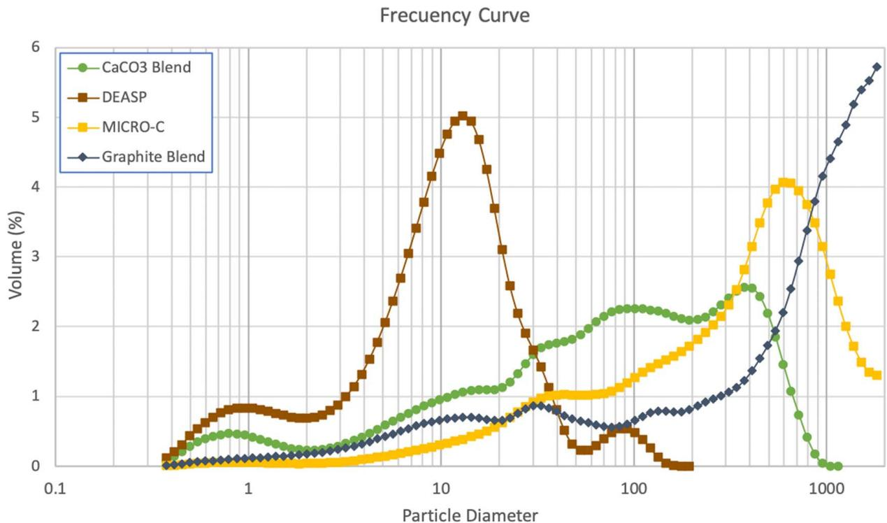
**Fig. 11 Frequency curve of particle diameter test on different fine granular LCMs**
