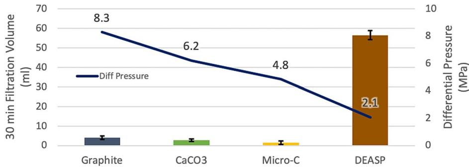
Fig. 12 Filtration and differential pressure results of fine granular LCMs tested
