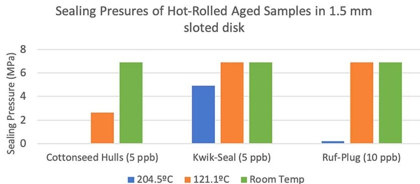
**Fig. 3 Sealing pressures of three cellulosic LCM products at different temperatures (plot generated with information adapted from Hinkebein et al. [1])**
