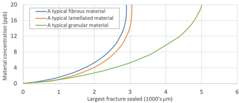
**Fig. 2 Effect of LCM concentration at different fracture sizes (modified from Howard and Scott [19])**
