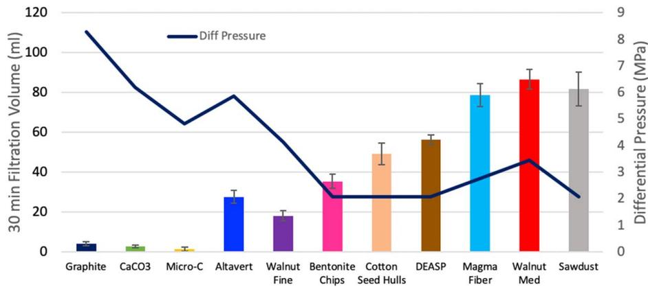
Fig. 8 Filtration volume and maximum sealing pressure obtained of different LCMs
