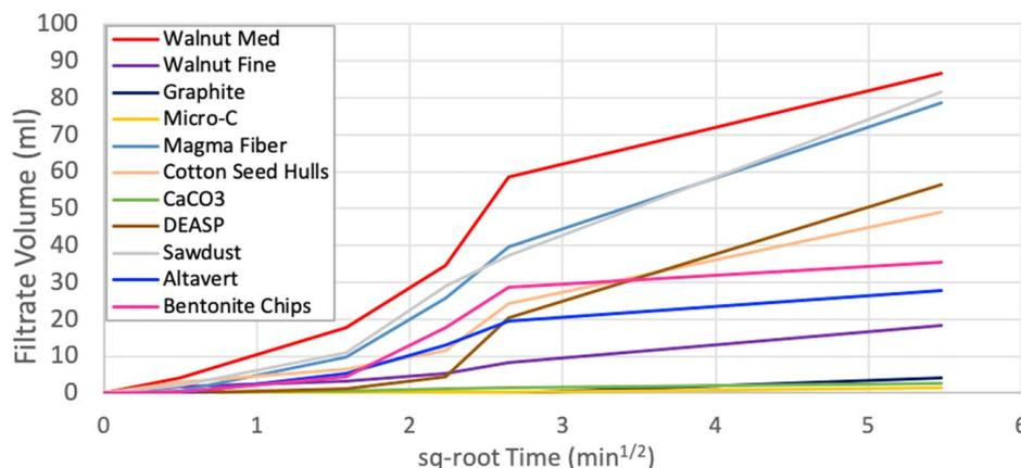
**Fig. 7 Filtration results of individual tests of the free of solids mud + LCMs**
