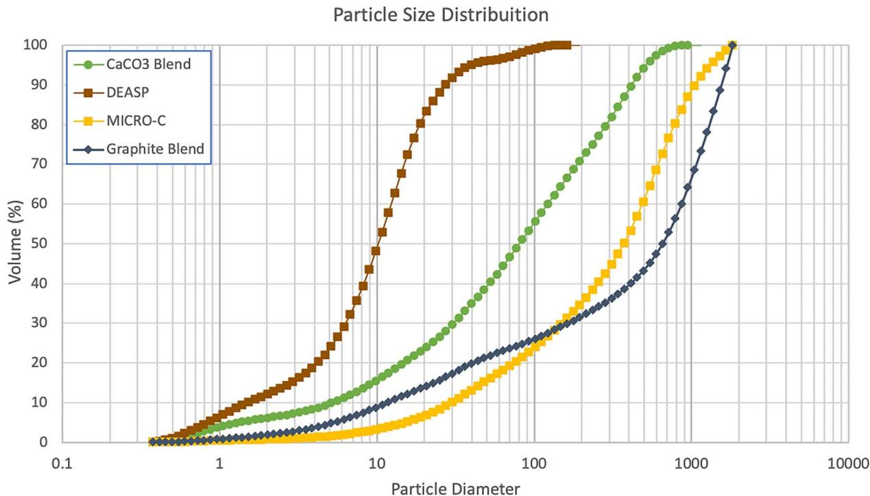
**Fig. 10 PSD test on different fine granular LCMs**
