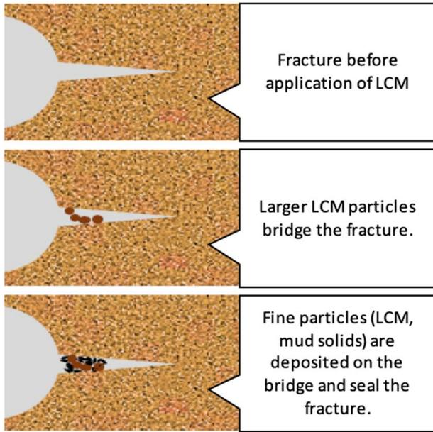
**Fig. 4 LCM bridging and sealing process (adapted from Lavrov [20])**
