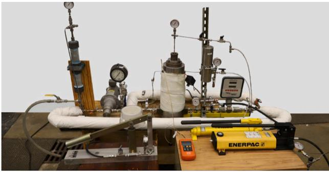
Fig. 5. Photo of the high temperature dynamic LCM testing setup.
