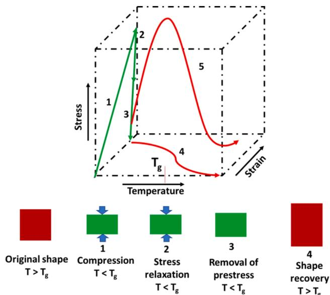
Fig. 2. Cold-Programming of thermoset SMPs (Modified after Li, 2014).
