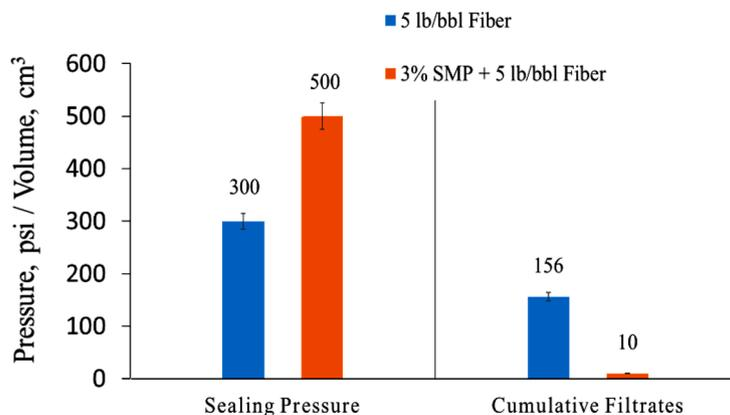
Fig. 13. Sealing pressure and filtrates volume from dynamic LCM testing for fiber and SMP/fiber blend.
