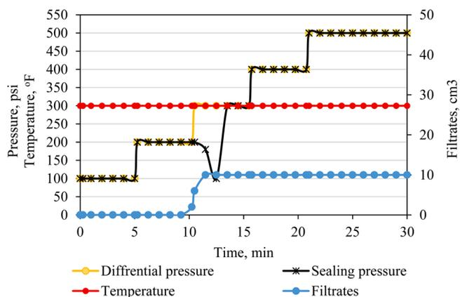
Fig. 12. Dynamic LCM testing with 3 wt.% SMP mixed with 5 lb/bbl fiber at 300oF.
