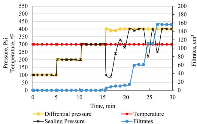
Fig. 11. Dynamic LCM testing with 5 lb/bbl fiber at 300oF.
