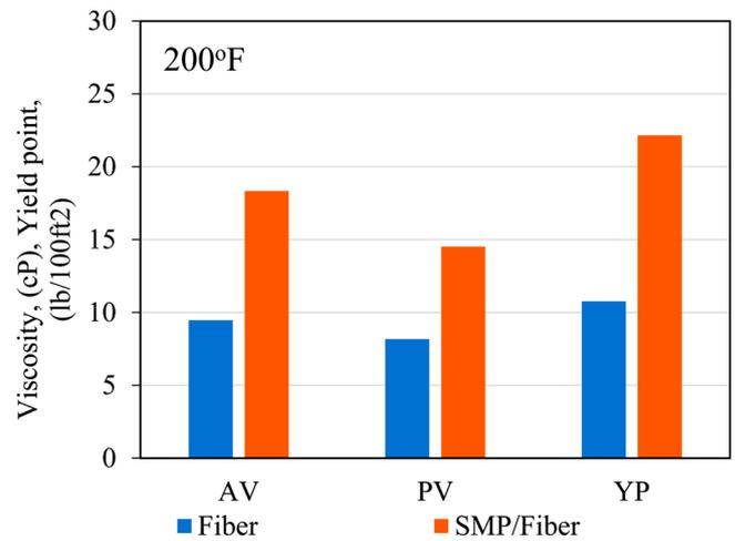
Fig. 7. Rheology result for the 5 lb/bbl fiber and 3 wt.% SMP plus 5 lb/bbl Fiber.
