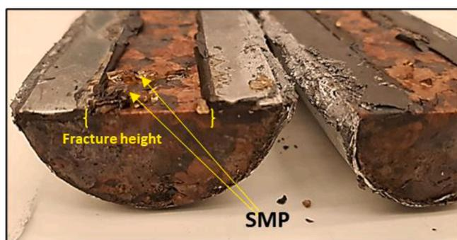
Fig. 14. Split core after the dynamic LCM testing with SMP/fiber blend.
