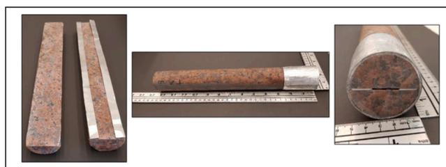
Fig. 4. Core with 2" OD x13.5" length core split into two halves (left), welded core with fracture length: 13.5" (middle), and top view of fracture width 1000  $\mu\text{m}$  (right).
