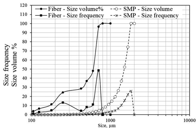
Fig. 8. Size volume % and frequency of the fiber and SMP from the particle size analysis.
