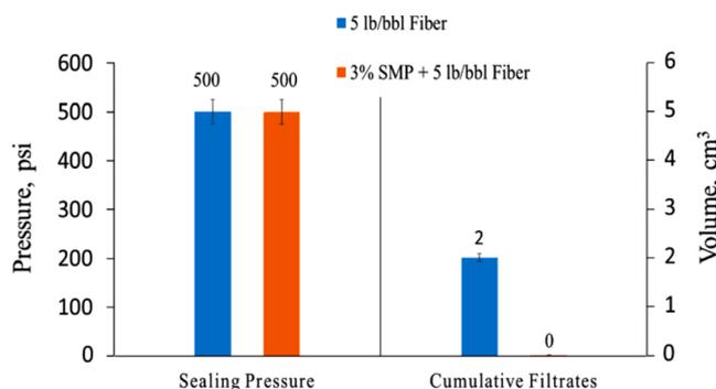
Fig. 9. Sealing pressure and cumulative 30 min filtrates volume of the PPT for SMP and fiber.
