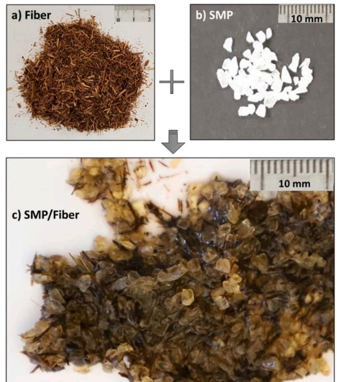
Fig. 3. Photos of a) Cedar fiber, b) SMP, and c) SMP/Fiber mixture after a fracture sealing test.
