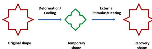
Fig. 1. Deformation and shape recovery of shape memory materials.
