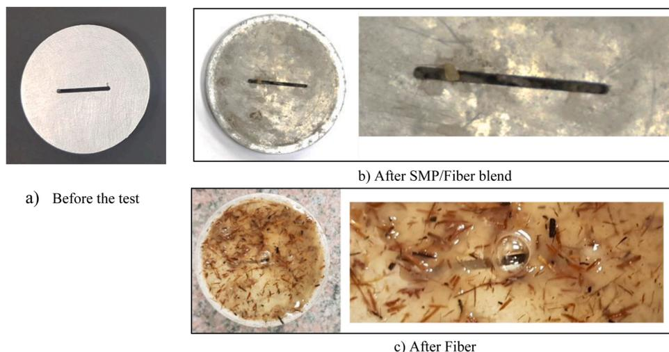
Fig. 10. Aluminum disc, a) before and after PPT, tested with b) SMP/Fiber blend and with c) Fiber.
