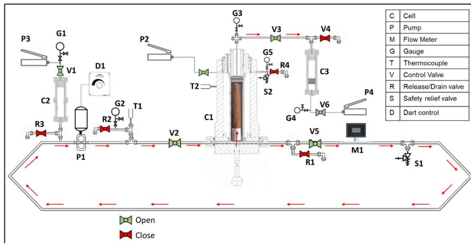
Fig. 6. Sketch of the high temperature dynamic LCM testing unite, and a 2 × 13.5" core inserted in the confined cell.
