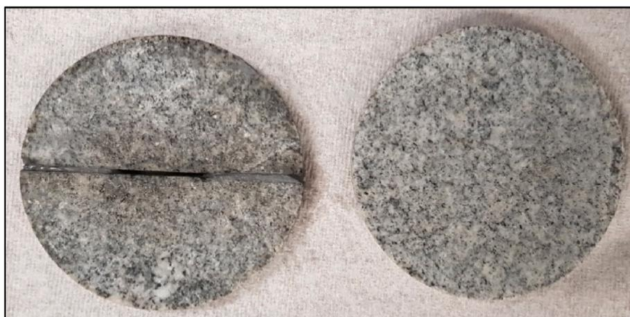
Fig. 5. (Right) Granite disk, 2.5" Di x 0.25" thickness, (Left) Same disk with a fracture of 1" length x 1000 μm width.
