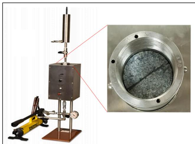
Fig. 2. Static filtration experimental setup, PPA with the fractured disk.
