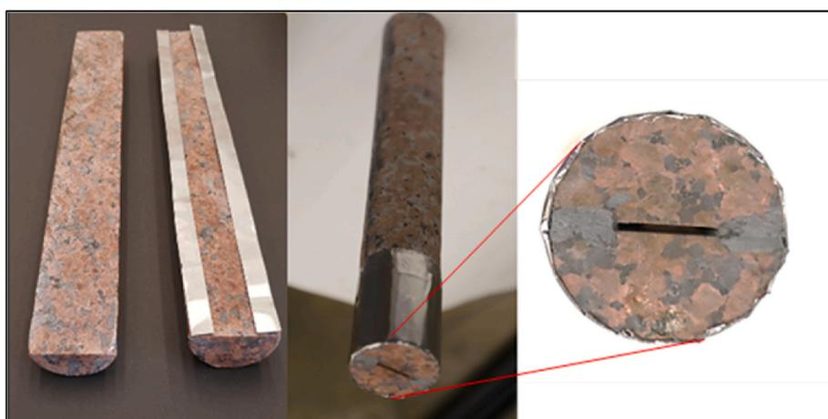
Fig. 6. A core with O.D. of 2.5 in and length of 13.5 in with longitudinal and cross-sectional views of the fracture with the width of 1000 μm.
