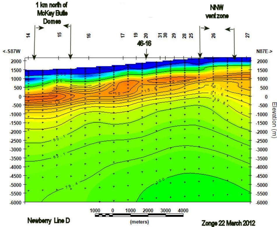
Figure 9: 2-D MT slice Line D. The two digit numbers across the top identify MT stations.
