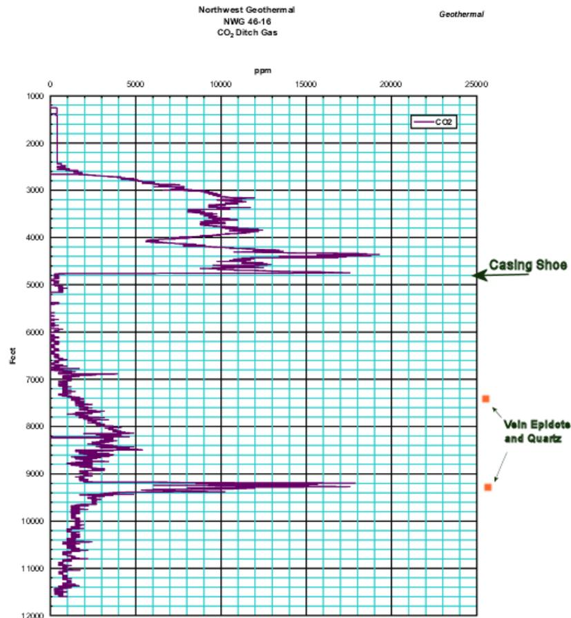
*Figure 3: A graph showing CO<sub>2</sub> values measured by Epoch Mudlogging during drilling of well 46-16. To the right are noted the depth of the casing shoe and the location of hydrothermally precipitated druse quartz and epidote observed in the drill cuttings.*
