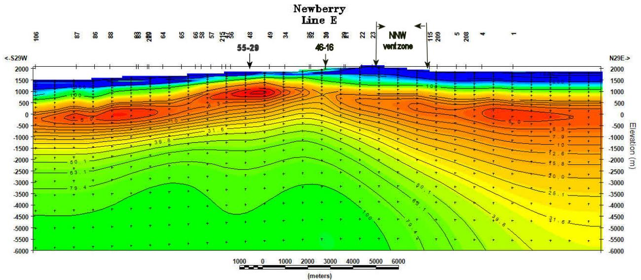
Figure 10: 2-D MT slice Line E. The one, two and three digit numbers across the top identify MT stations.
