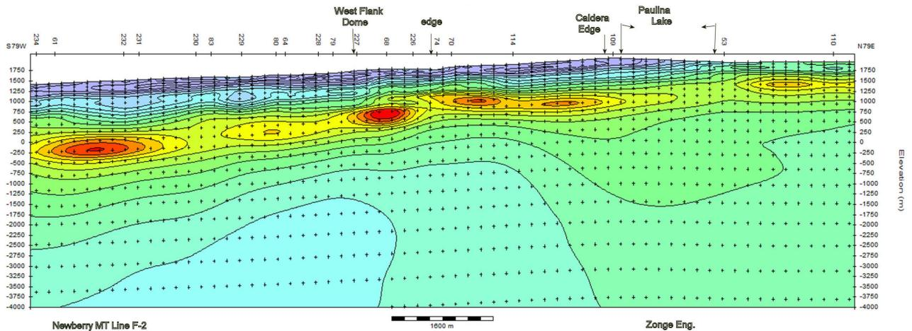
Figure 11: 2-D MT slice Line F. The two and three digit numbers across the top identify MT stations.
