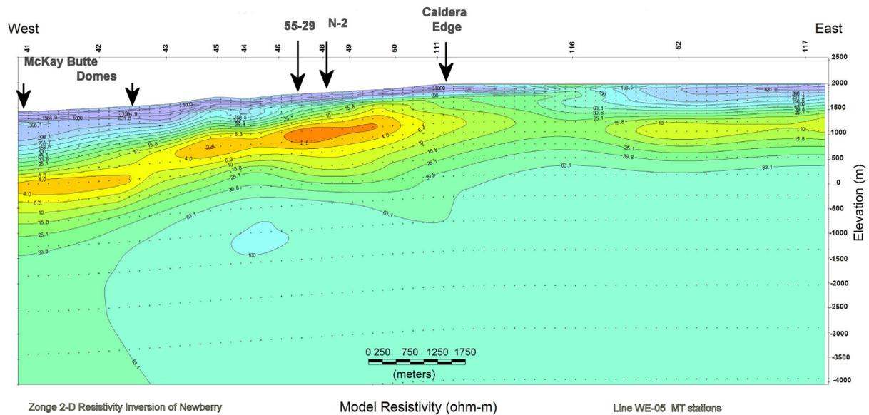
Figure 12: 2-D slice Line 05. The two and three digit numbers across the top identify MT stations.
