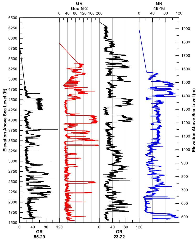
Figure 6: Gamma logs of the upper 4,000 ft. of wells 55029, N-2, 23-22 and 46-16 on the northwest flank of Newberry Volcano. These sections of the wells show details of the gamma logs penetrating into the shallow electrically conductive layer.
