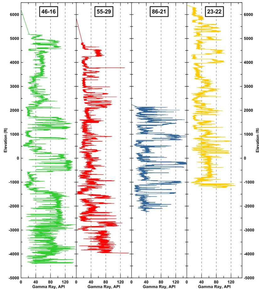
*Figure 5: Gamma logs of each of the four deep exploration wells drilled on the northwest flank of Newberry Volcano.*
