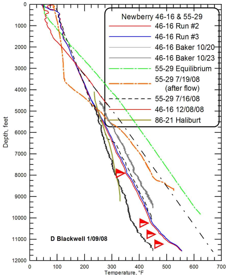
Figure 4: Temperature plots of deep exploration wells 46-16, 55-29 and 86-21. The red arrows are locations where Dr. D.D. Blackwell observed evidence in the temperature profiles of formation fluid flow.
