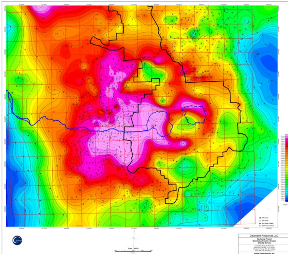
Figure 7: Complete Bouguer Anomaly with a density reduction value of 2.5 g/cc.
