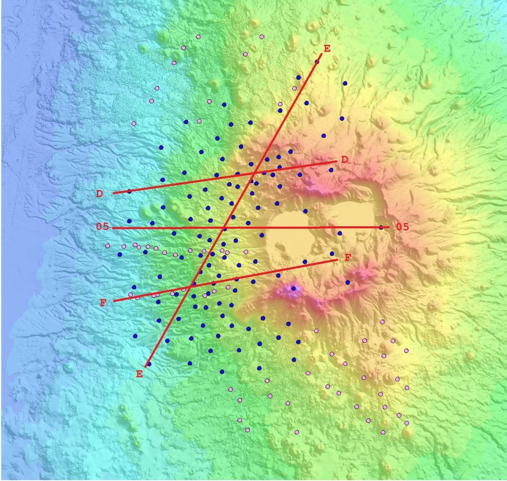
*Figure 8: Map of Newberry Volcano showing MT station locations. The red lines show the location of four MT slices of Figures 9, 10, 11, and 12. The blue dots identify MT station locations from the 2007 survey. The red dots identify MT station locations from the 2011 survey*
