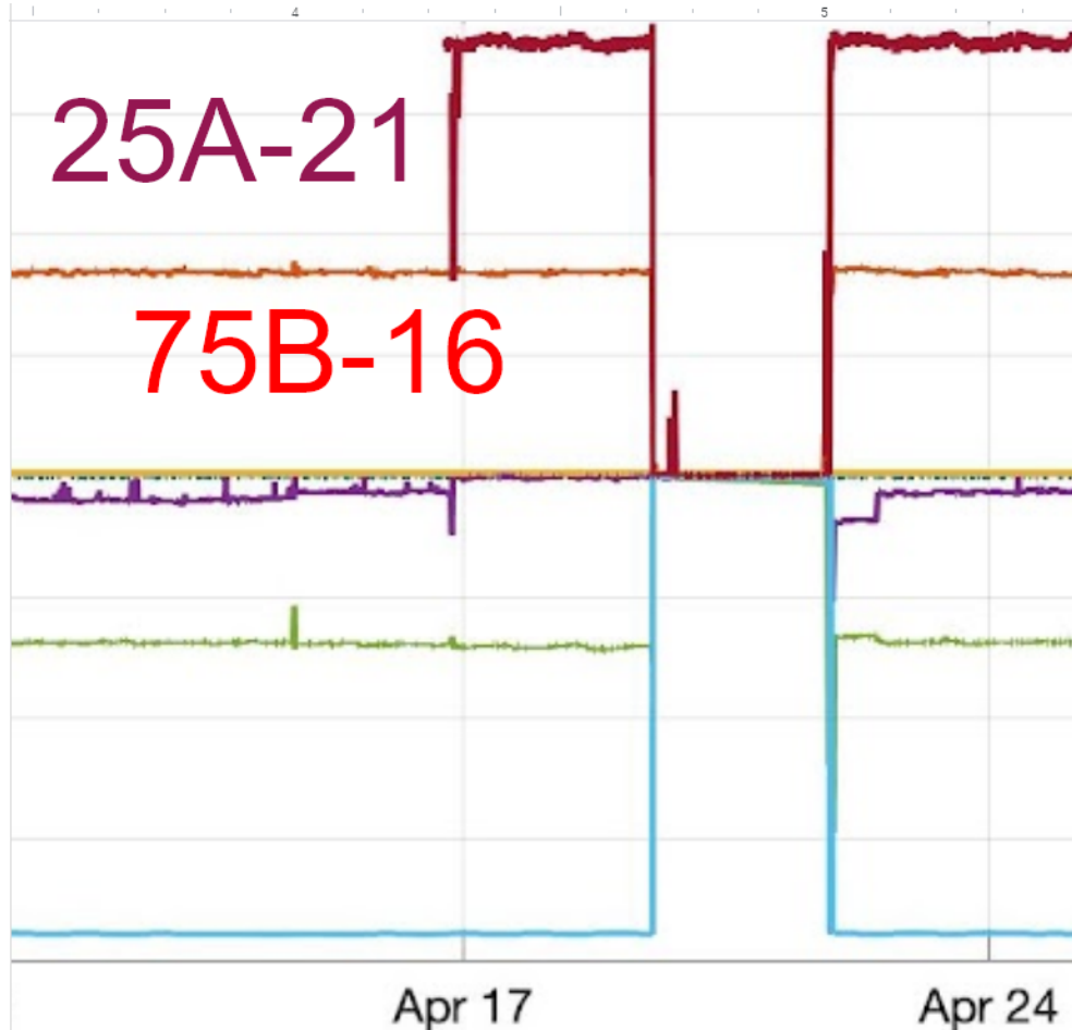
Figure 7. Plot showing the pumping rates at production and injection wells near the times of the start of the planned shutdown and gradual resumption of pumping.
