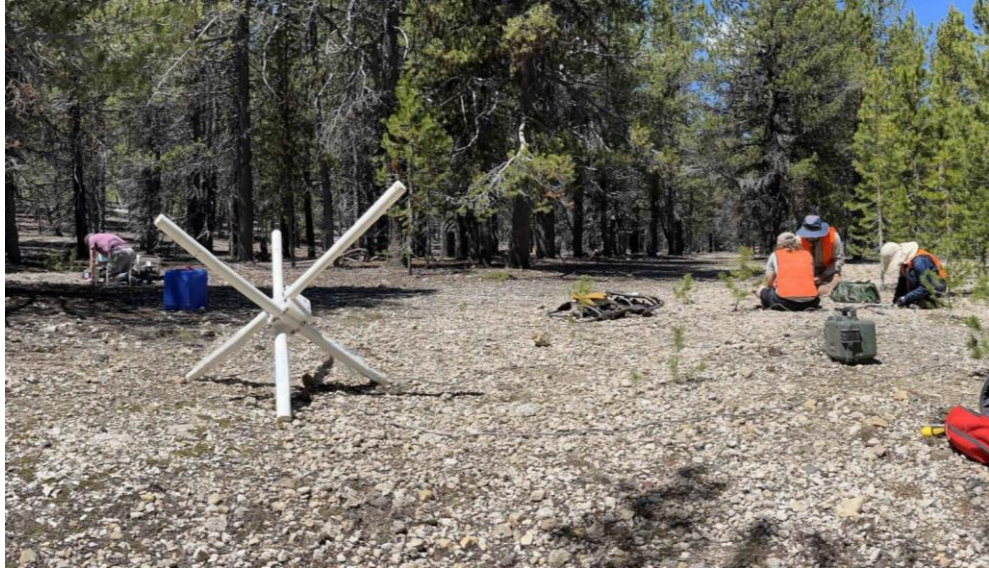
Figure 5. Three wideband induction coil sensors (white tubes approx. 40-in long) are clamped together and placed on the ground as seen on the left-hand side of the photo. A data acquisition system is located ~5m away (shown here surrounded by crew members on the right-hand side of the photo), powered by a lithium polymer battery pack (green Pelican™-style case) shown in the right foreground. A gravity reading is being taken in the left background of the photo.
