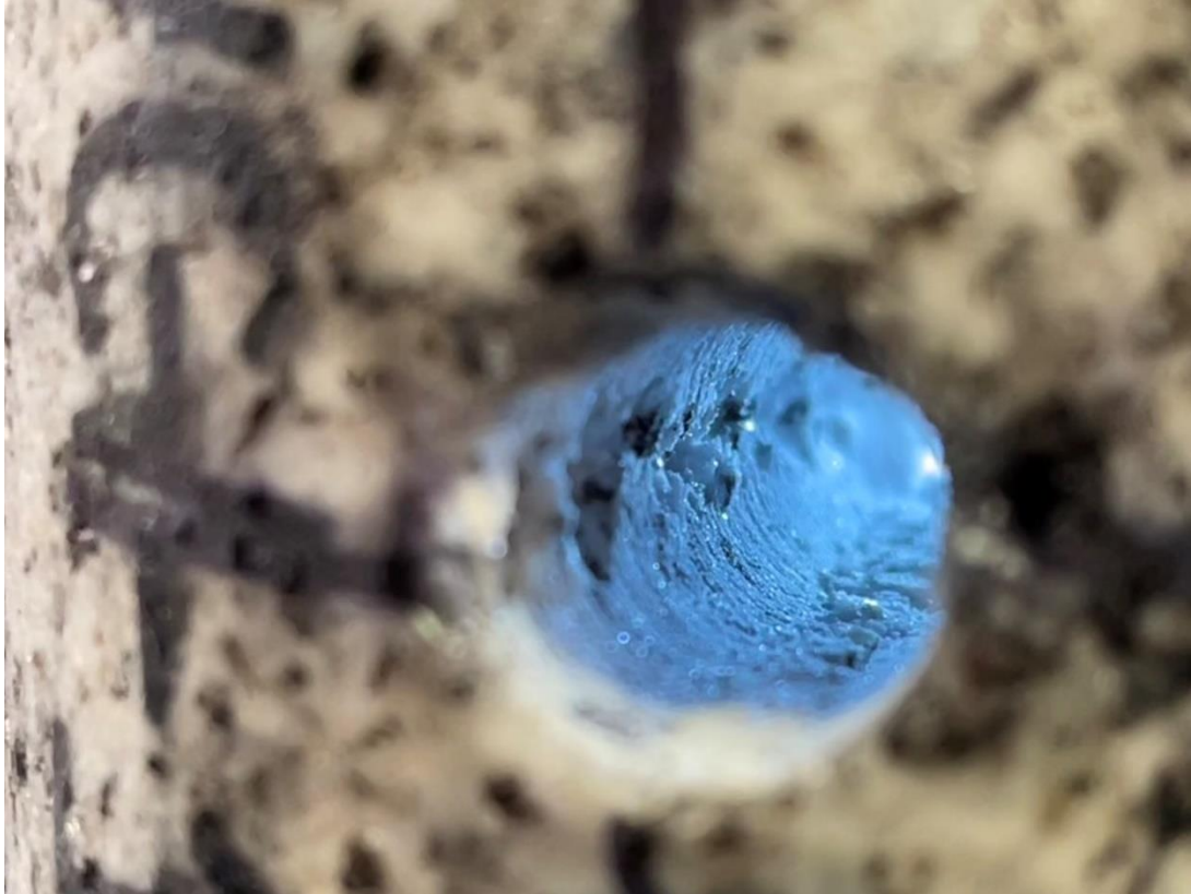
Figure 10. Borehole of sample SWG-01 after deformation. Fracturing occurs along the horizontal plane of the borehole.
