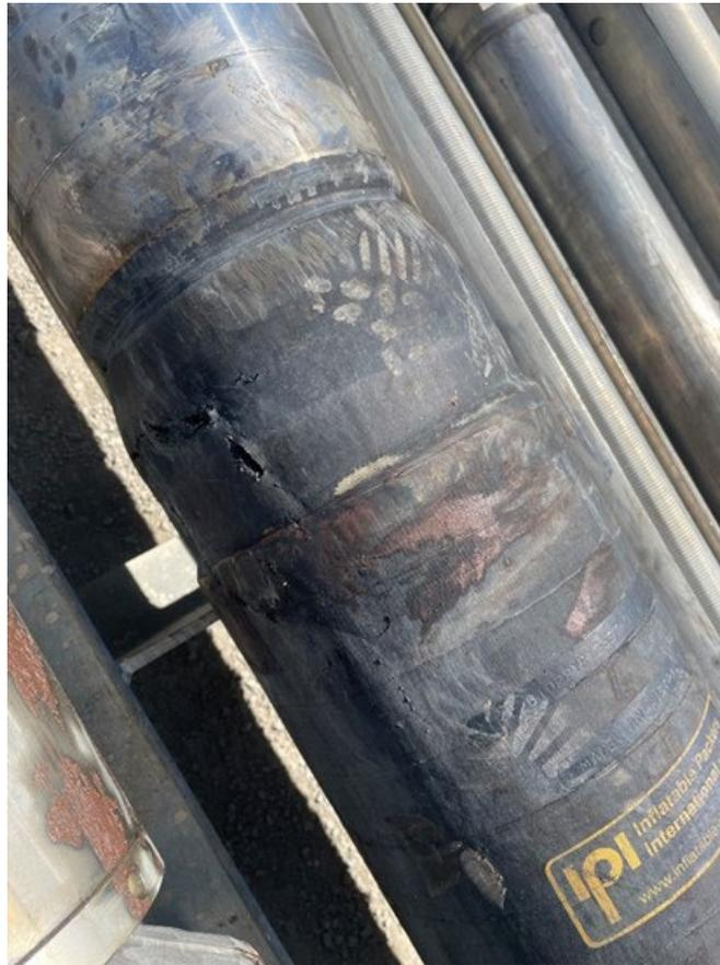
**Figure A-9. Punctures in the straddle packer tool prevented effective pressure buildup during later tests.**
