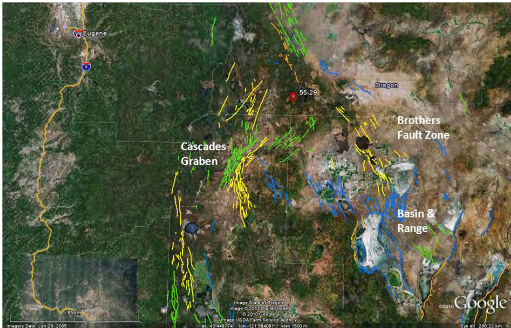
Figure 2-3. Regional structure map showing location of the Newberry EGS Demonstration, indicated by the EGS injection well NWG 55-29. Newberry Volcano lies at the intersection of three structural trends in central Oregon (see Figure 2-1 for geographic reference). Colored lines are faults from the USGS Quaternary fold and fault database. The fault ages are coded by color, from oldest to youngest: blue, younger than 1.6 million years; green, younger than 750000 years; yellow, younger than 130000 years; and orange, younger than 15000 years.
