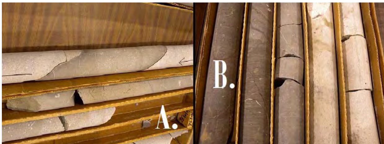
Figure 3-8. Drill core from the University of Utah core library showing that lithologic changes can be both abrupt (A), as with a dike (from well 72-3 at 1363 m (4469 ft), or gradual (B), as with hydrothermal bleaching (from GEO N-2 corehole at 1101-1104 m [3610-3620 ft]). Cores are approximately 7.6 cm (3 in) in diameter.
