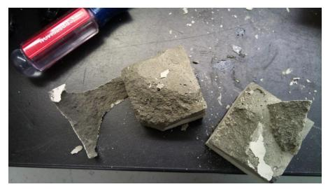
Figure 1 Damaged Ferrierite samples while de-molding
