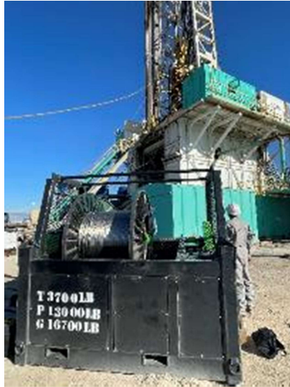
Figure 13. Spooler with Fiber Optic Cable.
