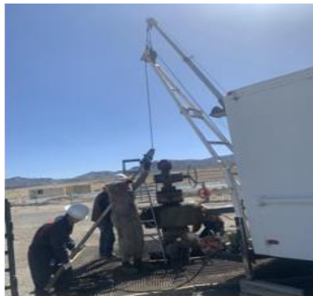
Figure 7 Deploying the transmitter tool into Bread Truck at well 16A-78(32)
