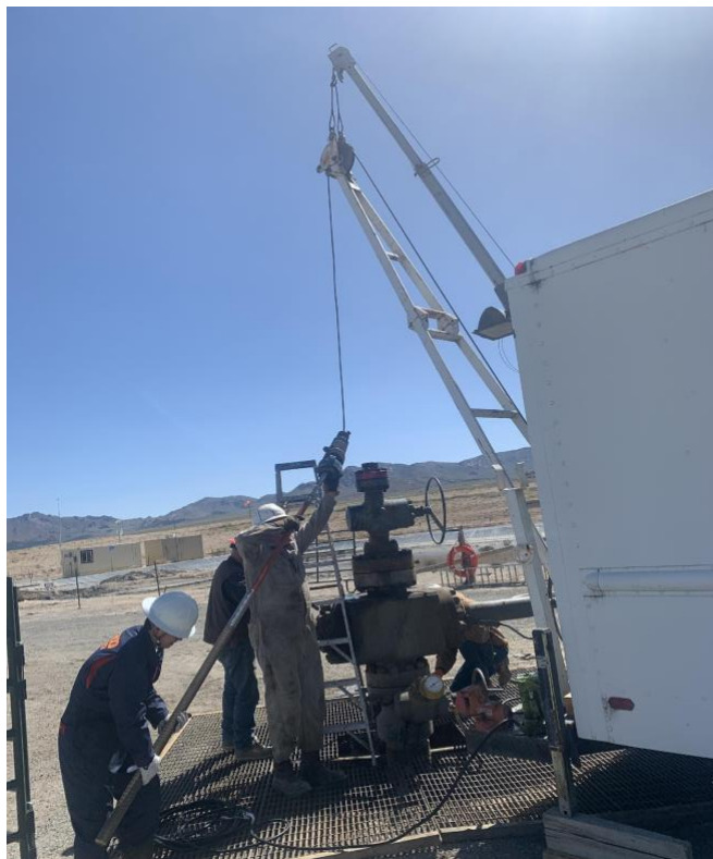
Figure 7 Deploying the transmitter tool into Bread Truck at well 16A-78(32)
