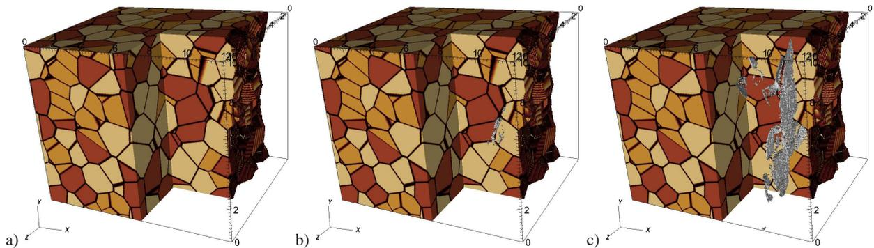
Figure 3: Fracture initiation and propagation in a three-dimensional grain-scale simulation. a) Cutaway of the grain microstructure: light colored grains are quartz; orange grains are k-spar; brown grains are plagioclase. The rock face is heated by fluid in the space on the right of the image. b) Fractures (gray planes in the cutaway section) tend to initiate at inter-grain boundaries, c) but propagate along the thermal front, following the principal compressive stresses.
