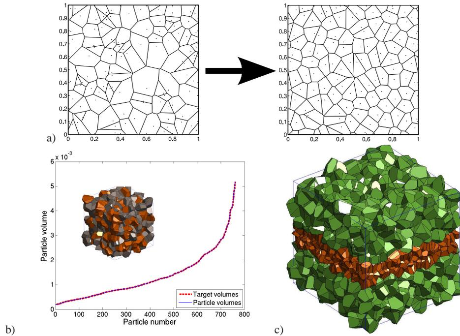
Figure 2: Examples of Voroni-cell based microstructures: a) Microstructures are generated from a random set of points, which are then perturbed over a series of iterations to fit a pre-determined particle size distribution, shown here for a two dimensional assembly; b) Target (dashed red line) and generated (solid blue line) particle-size volume for a three dimensional assembly (inset figure); and c) A layered three dimensional assembly.
