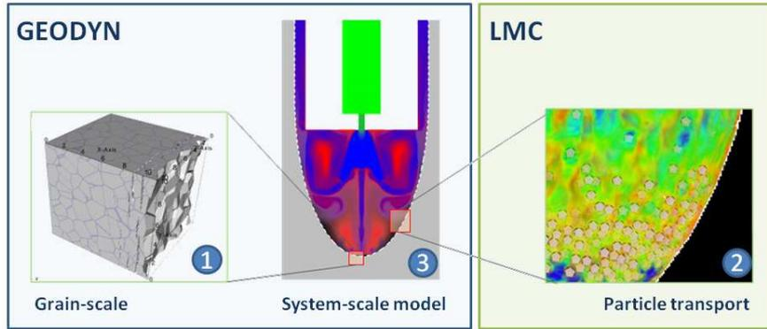
Figure 1: Illustration of the three models outlined in this paper: 1) a high-resolution model capturing the grain-scale failure of granitic materials; 2) a particulate-fluids model for spall transport simulations; and 3) a system-scale model to simulate the borehole behavior. The grain-scale and system-scale models are both simulated with the GEODYN modeling framework, while particle transport is simulated with the Low Mach Code (LMC).
