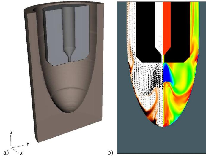
Figure 5: Axisymmetric GEODYN borehole-scale model: a) problem geometry showing a cross-sectional view of the borehole geometry (brown) and drill-bit head (grey); b) spall volume fraction and fluid velocities (left) and fluid temperature (right).
