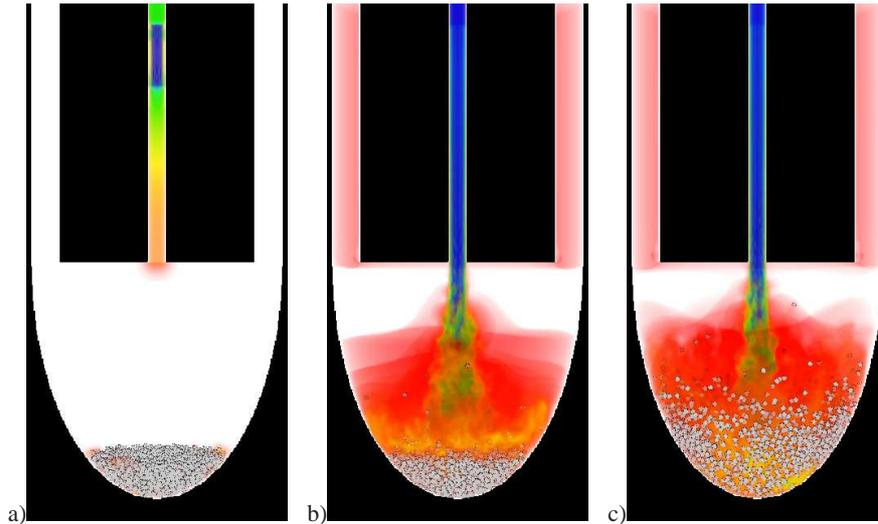
Figure 4: Three-dimensional LMC simulation of spall transport: a) Initial particle setup, b) vertical fluid velocities and particle locations at 0.01 seconds, and c) at 0.02 seconds, when all particles have been entrained in the flow. Two dimensional cross-sections of the borehole geometry and drill head are shown in black.
