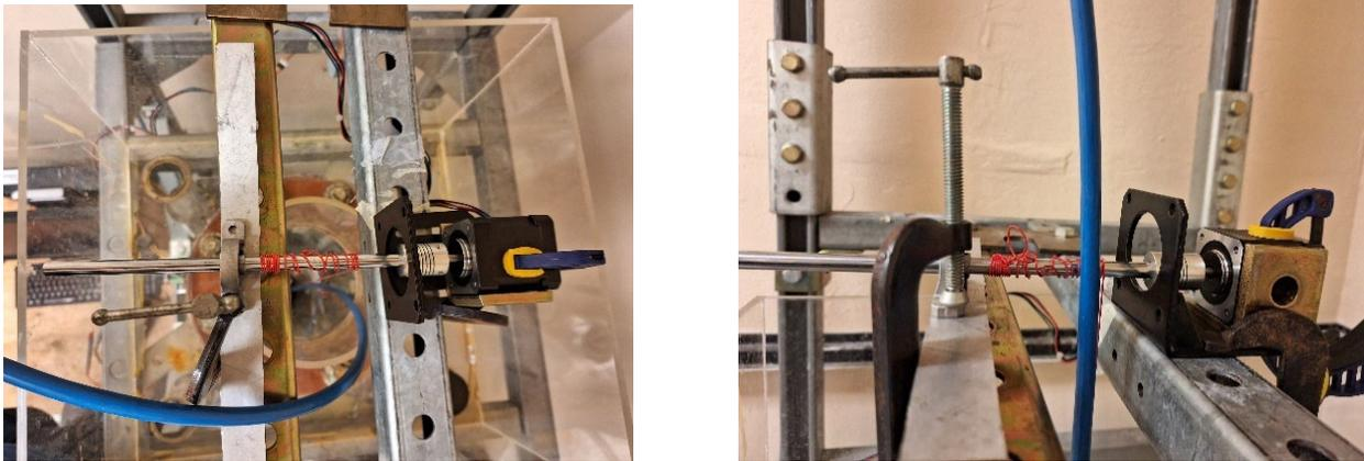
**Figure 4-19:** Stepper motor, wire, and rod configuration at the top of wellbore.
