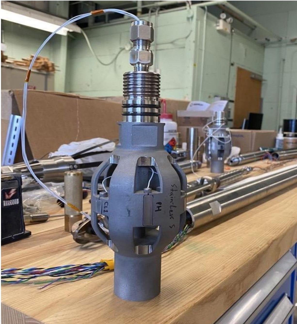
**Figure 2-25:** Fabricated sensor housing populated with installed sensors and bulkhead fitting.
