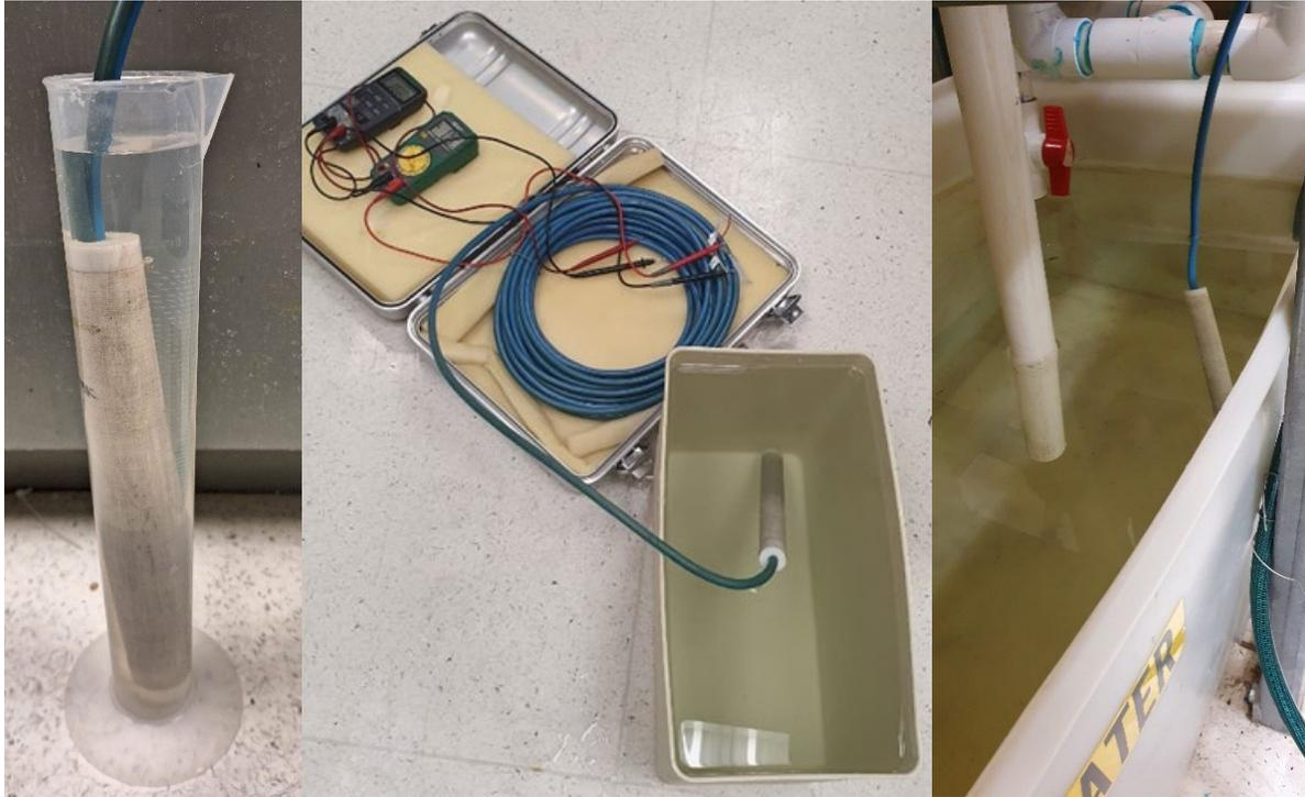
**Figure 4-5:** Tool calibration container: 400 ml (left), 20 L (center), and 100 L(right).
