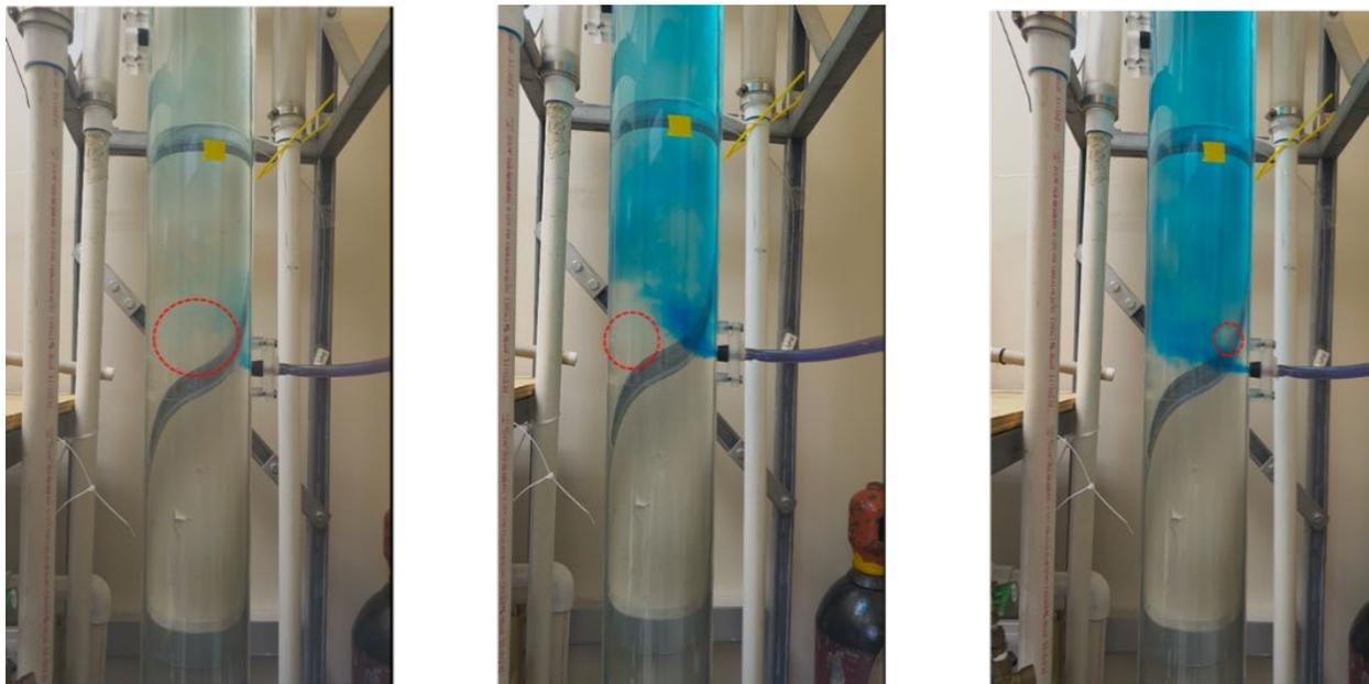
**Figure 4-18:** Dye injection tracer test (left) 20 ml/s, (center) 50 ml/s, (right) 70 ml/s.
