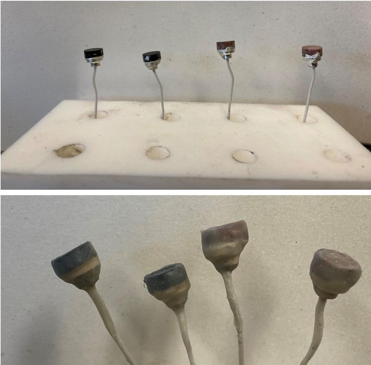
**Figure 2-7:** ISE and reference sensor assemblies before (top) and after (bottom) application of Gagekote.
