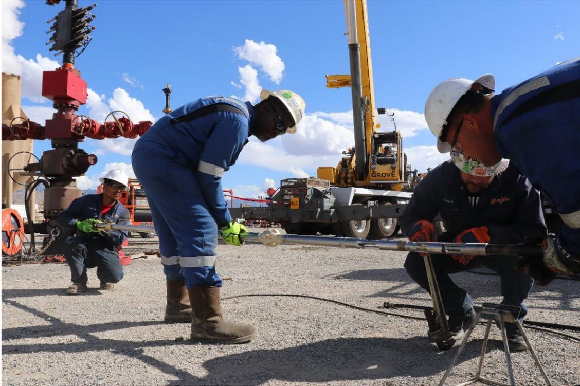
**Figure 5-9:** Full chemical tool assembly attached to weight bars and being loaded into lubricators.
