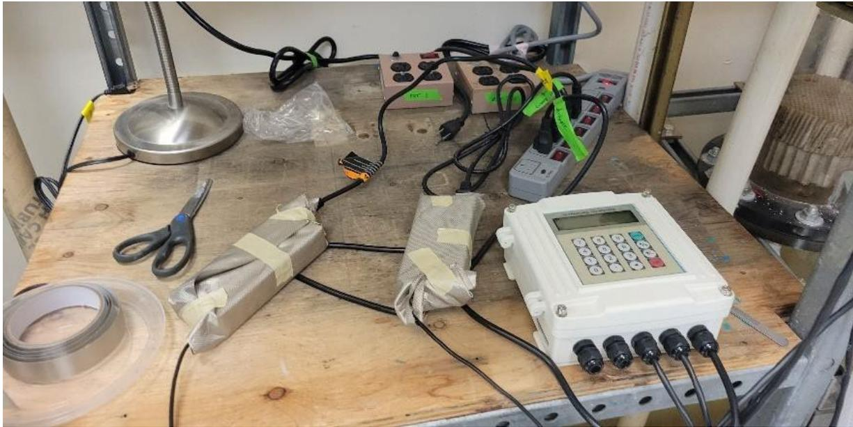
**Figure 4-63:** Faraday mesh applied to the power supply transformers of the submersible pumps in the Stanford Geothermal Laboratory
