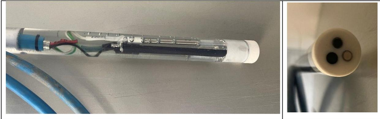
**Figure 2-20:** Side view (left) and bottom view (right) of the updated lab-scale tool fabricated in 2023. The bottom view shows the sensors' interface.
