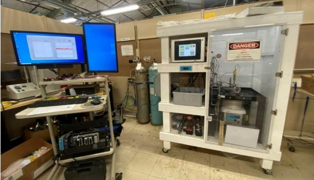
**Figure 2-10:** The full setup of the Sandia autoclave testing.
