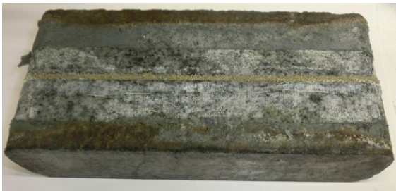
Figure 6. Sample ReB (RC proppant). Propped fracture conductivity decreases with both increasing temperature and applied stress. Data scatter is due to unstable flow behavior characteristic of proppant packs.
