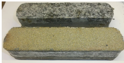
Figure 6. Sample ReB (RC proppant). Propped fracture conductivity decreases with both increasing temperature and applied stress. Data scatter is due to unstable flow behavior characteristic of proppant packs.
