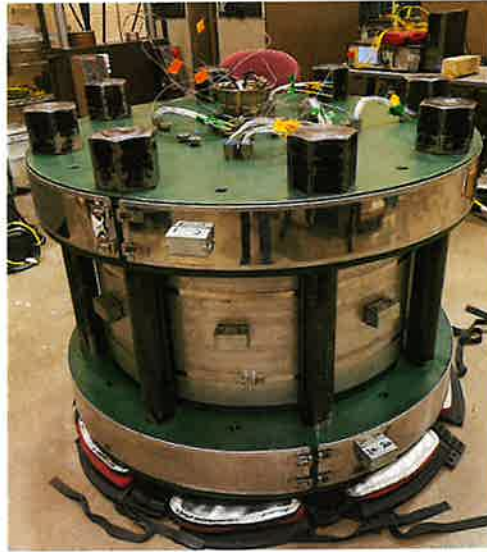
Figure 7.3. In-house high-temperature true-triaxial testing system that replicates subsurface reservoir. This system is designed to independently apply stress to a cubic rock sample along three orthogonal axes and can accommodate samples up to 432×432×432 mm (approximately 17×17×17 inches). It is capable of being employed in various experiments to investigate subsurface engineering challenges, including hydraulic fracturing, in-situ stress measurements, heat extraction, and induced seismicity.
