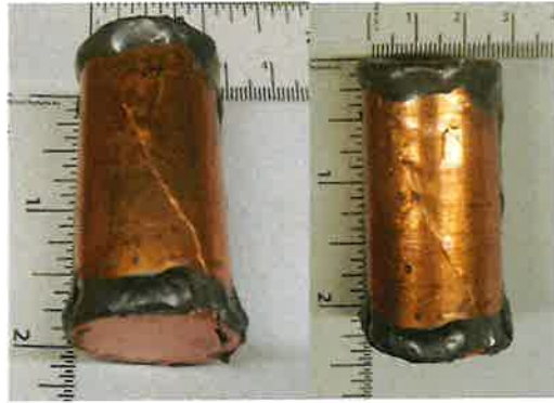
Figure 6.6. Distinct trace of a well-developed shear fracture marked on the copper jacket after rock failure.
