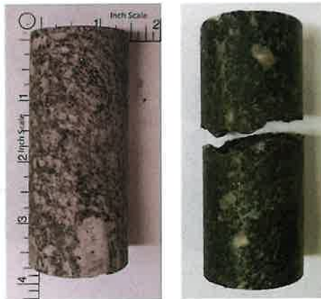
Figure 5.11. Sample E before and after splitting. The fracture is a sub-horizontal, rough tensile fracture.
