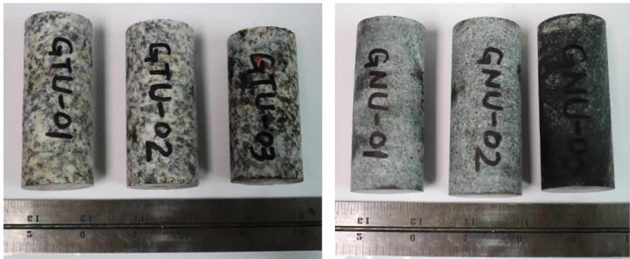
GTU samples (Granite UCS tests)
