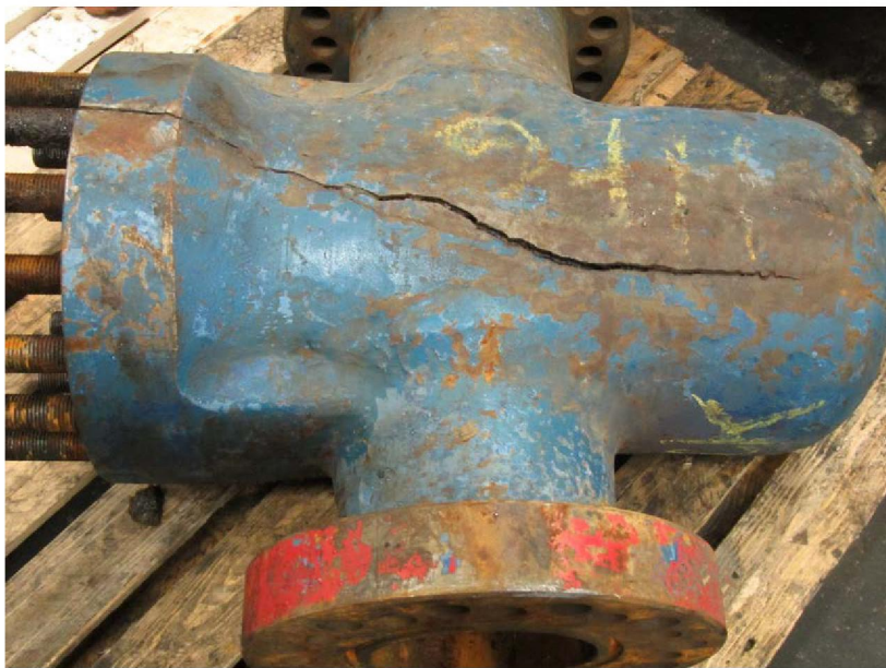
Figure 39 Cracking Corrosion of Valve Body
