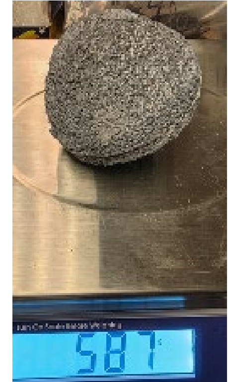
3.75" OD ball held against a 3.50" seat 10,000 psi at 450°F. Then held 6000 psi at 450°F for 48 hours until it dissolved enough to pass through the seat.
