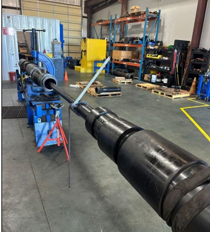
Straddle element getting loaded into the fixture for testing.
