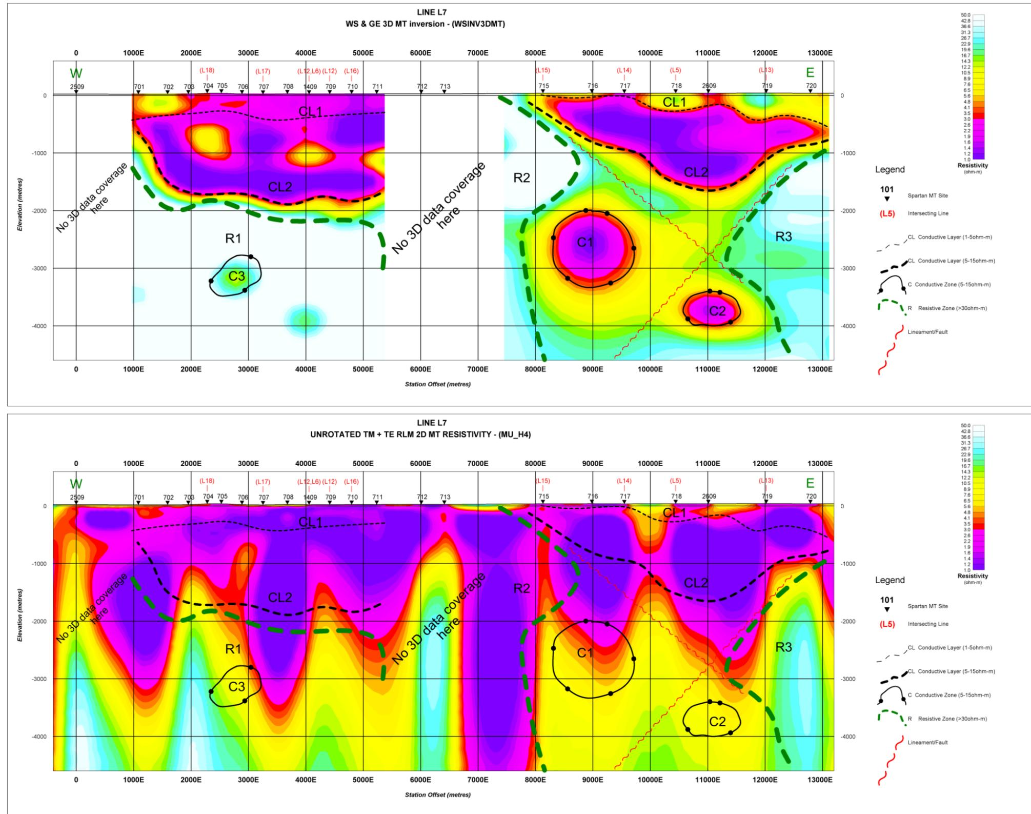
Figure 3-20: Cross-sections of the 3D inversion results (top) and the RLM 2D inversion results (bottom) along line 7.
