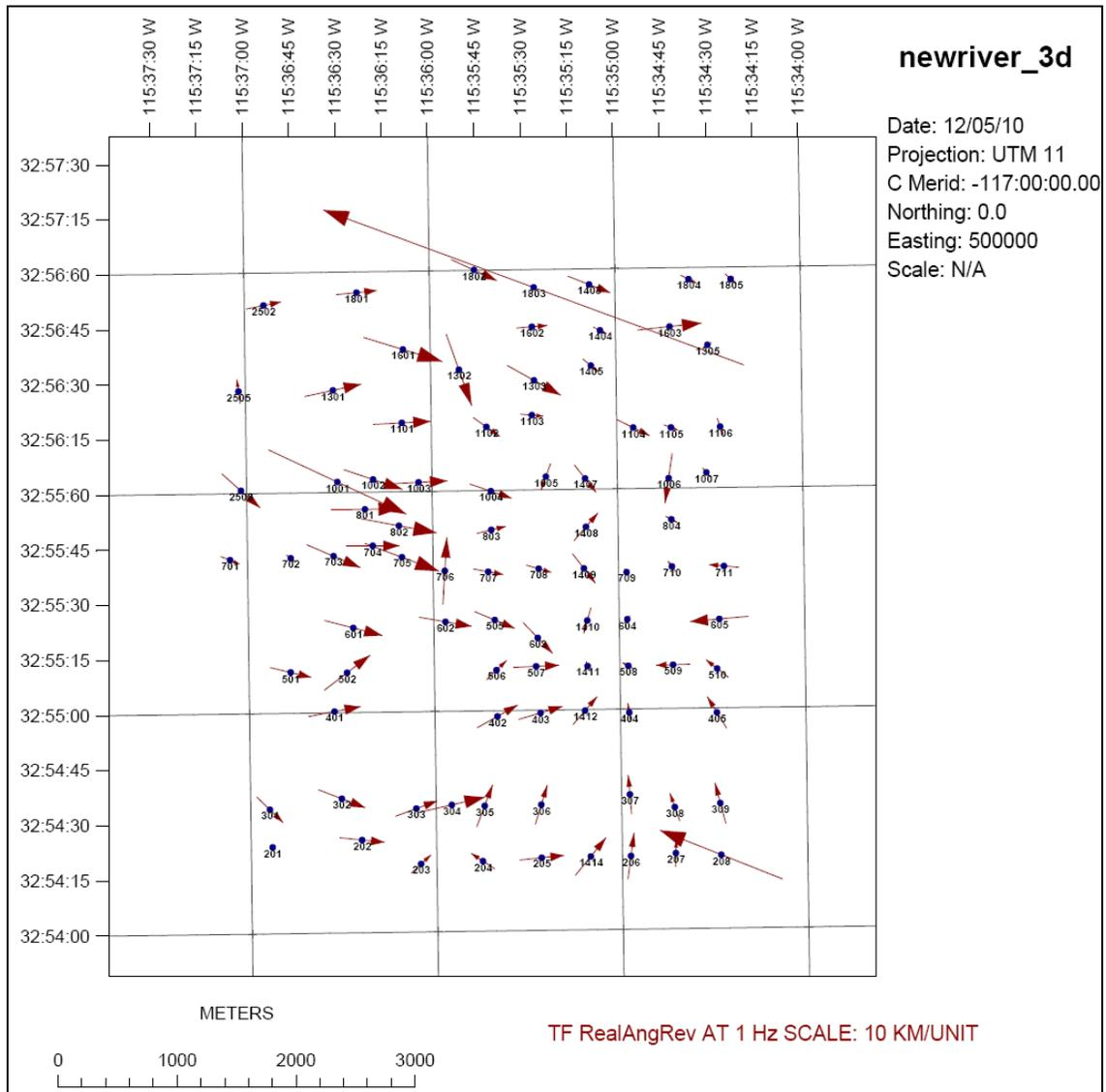
***Figure 3-4: New River grid Tipper induction vector (Re-Parkinson) at 1Hz.***
