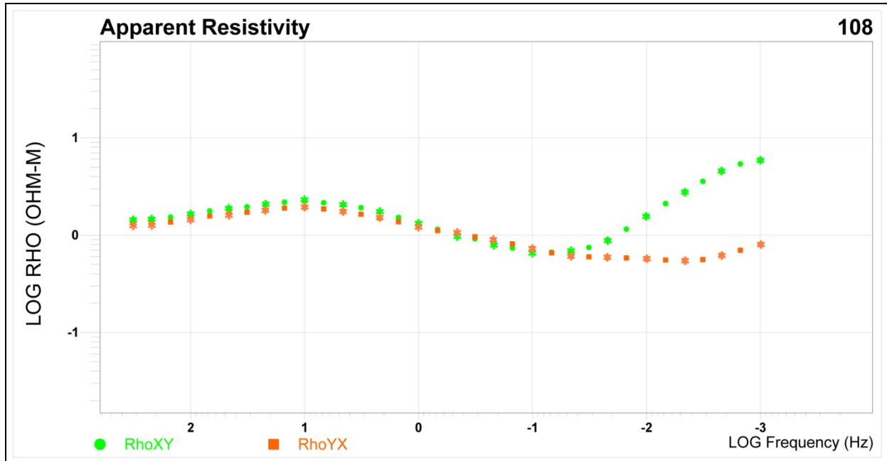
**Figure 2-1. Example of the apparent resistivity data in New River survey area. Solid Asterisk denote the selected frequencies used in the 3D inversions.**
