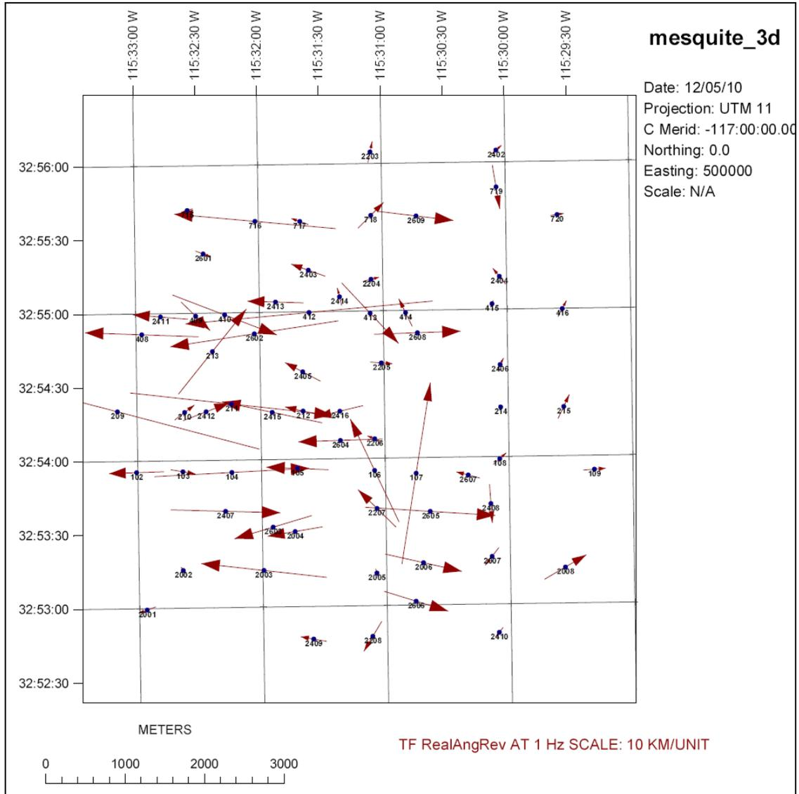
***Figure 3-2: Mesquite grid Tipper induction vector (Re-Parkinson) at 1Hz.***
