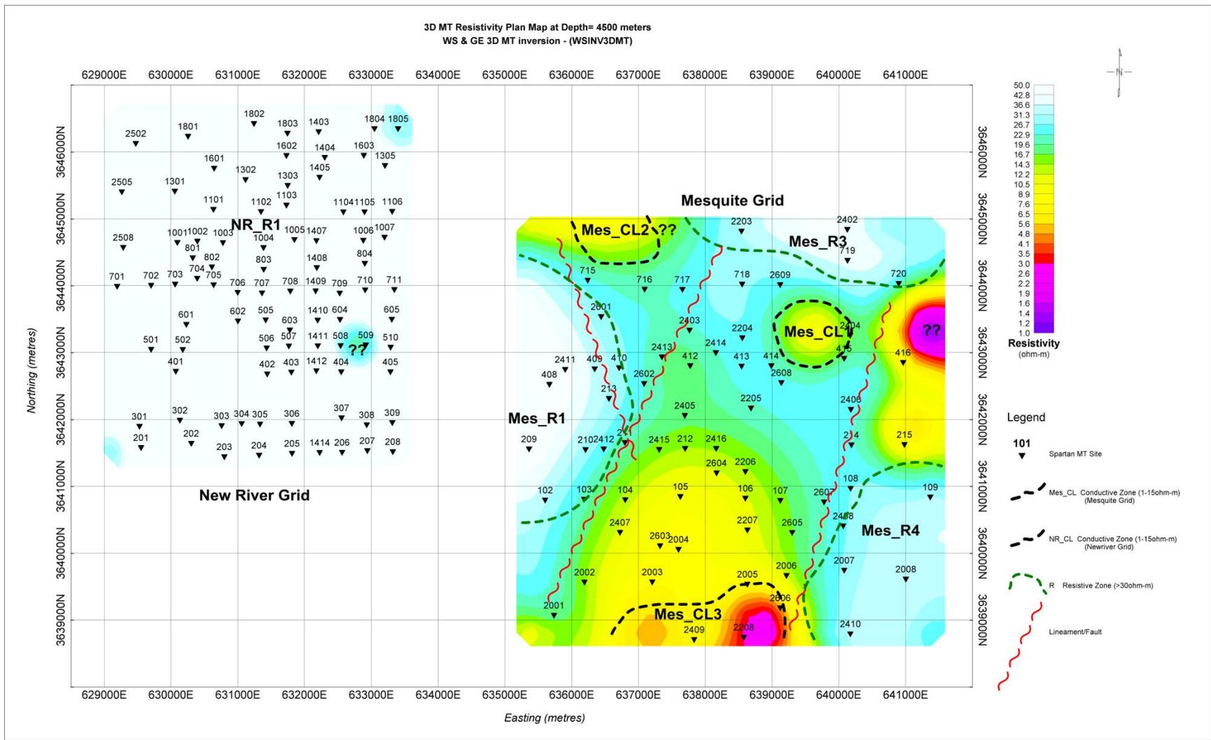
**Figure 3-15: Resistivity Plan Map of MT 3D Inversion at Depth of 4500m**
