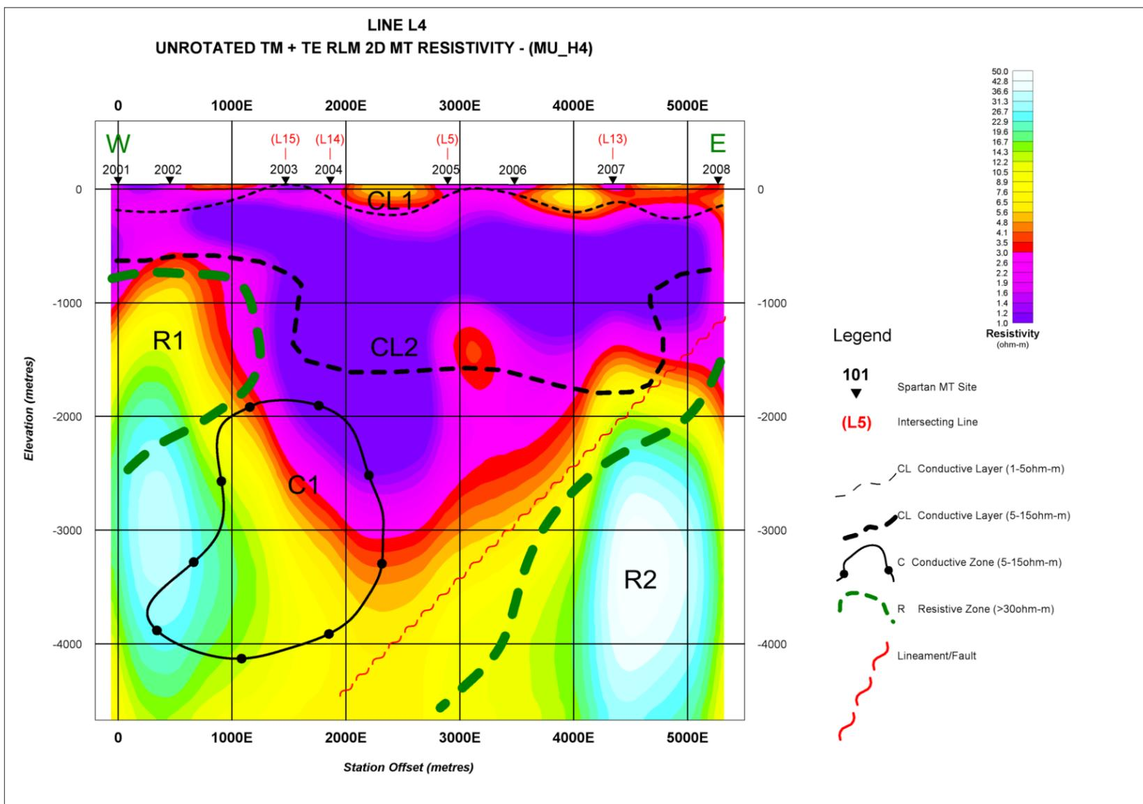
**Figure 3-19: Cross-sections of the 3D inversion results (top) and the RLM 2D inversion results (bottom) along line 4.**
