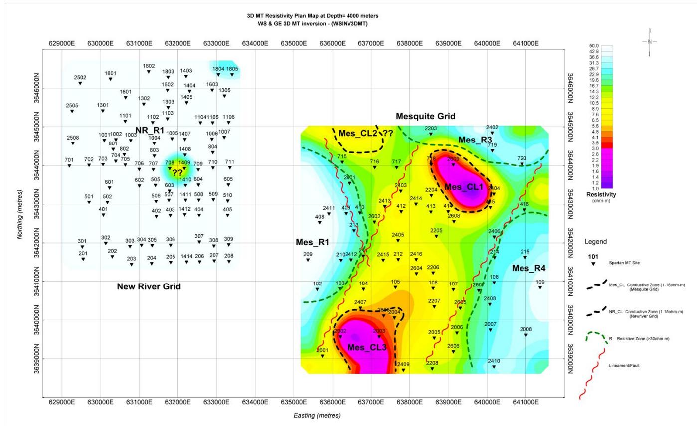
**Figure 3-14: Resistivity Plan Map of MT 3D Inversion at Depth of 4000m**
