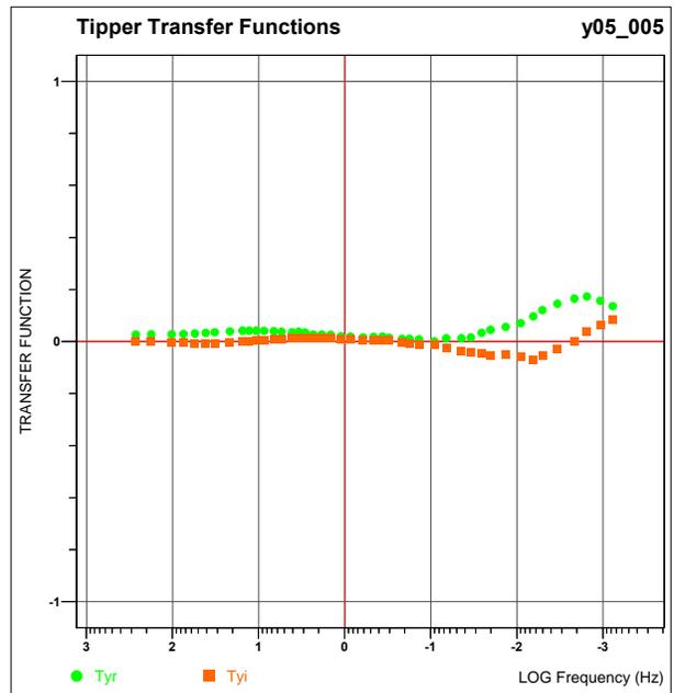
**Example of Apparent Resistivity, Phase, and Tipper Sounding Curves.**
