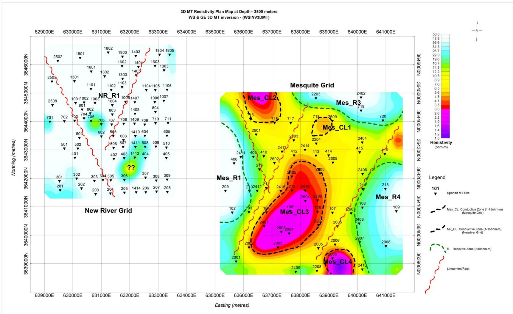
***Figure 3-13: Resistivity Plan Map of MT 3D Inversion at Depth of 3500m***
