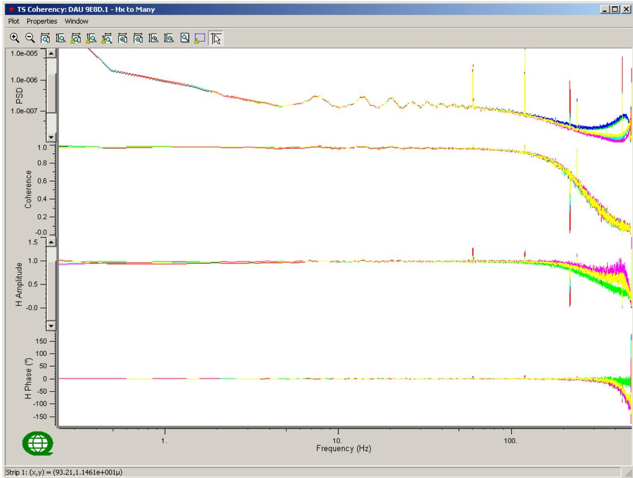
***From top to bottom: PSD of channels and Coherency and Response Function (Amplitude and Phase) compared to Reference Channel – Logarithmic frequency scale***
