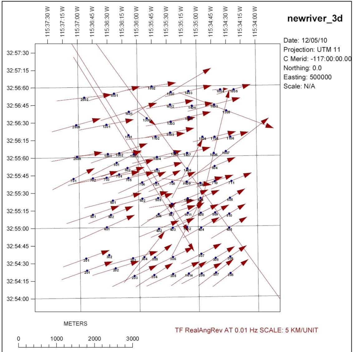
**Figure 3-5: New River grid Tipper induction vector (Re-Parkinson) at 0.01Hz.**
