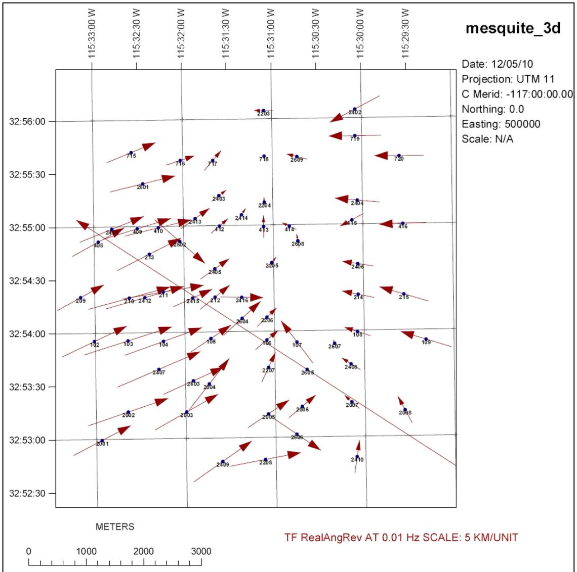
***Figure 3-3: Mesquite grid Tipper induction vector (Re-Parkinson) at 0.01Hz.***
