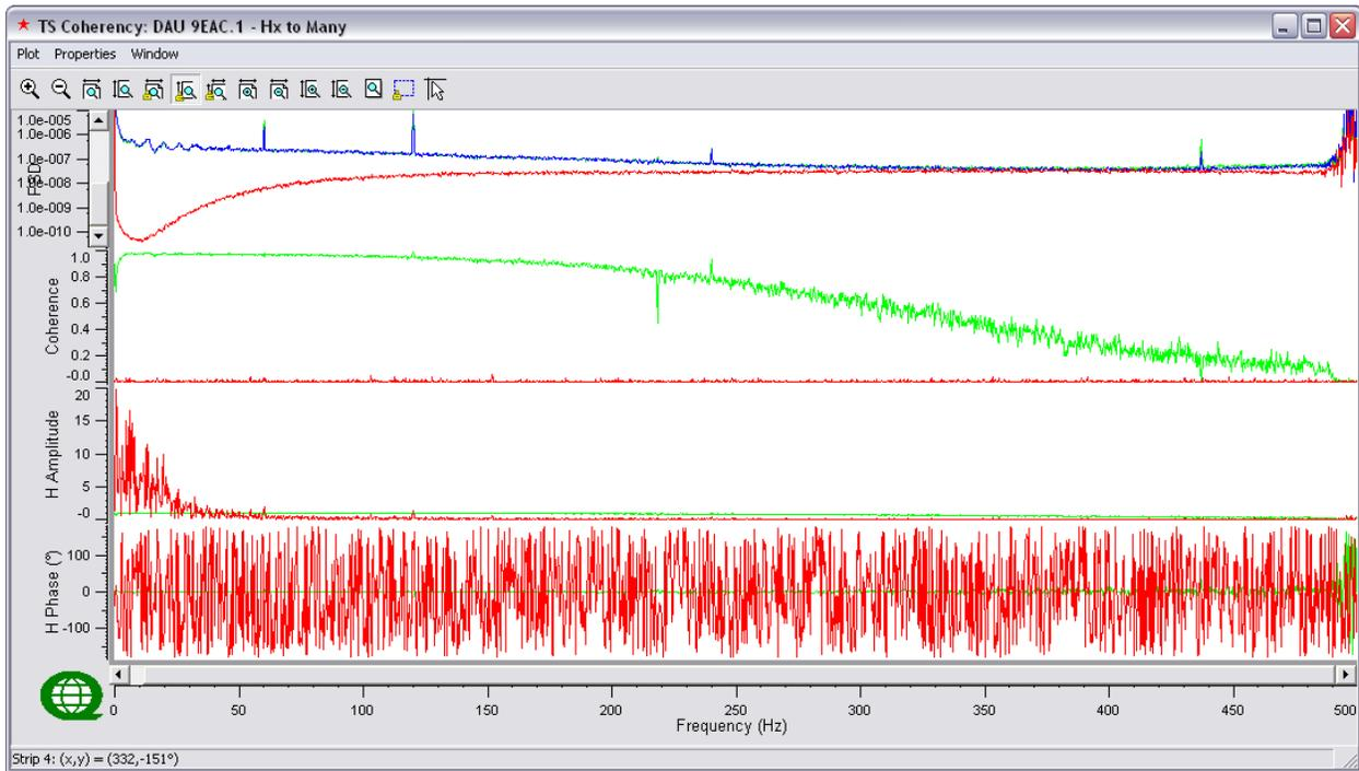
***From top to bottom: PSD of channels and Coherency and Response Function (Amplitude and Phase) compared to Reference Channel – Linear frequency scale***
