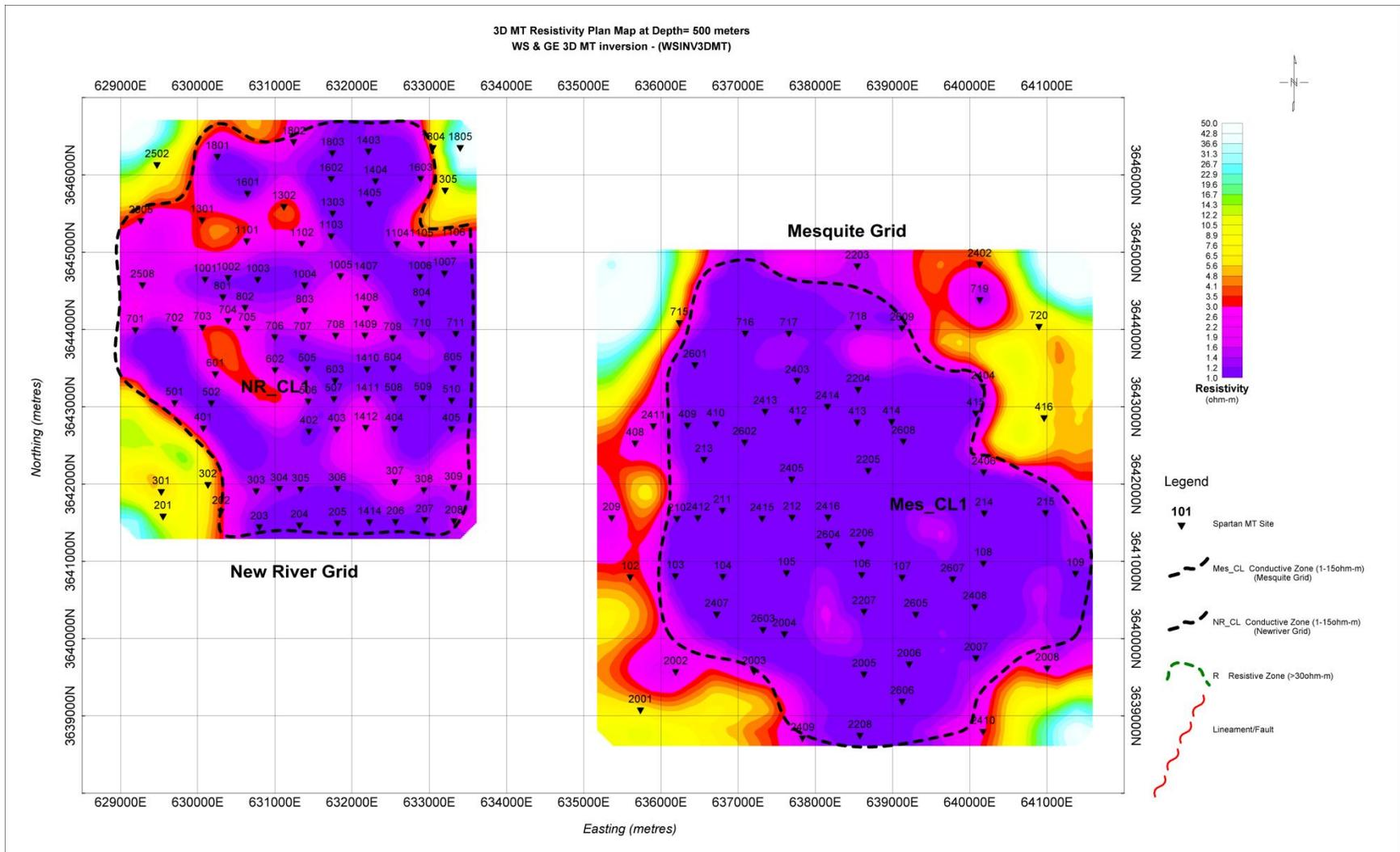
***Figure 3-7: Resistivity Plan Map of MT 3D Inversion at Depth of 500m***
