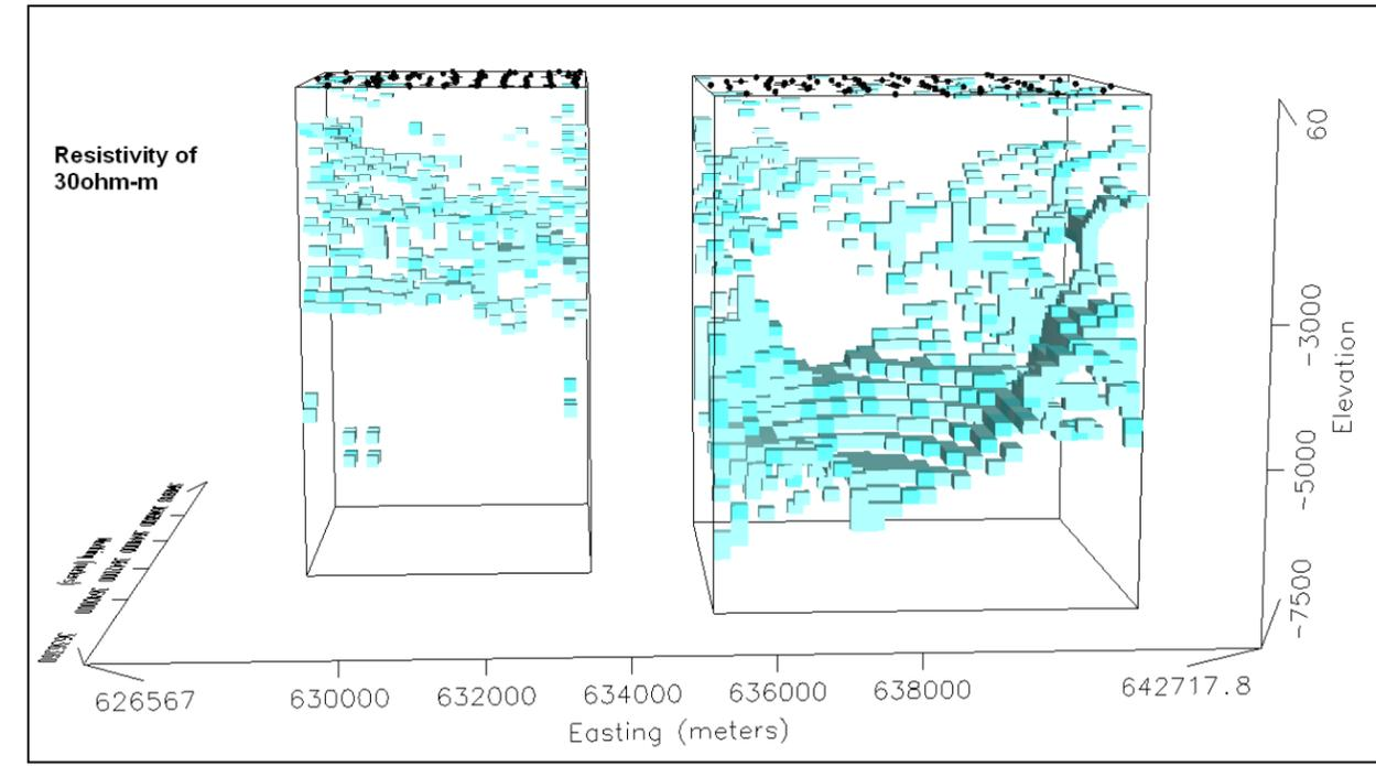
**Figure 5-1: 3D illustrations of the 3D inversion results with cut-off resistivities of less 5  $\Omega$ m (top-left), 10  $\Omega$ m (top-right), 15  $\Omega$ m (bottom-left), and 30  $\Omega$ m (bottom-right). The MT site locations are denoted as solid black circle at the surface.**
