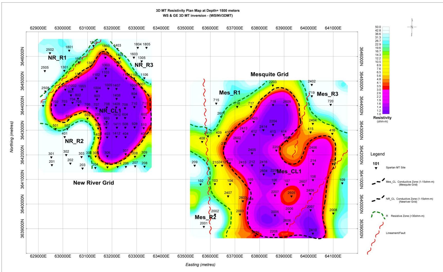
***Figure 3-9: Resistivity Plan Map of MT 3D Inversion at Depth of 1500m***
