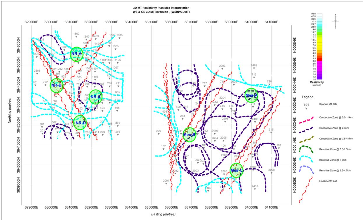
**Figure 4-4: Interpreted plan map of Mesquite and New River grids at 2-3km**
