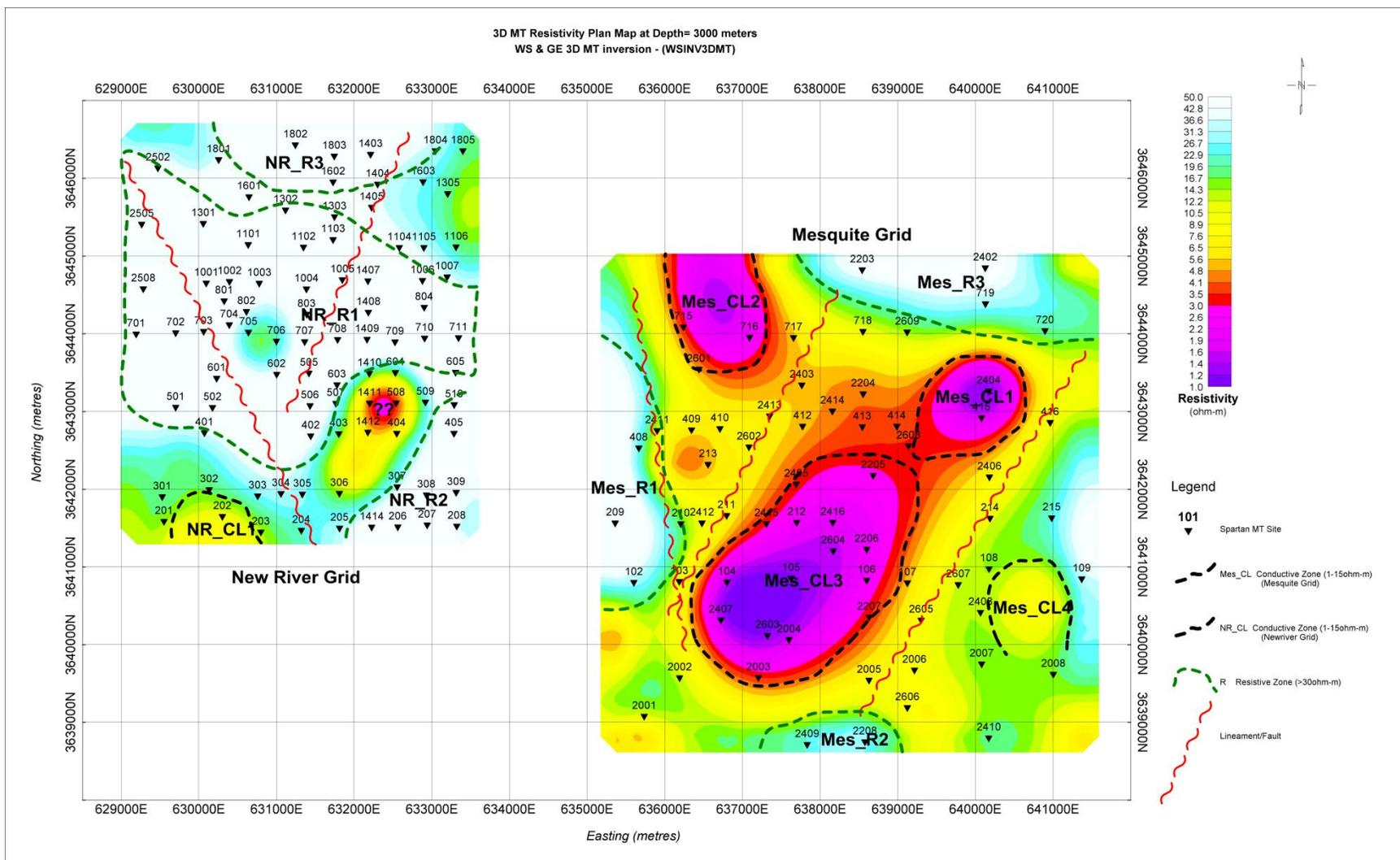
***Figure 3-12: Resistivity Plan Map of MT 3D Inversion at Depth of 3000m***
