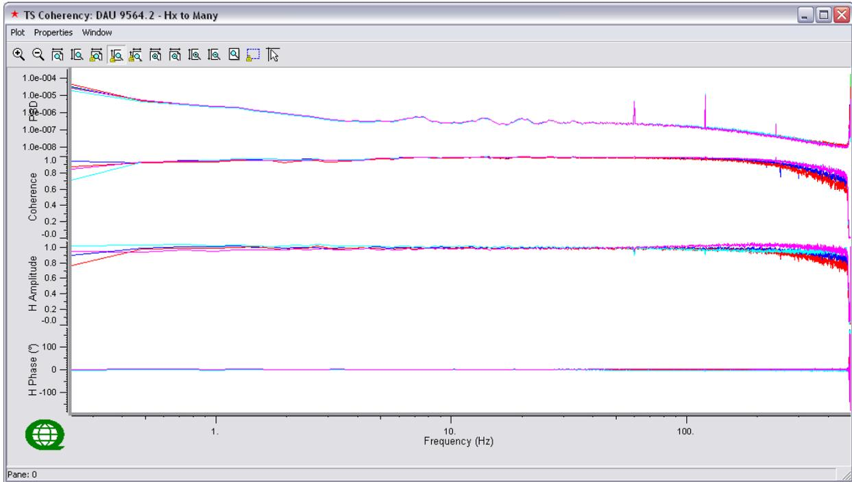
***From top to bottom: PSD of channels and Coherency and Response Function (Amplitude and Phase) compared to Reference Channel – Logarithmic frequency scale***
