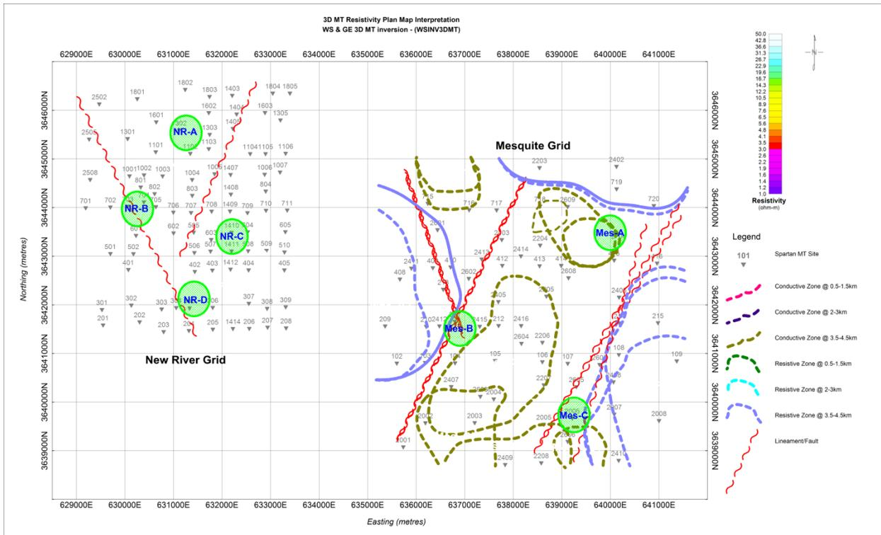
**Figure 4-5: Interpreted plan map of Mesquite and New River grids at 3.5-4.5km**
