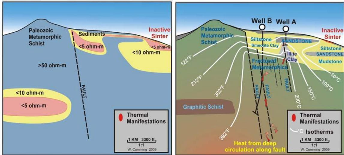
***Figure 4-2: MT cross-section and its conceptual model (from Cumming 2009).***
