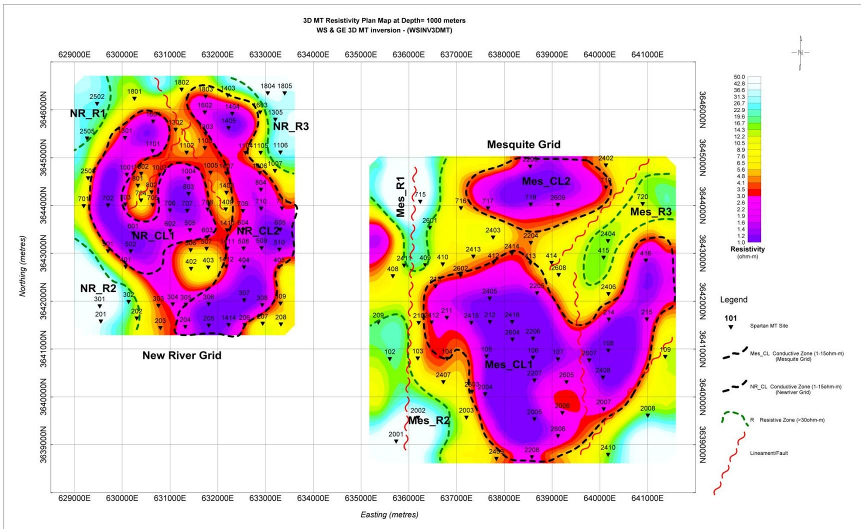
**Figure 3-8: Resistivity Plan Map of MT 3D Inversion at Depth of 1000m**
