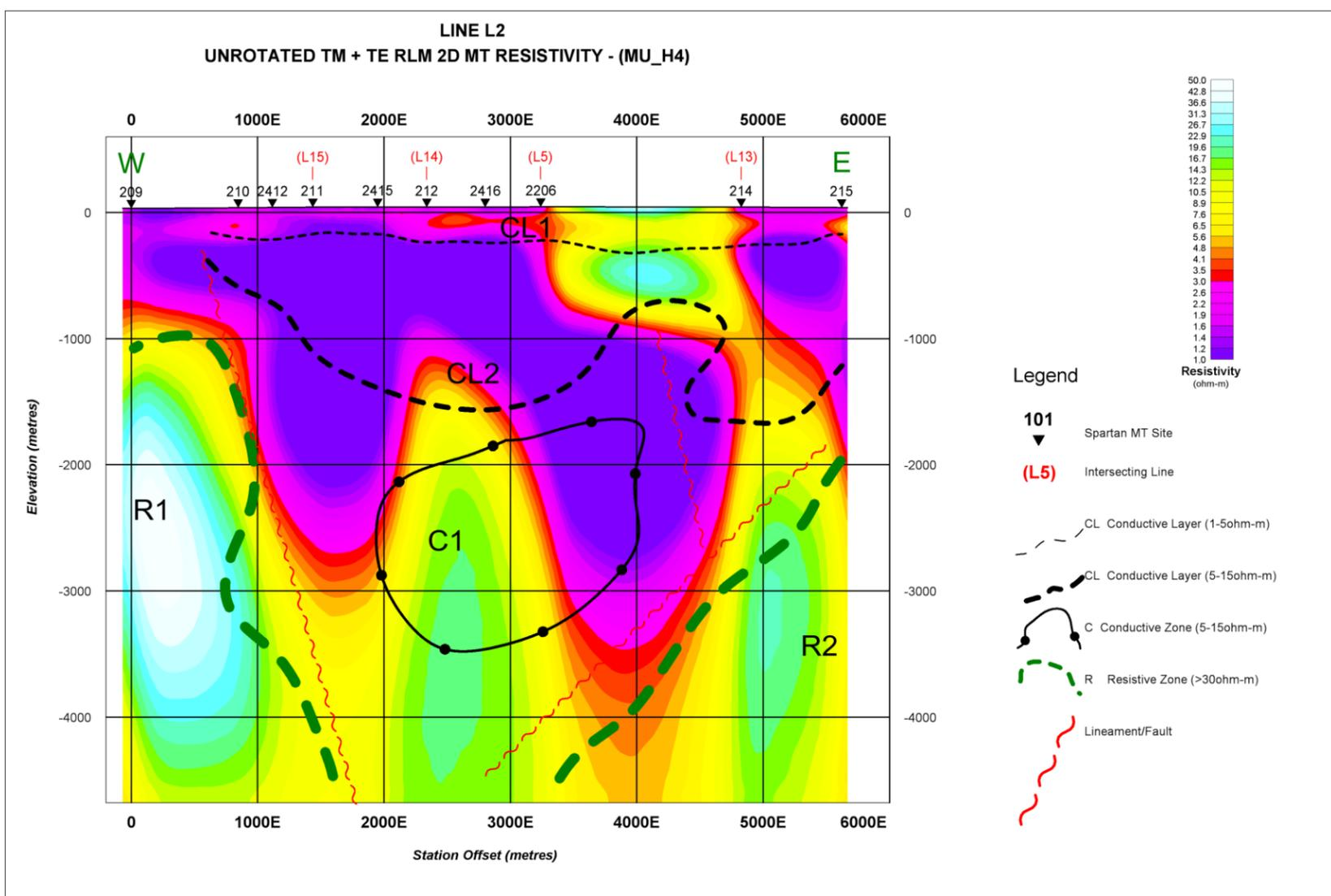
**Figure 3-17: Cross-sections of the 3D inversion results (top) and the RLM 2D inversion results (bottom) along line 2.**
