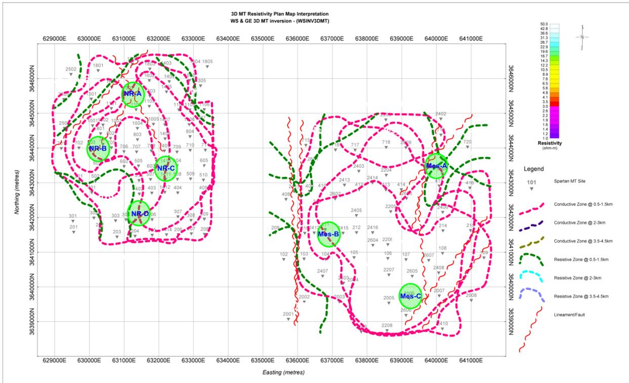
**Figure 4-3: Interpreted plan map of Mesquite and New River grids at 0.5-1.5km**
