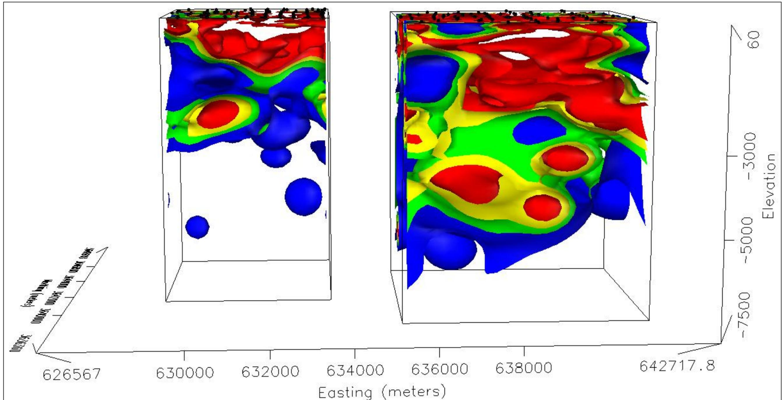
**Figure 5-2: Volumetric illustration of the Mesquite (left) and New River (right) 3D inversion results for the iso-surfaces of 5  $\Omega$ m (red), 10  $\Omega$ m (yellow), 15  $\Omega$ m (green), and 30  $\Omega$ m (blue). The MT site locations are denoted as solid black circle at the surface.**
