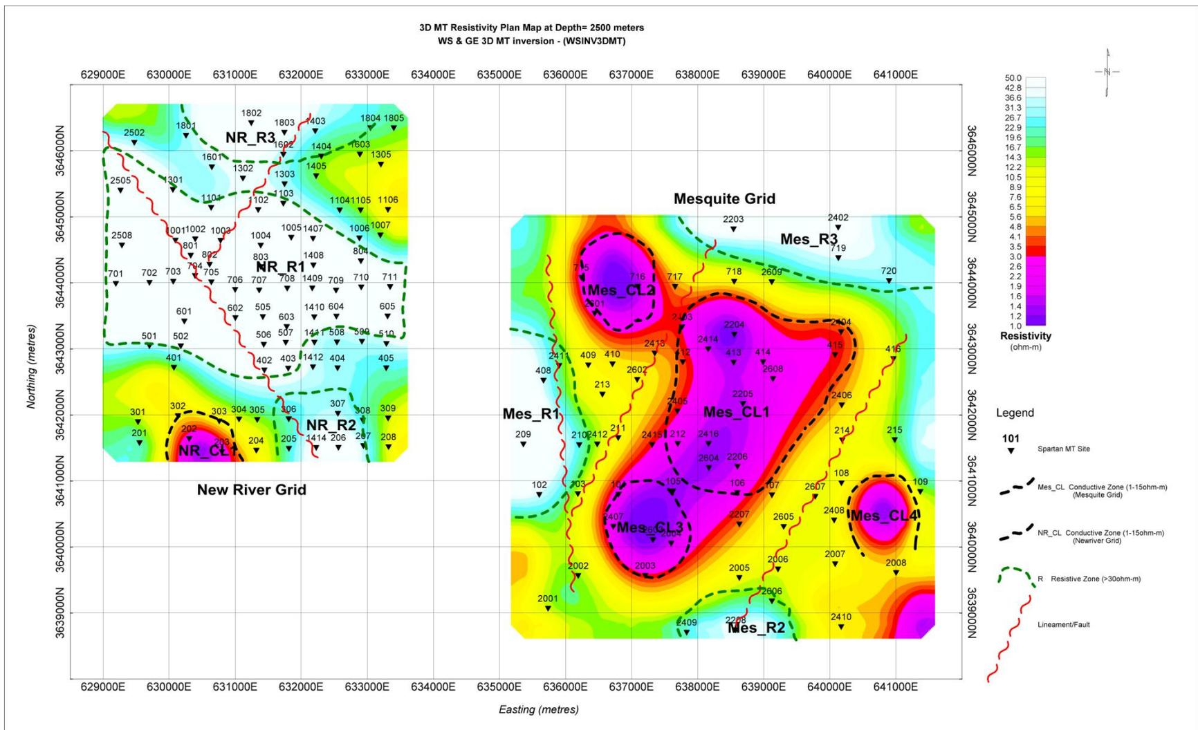
***Figure 3-11: Resistivity Plan Map of MT 3D Inversion at Depth of 2500m***
