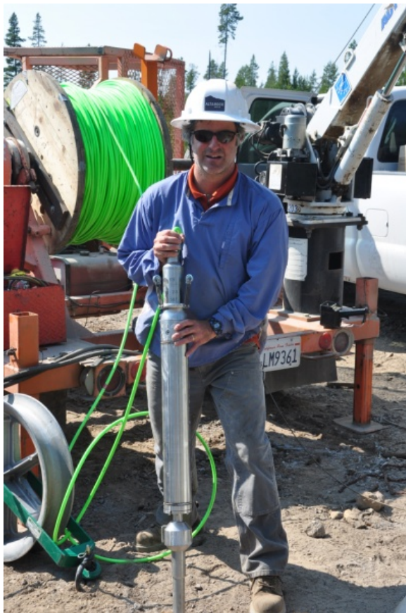
Figure 3: Borehole geophone with hole-lock adapter.
