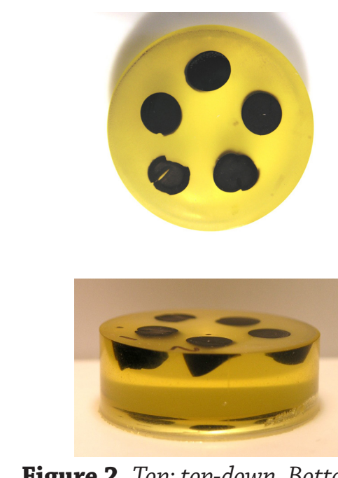
Figure 2. Top-down, Bottom: side view of cross-sectioned o-rings embedded in epoxy.
