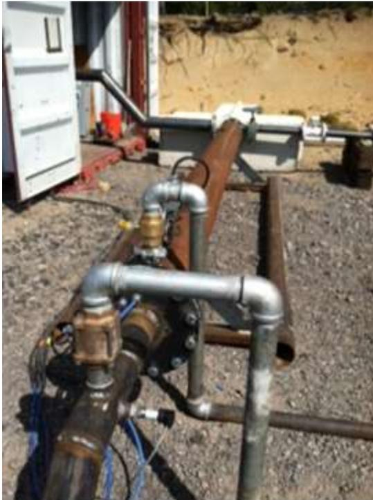
Figure 69 - Injection pump used at Pad 55-29
