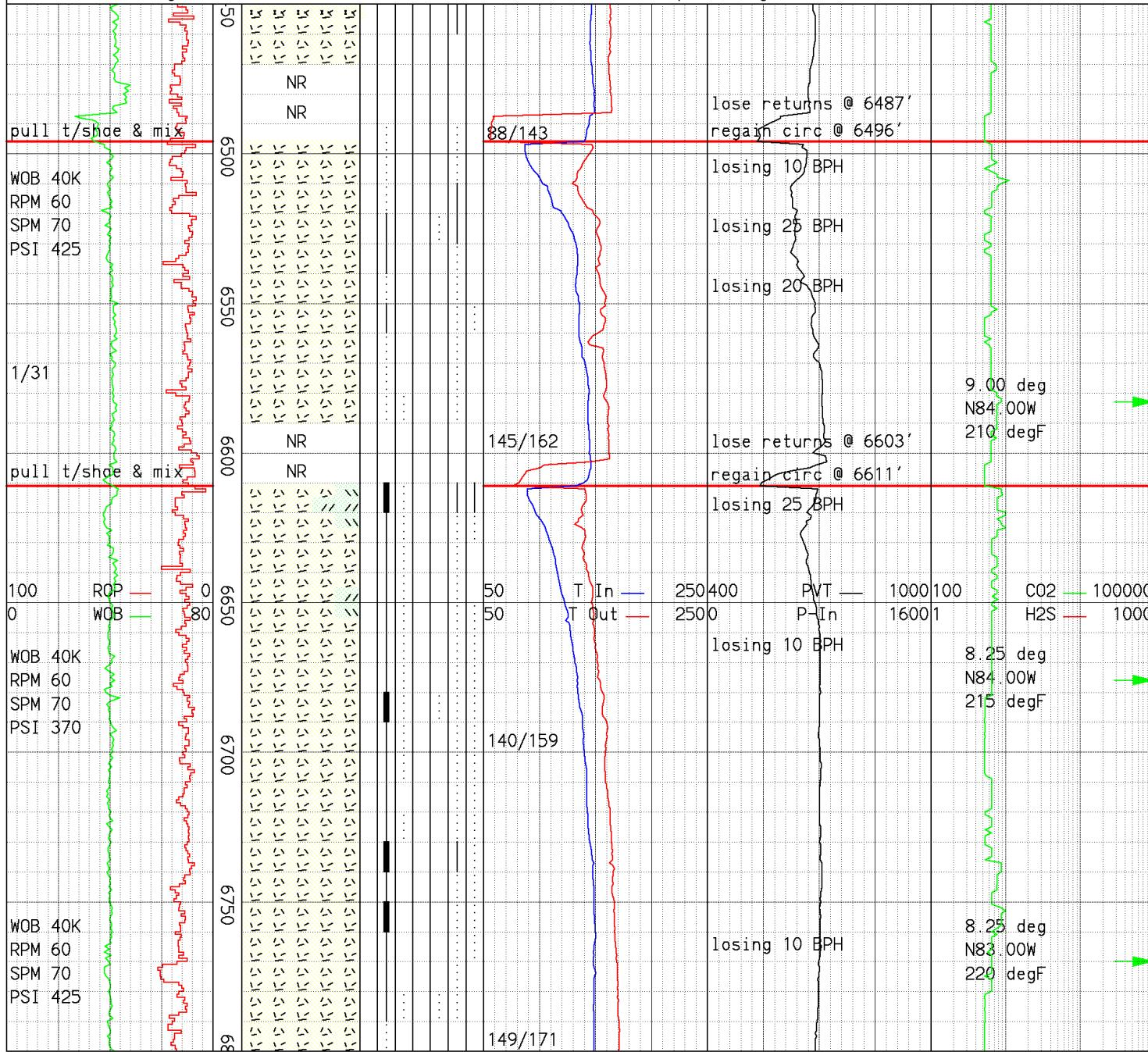
Lose returns at 6487', drill blind f/6487-96', regain circ at 6496'. Drill ahead losing 10-25 BPH.
