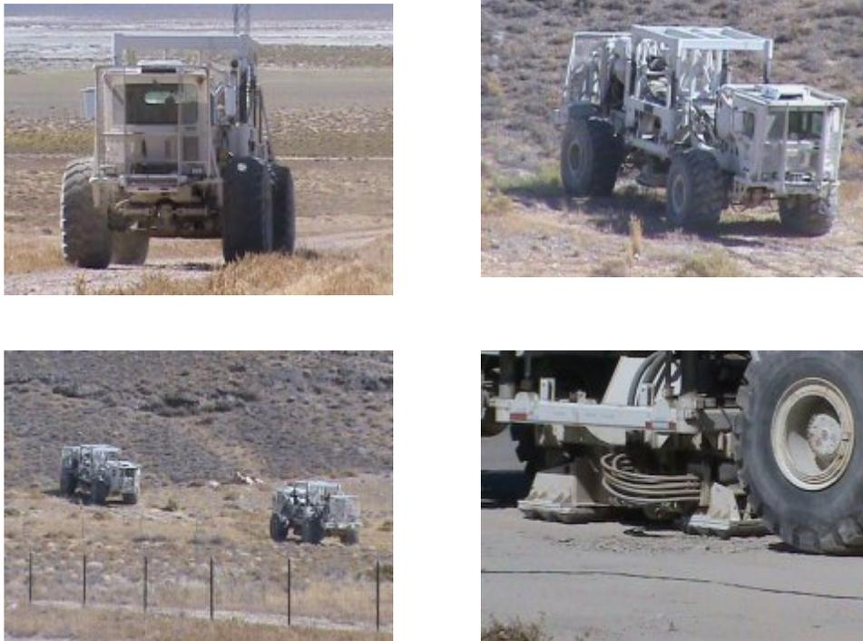
Figure 4: Shear-wave vibroseis trucks were used to shake the ground in the horizontal direction to produce shear wave energy. Shaking was done such that energy travelled along the array (inline) and also perpendicular to the array (cross line).
