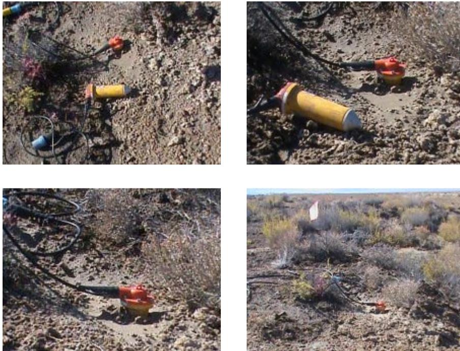
Figure 2: Three-component (3C) geophones were deployed at each geophone location at San Emidio.
