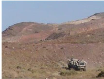
Figure 3: P-wave vibroseis trucks imparted vertical energy into the ground that was recorded by the 3C geophones.
