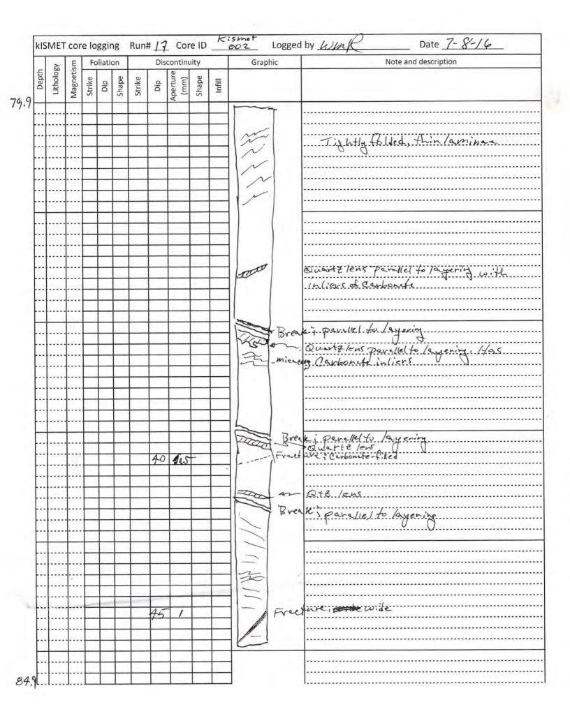
kISMET core logging Run#  $\frac{18}{002}$  Core ID  $\frac{1002}{002}$ Logged by \_\_ WMR \_\_\_\_ Date <u>7-//-/6</u> Magnetism Foliation Discontinuity Graphic Note and description Lithology Depth Aperture (mm) Strike Strike Shape Shape Infill Dip Dip 84.9 Alterneting light/derk w." more Certificate Vich / ayons predominating Drimen'h ar fenen - and/e: Drive ſω B 20 Nevy long inregular free Carboute - filled Ing (T ofen work/s 1 cm diame O · lined Q+2 Open work/Vufs C BW 89,9
