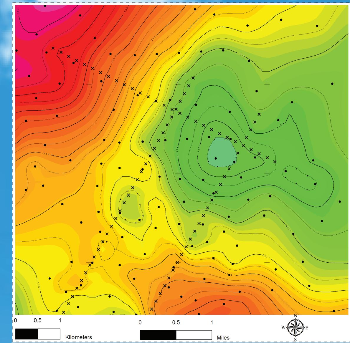
Bouger gravity calculated with a reduction density of 2.35 gm/cc over eastern dashed area shown on DEM map. Black dots and x's mark station locations. Contour interval is 0.5 mgal. Intersection of NNE-trending and ESE-trending structure may provide fluid conduit. Gravity low in northeast area would typically be interpreted as downthrown to both faults, in contrast with results from MT data.
