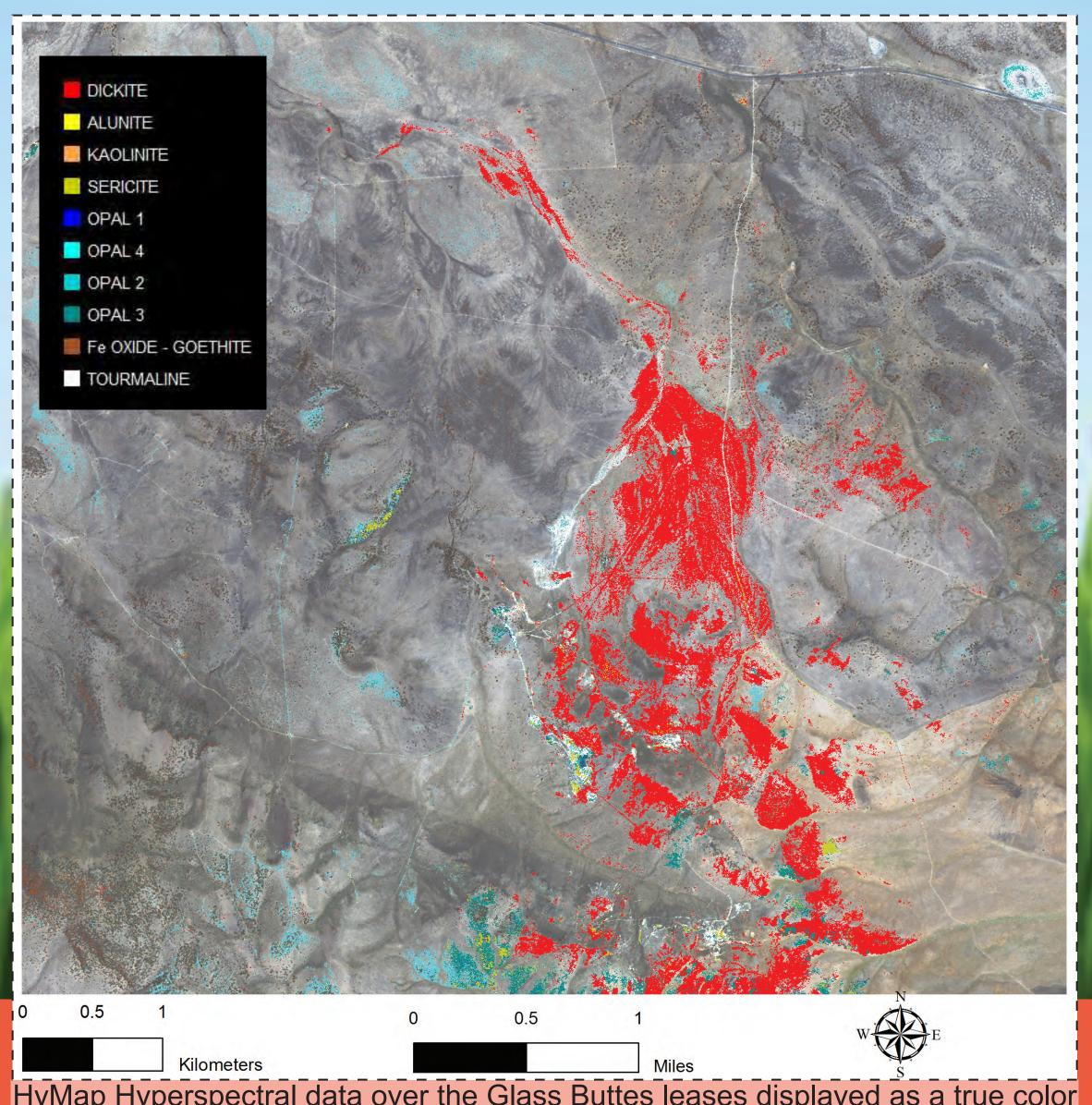
HyMap Hyperspectral data over the Glass Buttes leases displayed as a true color image. Extremely bright, disturbed areas will appear white to light blue/cyan. Overlay pixels colored according to mineralization described in inset legend. Classification from full spectral unmixing algorithms.
