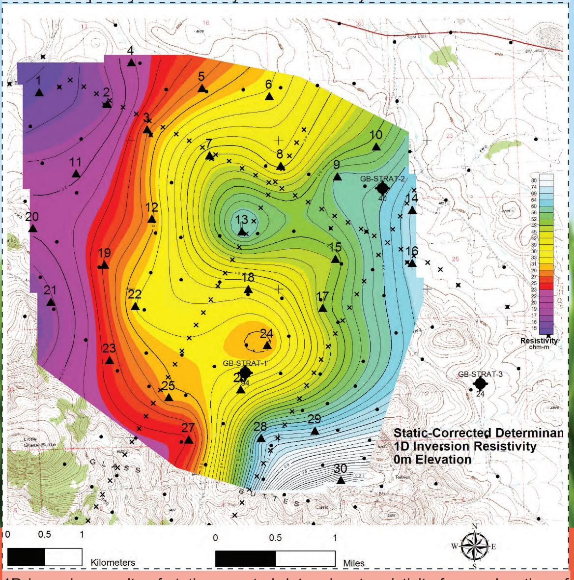
1D inversion results of static-corrected determinant resistivity for an elevation of 0 m, or approximate target depth for first slim well. North-south gradient is likely to be high angle faulting, as shown on sections to the right.
