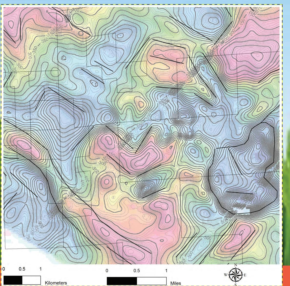
Reduced to pole aeromagnetic data with lineament interpretation.
