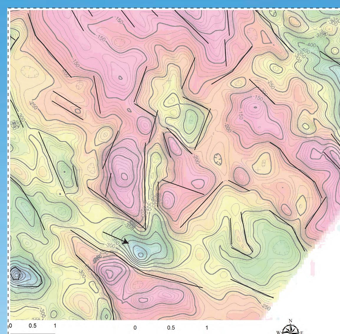
Reduced to pole aeromagnetic data with lineament interpretation. Several apparent structures correlate with faults mapped from LiDAR or on the surface (image to the right). Low magnetic susceptibility in the southeast correlates with area of hydrothermal alteration (e.g. hyperspectral image below left). The area of lowermagnetic susceptibility indicated by the arrow may indicate buried alteration.
