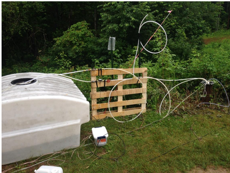
Figure 10. Picture of storage tank, flowmeters, tubing to pumps, and FSE 6.
